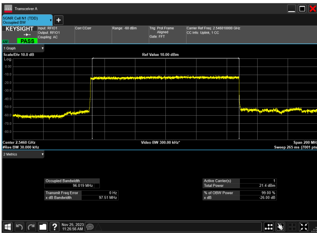
100MHz_30kHz_2546.01MHz_DFT-s-OFDM PI/2 BPSK_RB270@0 96.019 MHz
