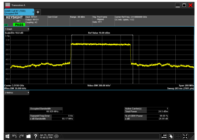
70MHz_30kHz_3515MHz_DFT-s-OFDM PI/2 BPSK_RB180@0 66.929 MHz
