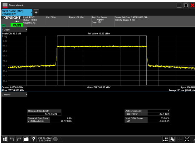
50MHz_30kHz_3475MHz_CP-OFDM 16 QAM_RB133@0 47.454 MHz
