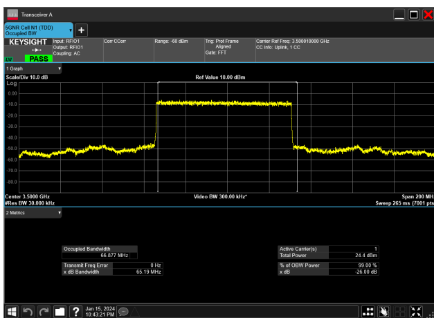
70MHz_30kHz_3500MHz_DFT-s-OFDM PI/2 BPSK_RB180@ 66.877 MHz
