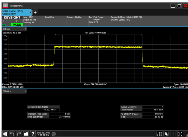
80MHz_30kHz_3740MHz_DFT-s-OFDM 256 QAM_RB216@ 77.023 MHz
