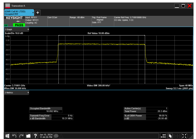
20MHz_15kHz_3710MHz_CP-OFDM 16 QAM_RB106@0 18.892 MHz
