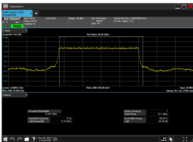
15MHz_30kHz_3840MHz_DFT-s-OFDM PI/2 BPSK_RB36@ 13.457 MHz
