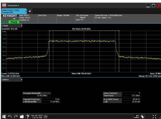
15MHz_30kHz_3707.5MHz_DFT-s-OFDM 16 QAM_RB36@0 13.453 MHz
