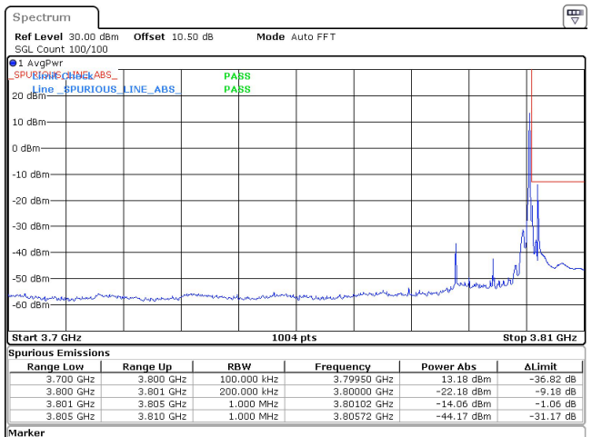
15MHz_15kHz_3792.5MHz_DFT-s-OFDM QPSK_RB1@78 -14.06 dBm
