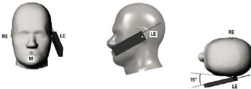
Fig.11.4 Illustration for Tilted Position
