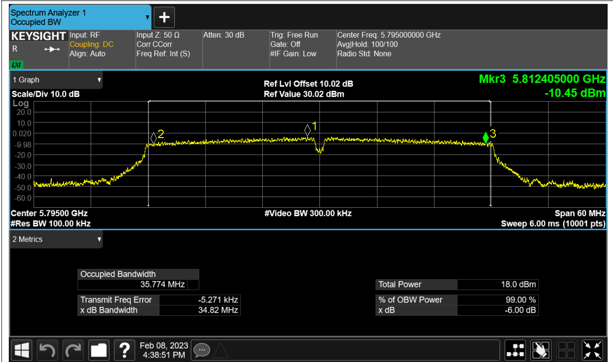
-6dB Bandwidth NVNT ac80 5775MHz Ant2
