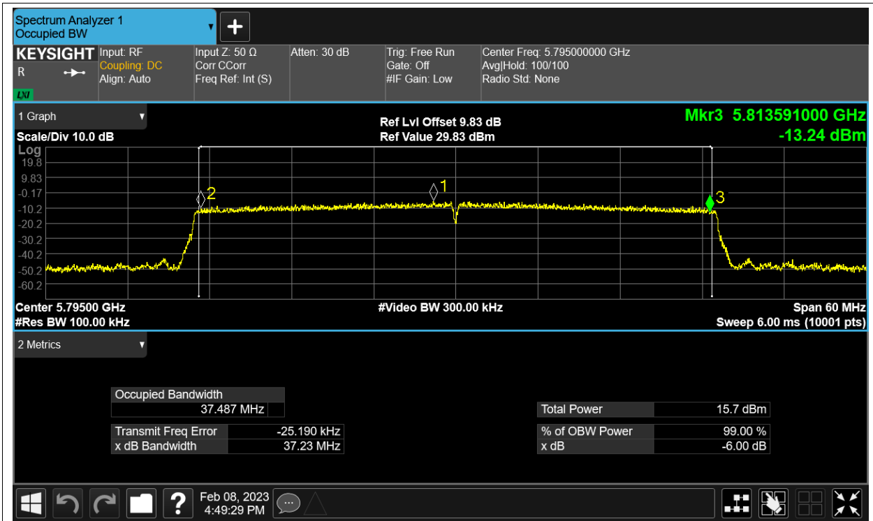
-6dB Bandwidth NVNT ax40 5795MHz Ant4
