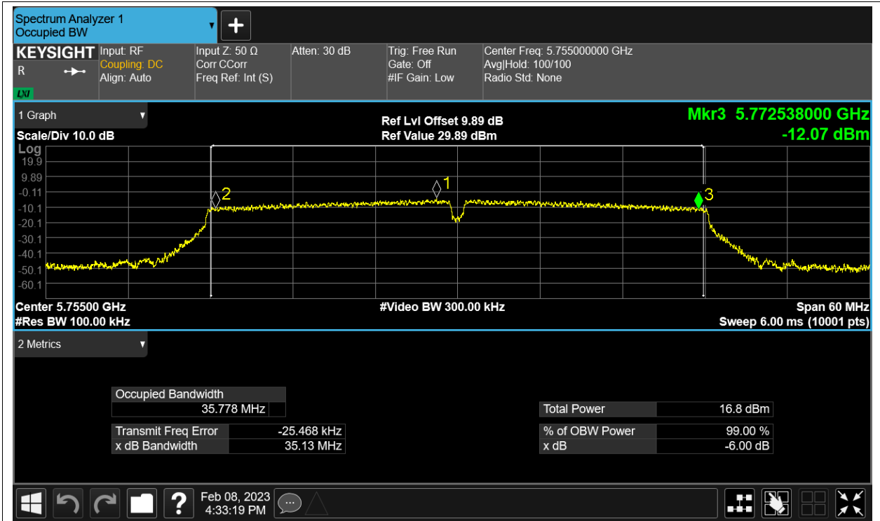
-6dB Bandwidth NVNT ac40 5755MHz Ant4
