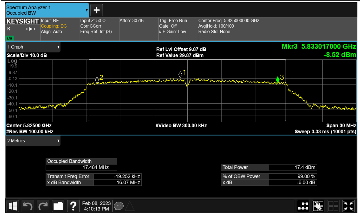
-6dB Bandwidth NVNT ac40 5755MHz Ant2
