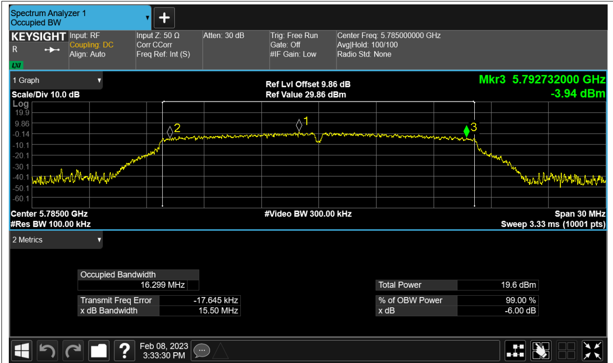
-6dB Bandwidth NVNT a 5825MHz Ant4
