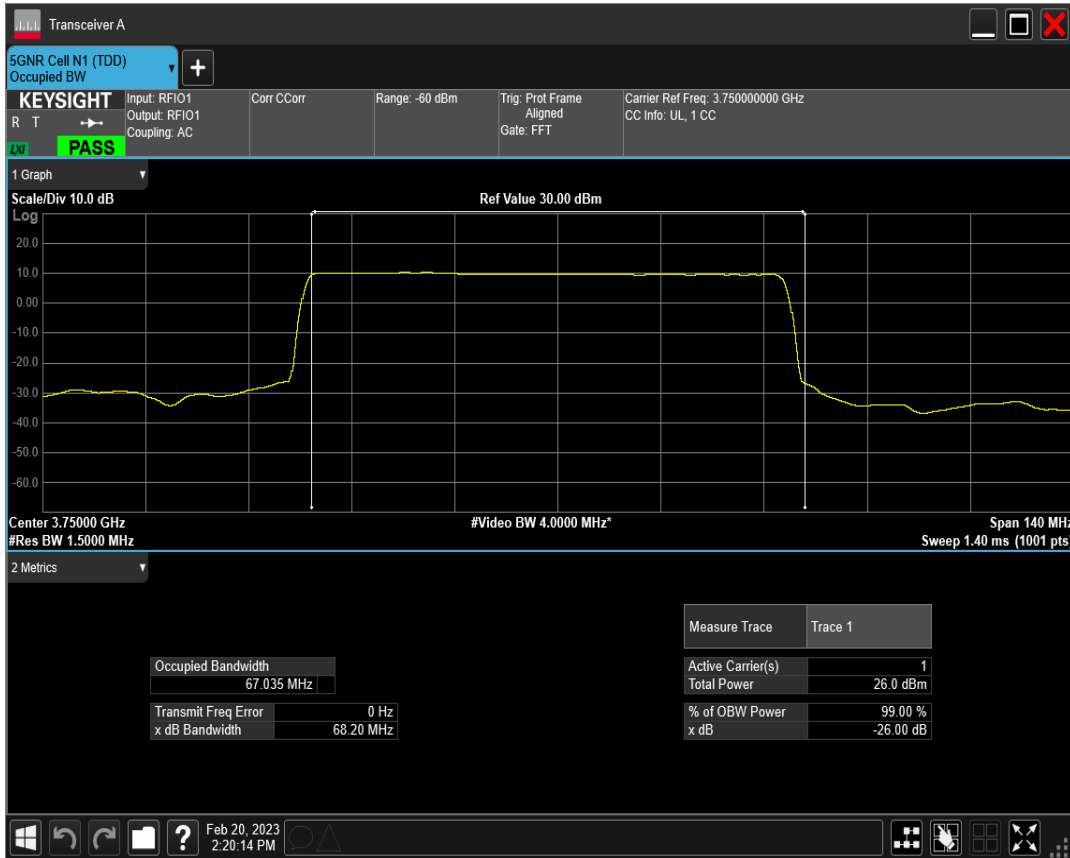
n78(3700-3800) SCS=30kHz DFT_QPSK BW=70MHz Channel=650000 RB=180@0
