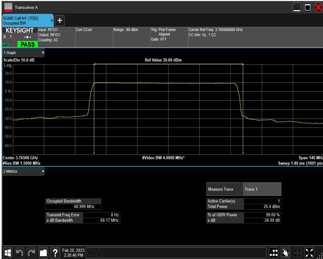
n78(3700-3800) SCS=30kHz DFT_QAM16 BW=70MHz Channel=651000 RB=180@0
