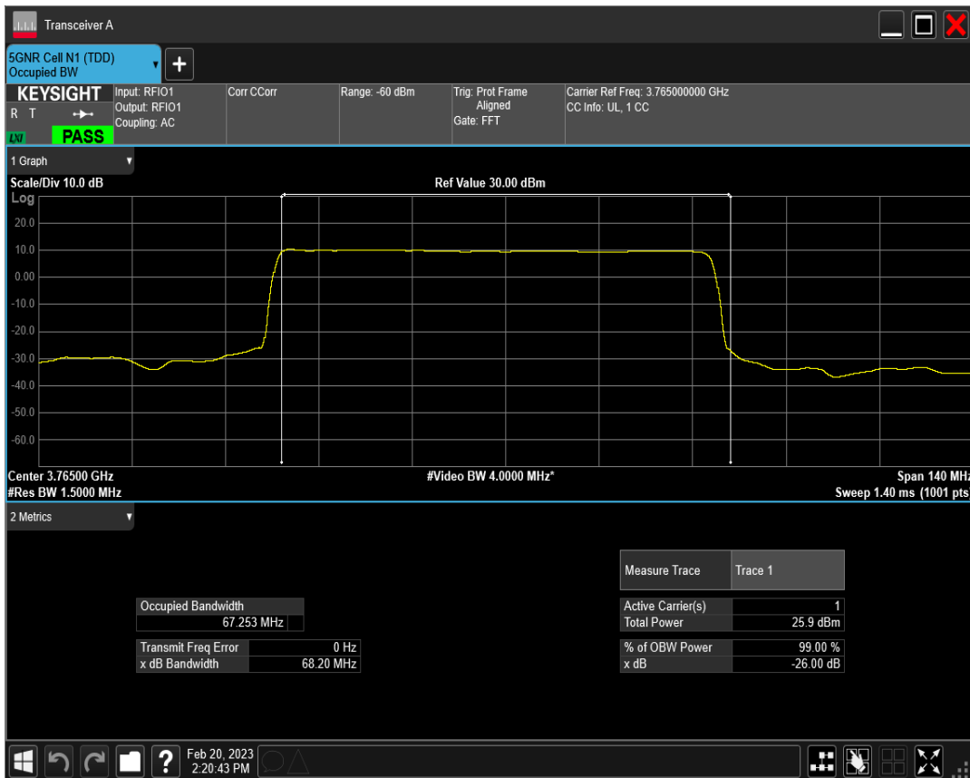
n78(3700-3800) SCS=30kHz DFT_QPSK BW=70MHz Channel=651000 RB=180@0
