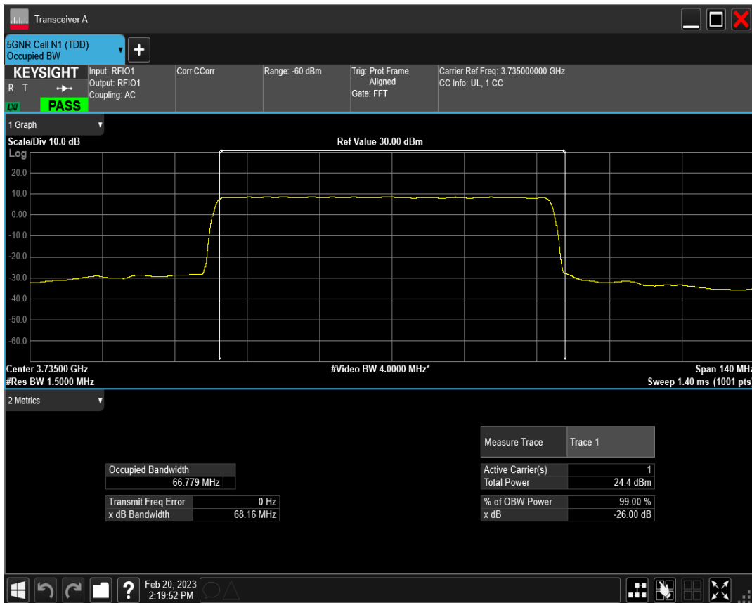
n78(3700-3800) SCS=30kHz DFT_QAM64 BW=70MHz Channel=649000 RB=180@0
