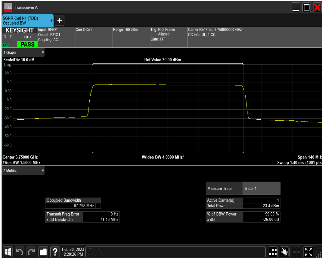
n78(3700-3800) SCS=30kHz DFT_BPSK BW=70MHz Channel=651000 RB=180@0
