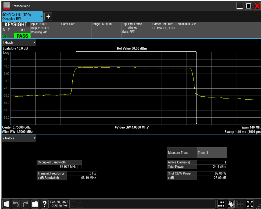
n78(3700-3800) SCS=30kHz DFT_QAM64 BW=70MHz Channel=650000 RB=180@0
