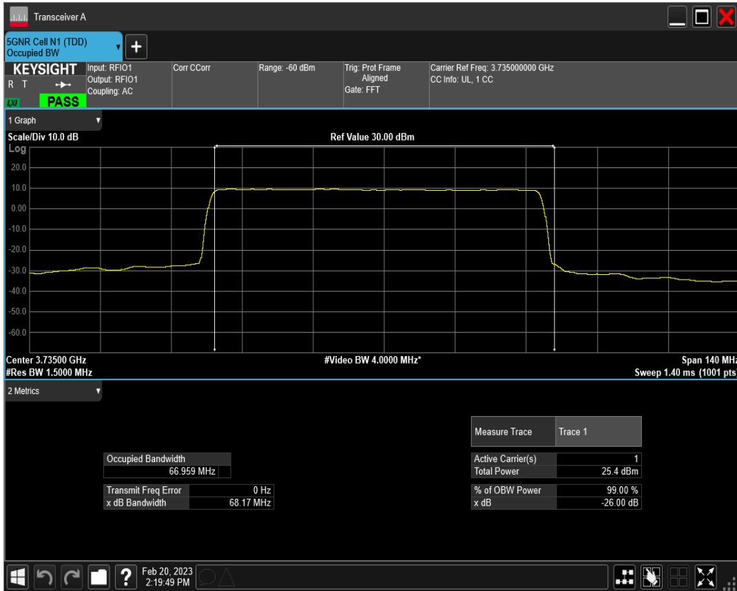
n78(3700-3800) SCS=30kHz DFT_QAM16 BW=70MHz Channel=649000 RB=180@0
