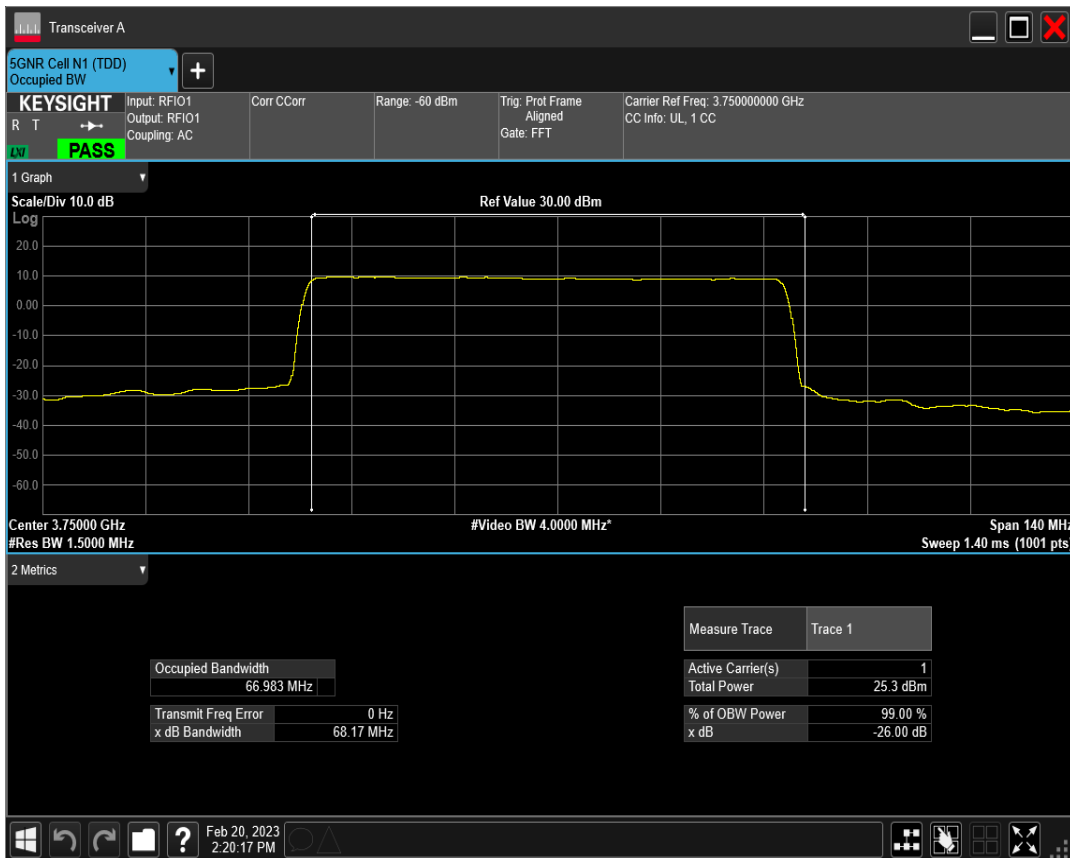
n78(3700-3800) SCS=30kHz DFT_QAM16 BW=70MHz Channel=650000 RB=180@0
