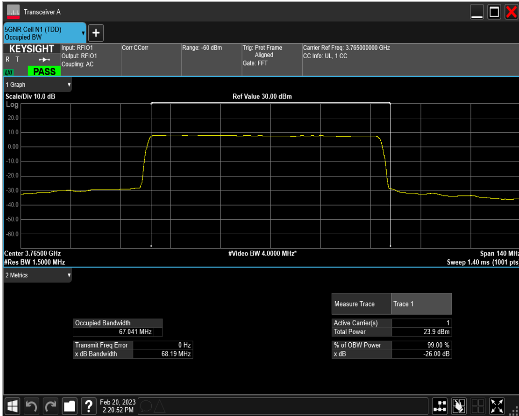
n78(3700-3800) SCS=30kHz CP_QPSK BW=70MHz Channel=651000 RB=189@0
