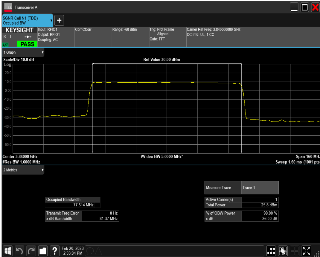
n77(3700-3980) SCS=30kHz DFT_QPSK BW=80MHz Channel=656000 RB=216@0
