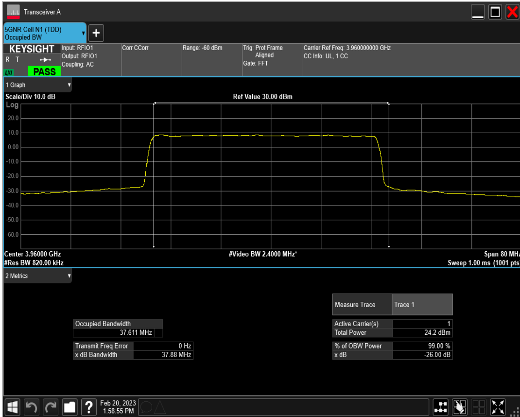
n77(3700-3980) SCS=30kHz DFT_QAM64 BW=40MHz Channel=664000 RB=100@0
