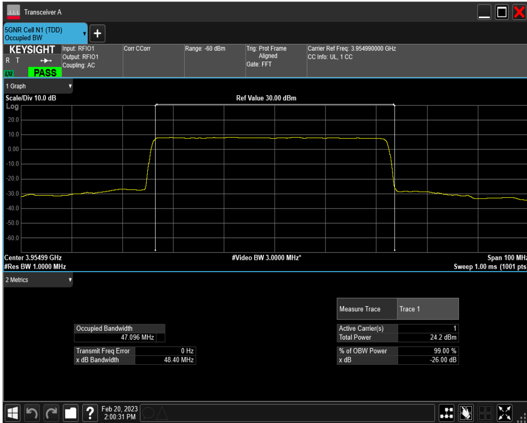
n77(3700-3980) SCS=30kHz DFT_QAM64 BW=50MHz Channel=663666 RB=128@0
