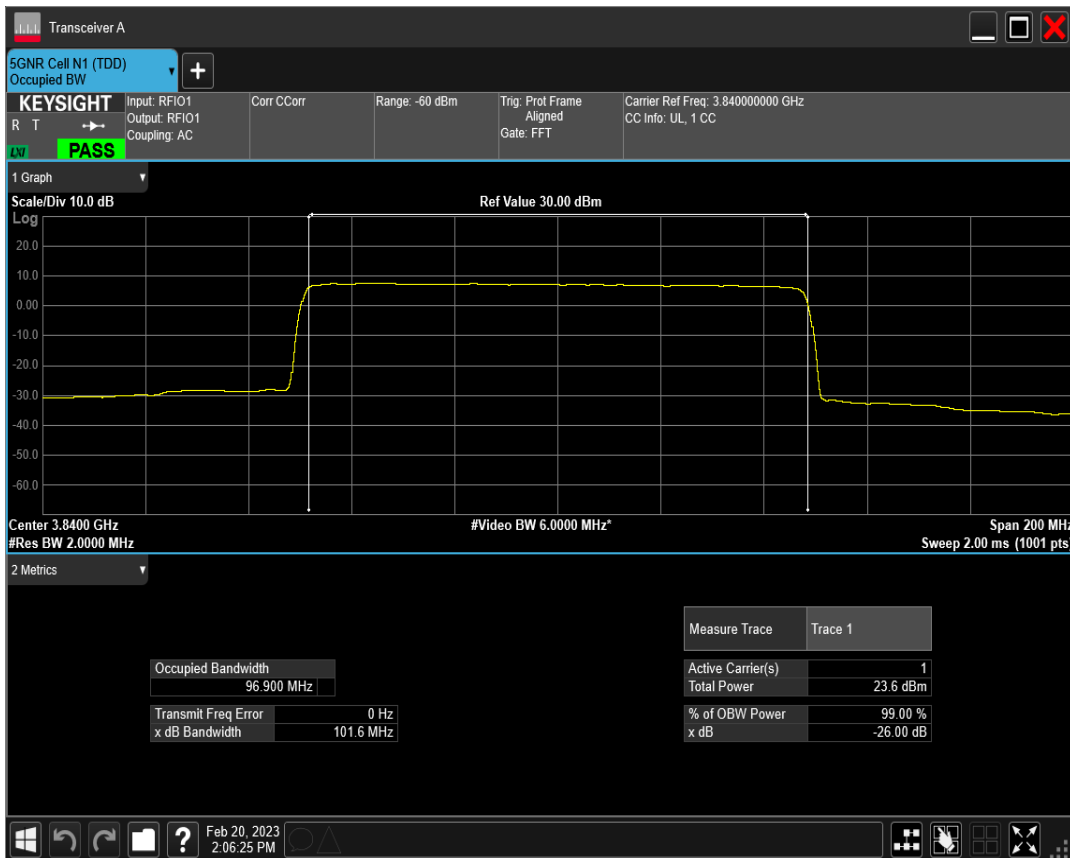
n77(3700-3980) SCS=30kHz DFT_QAM256 BW=100MHz Channel=656000 RB=270@0
