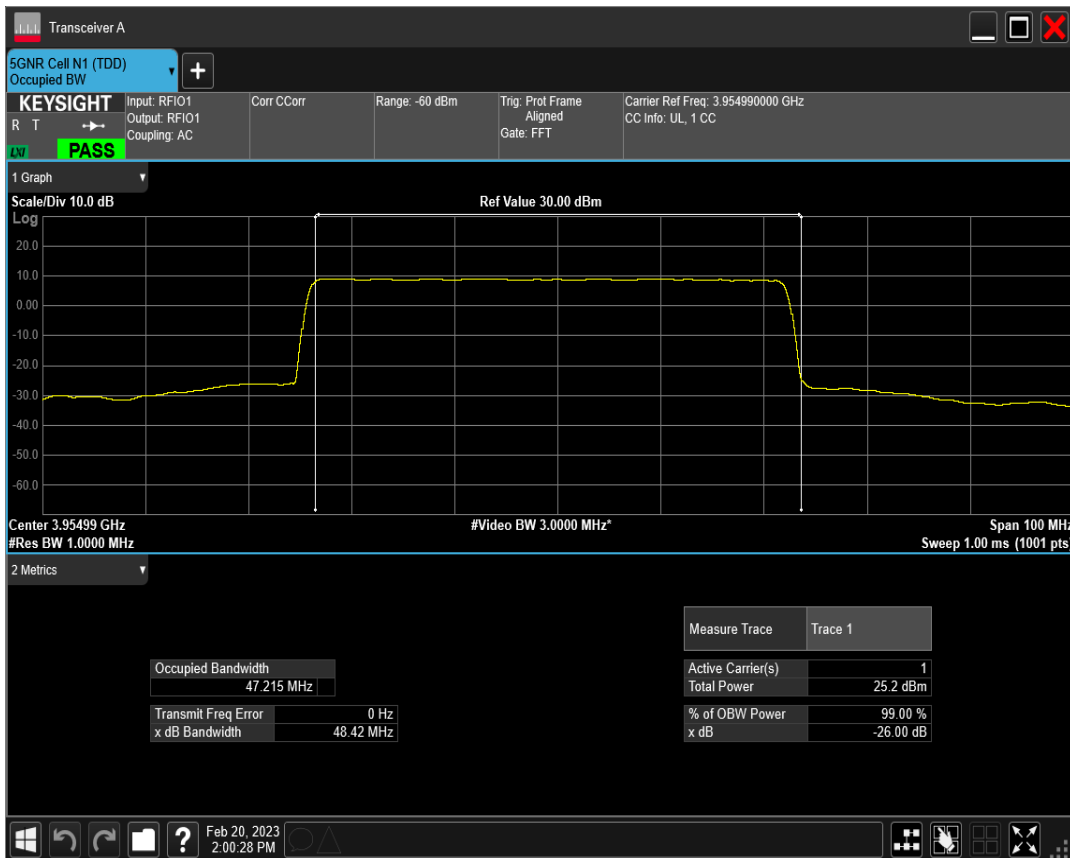
n77(3700-3980) SCS=30kHz DFT_QAM16 BW=50MHz Channel=663666 RB=128@0
