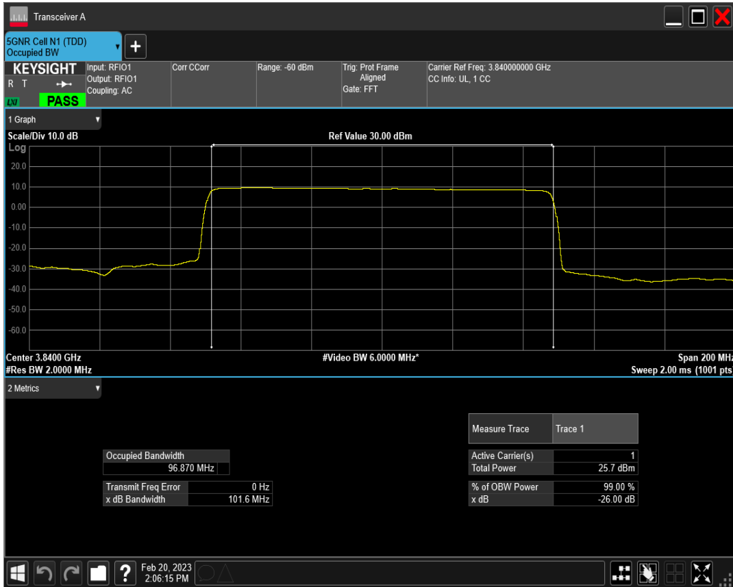
n77(3700-3980) SCS=30kHz DFT_QPSK BW=100MHz Channel=656000 RB=270@0
