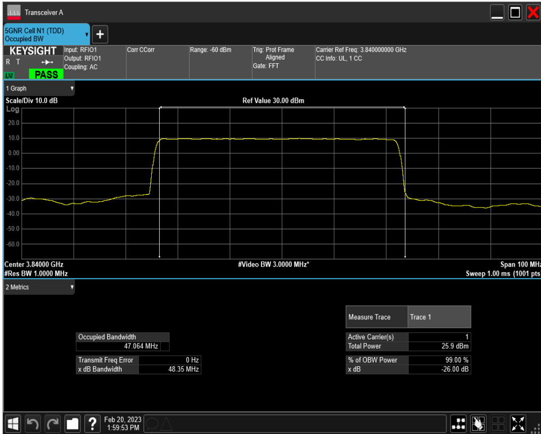
n77(3700-3980) SCS=30kHz DFT_QPSK BW=50MHz Channel=656000 RB=128@0
