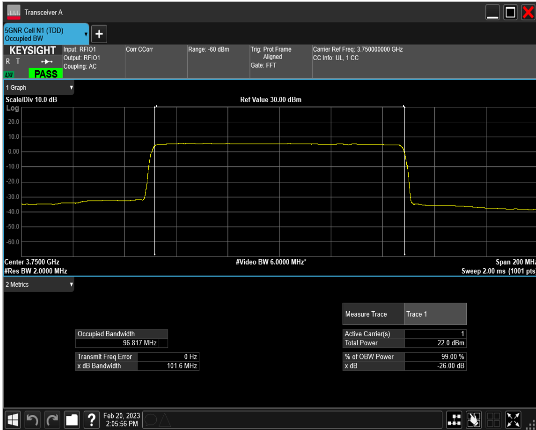
n77(3700-3980) SCS=30kHz CP_QPSK BW=100MHz Channel=650000 RB=273@0
