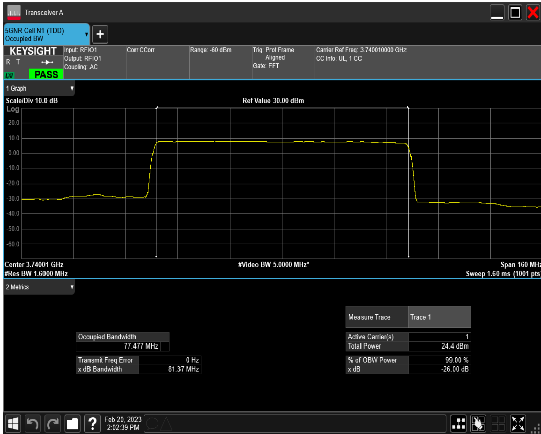
n77(3700-3980) SCS=30kHz DFT_QAM64 BW=80MHz Channel=649334 RB=216@0
