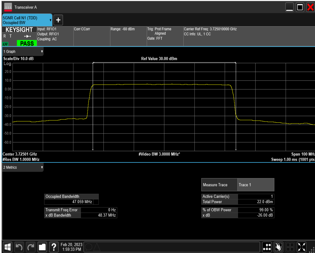
n77(3700-3980) SCS=30kHz CP_QPSK BW=50MHz Channel=648334 RB=133@0
