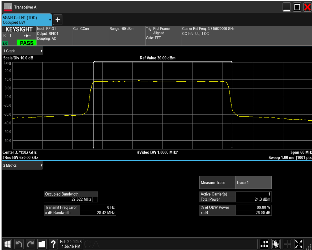
n77(3700-3980) SCS=30kHz DFT_QAM64 BW=30MHz Channel=647668 RB=75@0
