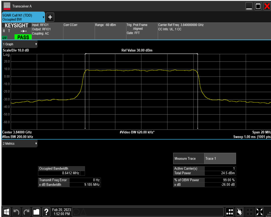
n77(3700-3980) SCS=30kHz DFT_QAM64 BW=10MHz Channel=656000 RB=24@0
