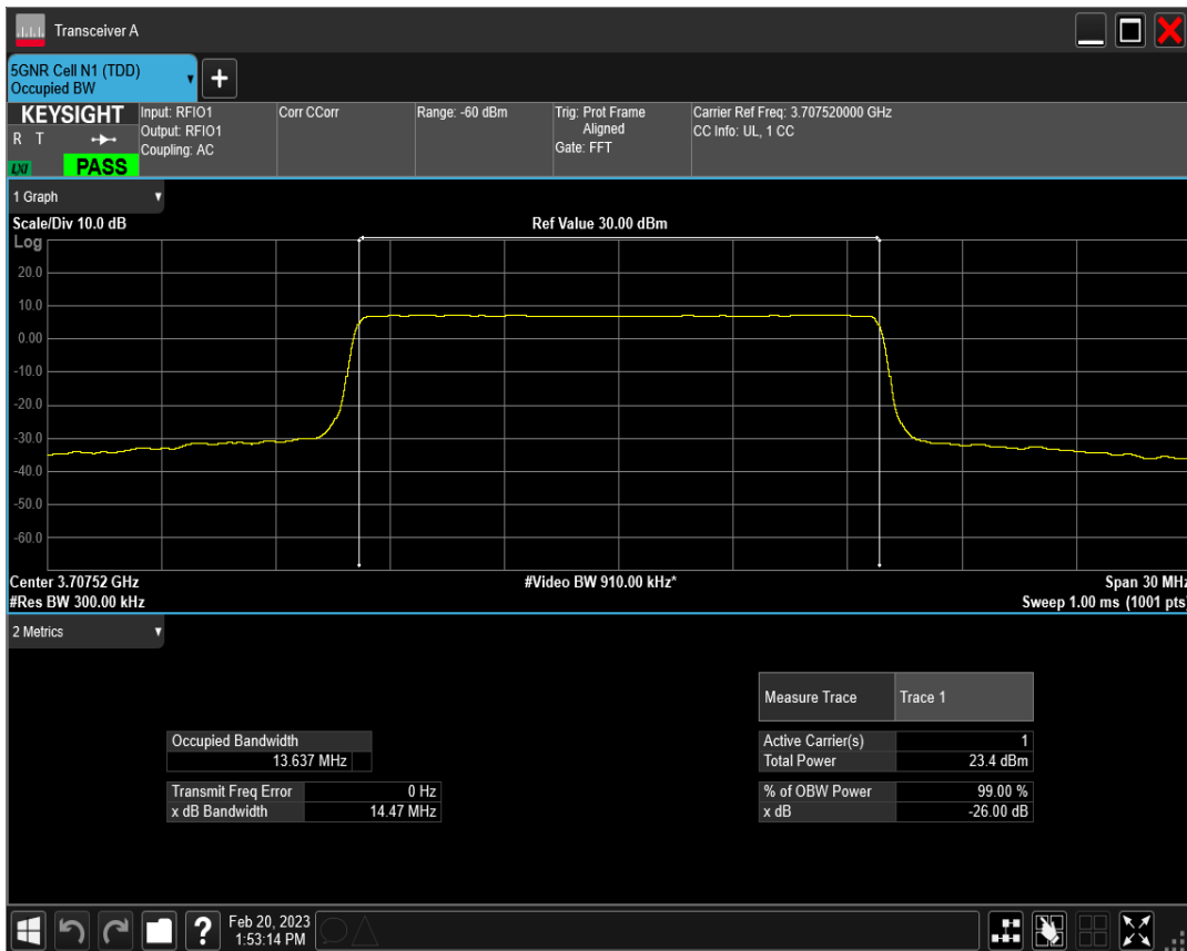
n77(3700-3980) SCS=30kHz DFT_BPSK BW=15MHz Channel=656000 RB=36@0
