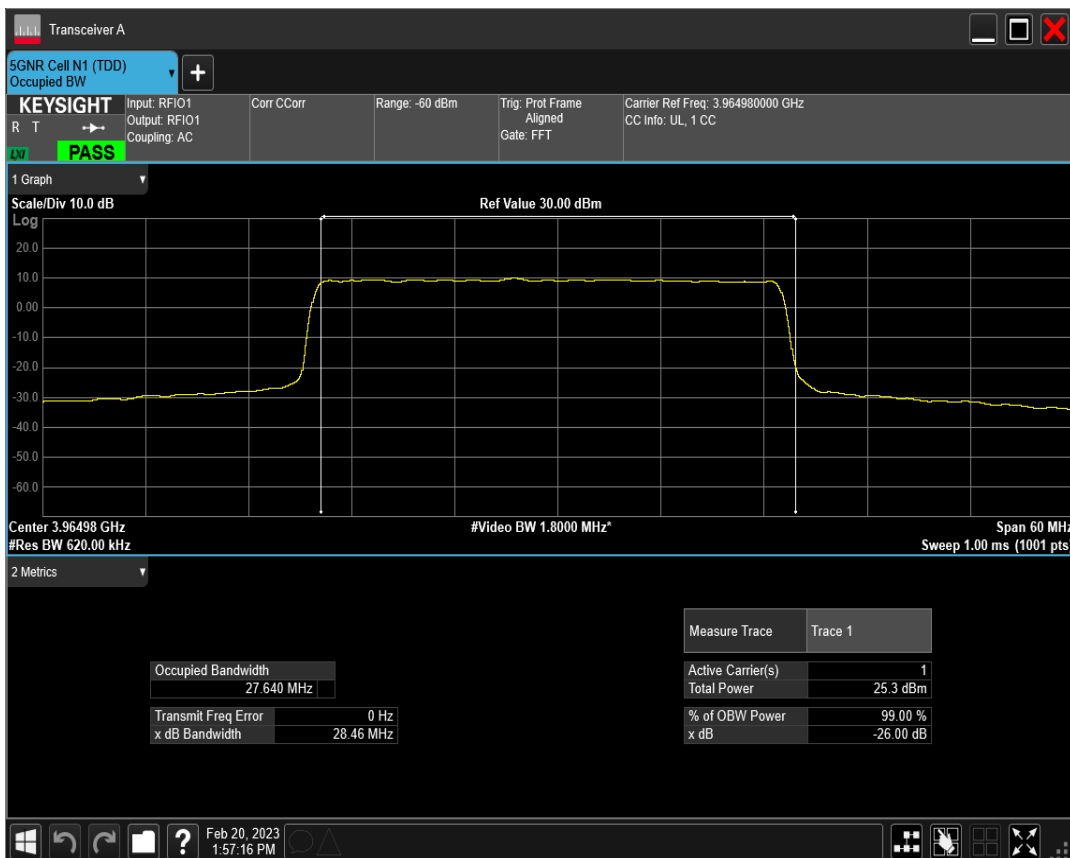
n77(3700-3980) SCS=30kHz DFT_QAM16 BW=30MHz Channel=664332 RB=75@0
