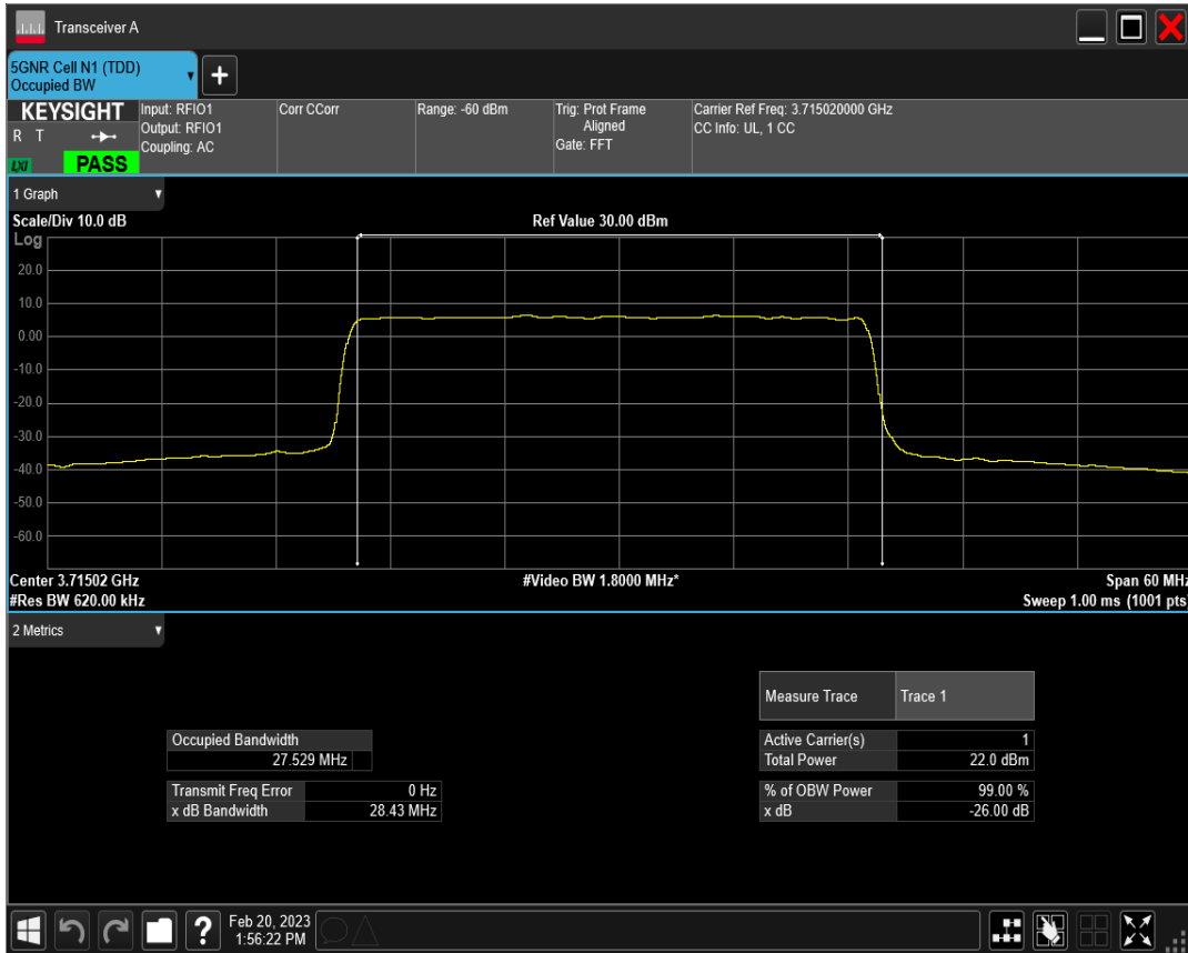
n77(3700-3980) SCS=30kHz CP_QPSK BW=30MHz Channel=647668 RB=78@0
