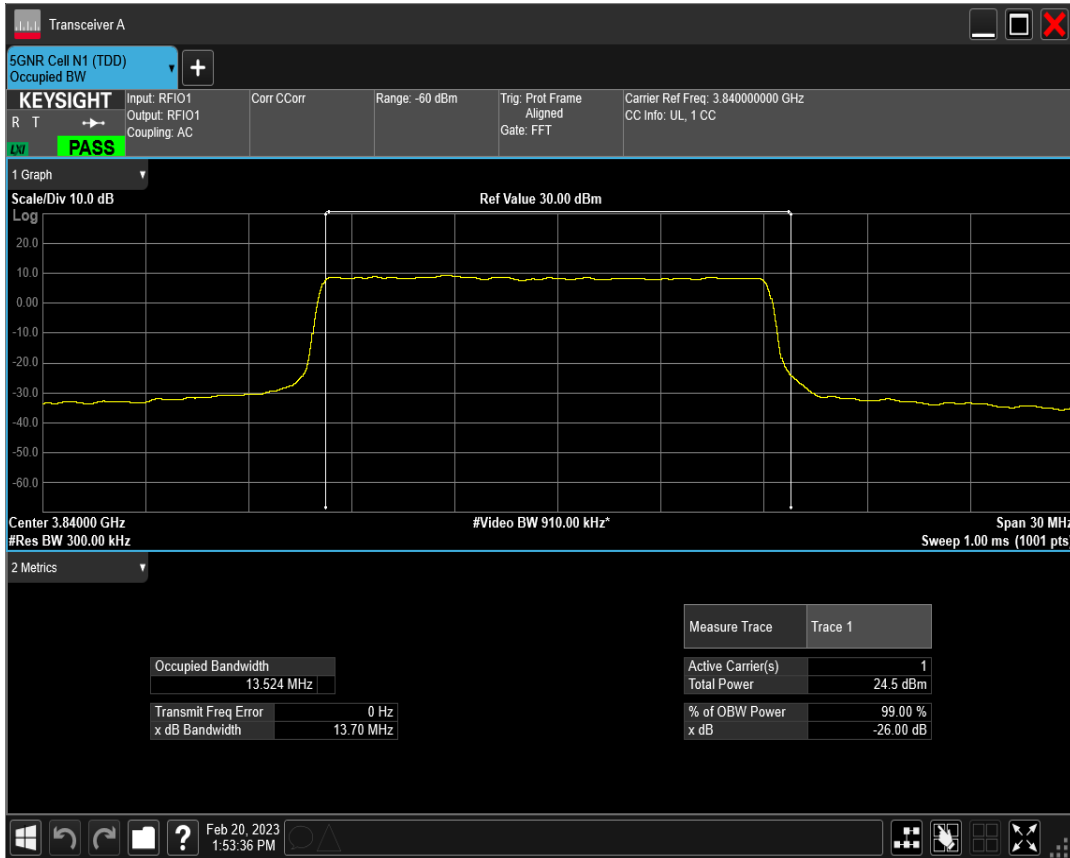
n77(3700-3980) SCS=30kHz DFT_QAM64 BW=15MHz Channel=656000 RB=36@0
