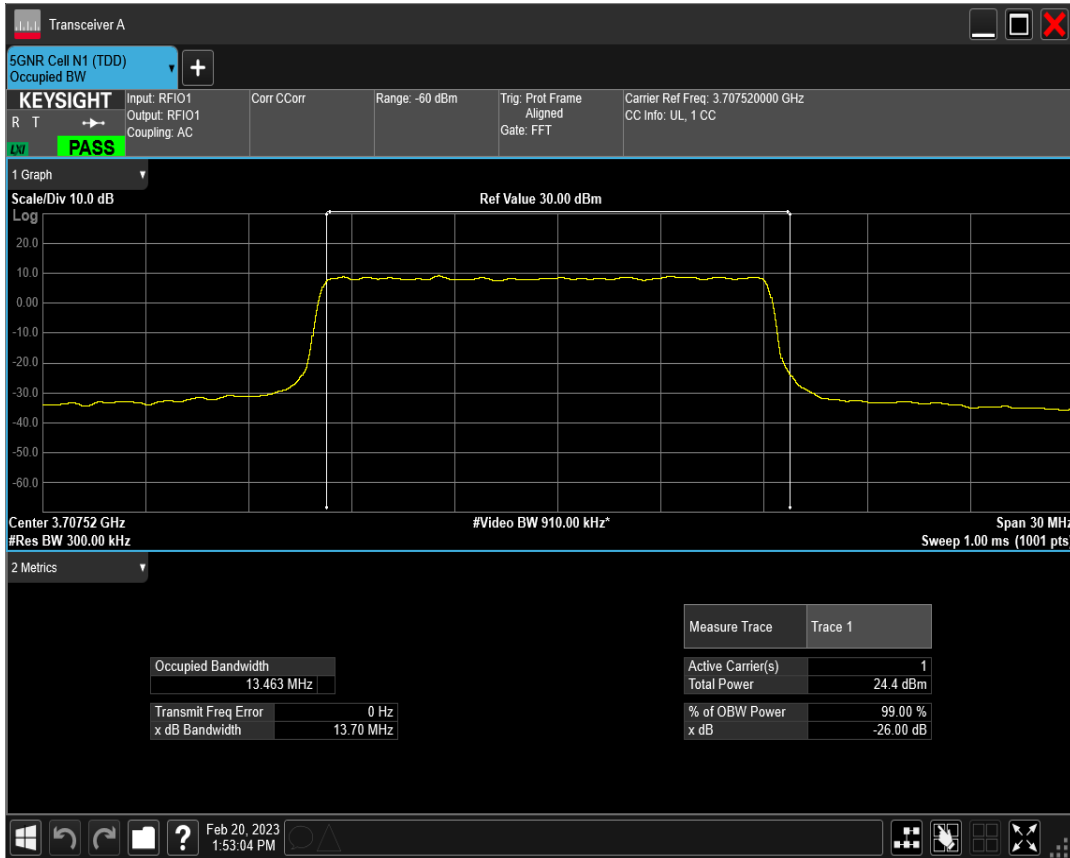
n77(3700-3980) SCS=30kHz DFT_QAM64 BW=15MHz Channel=647168 RB=36@0
