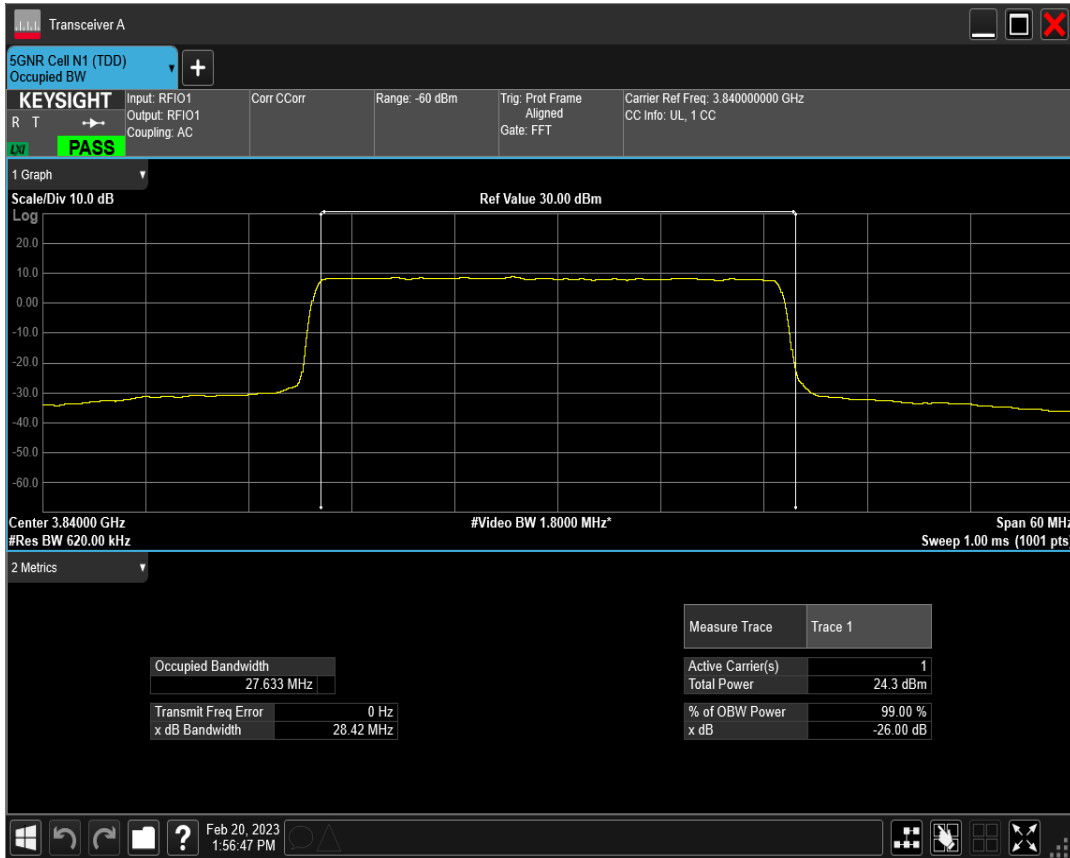
n77(3700-3980) SCS=30kHz DFT_QAM64 BW=30MHz Channel=656000 RB=75@0
