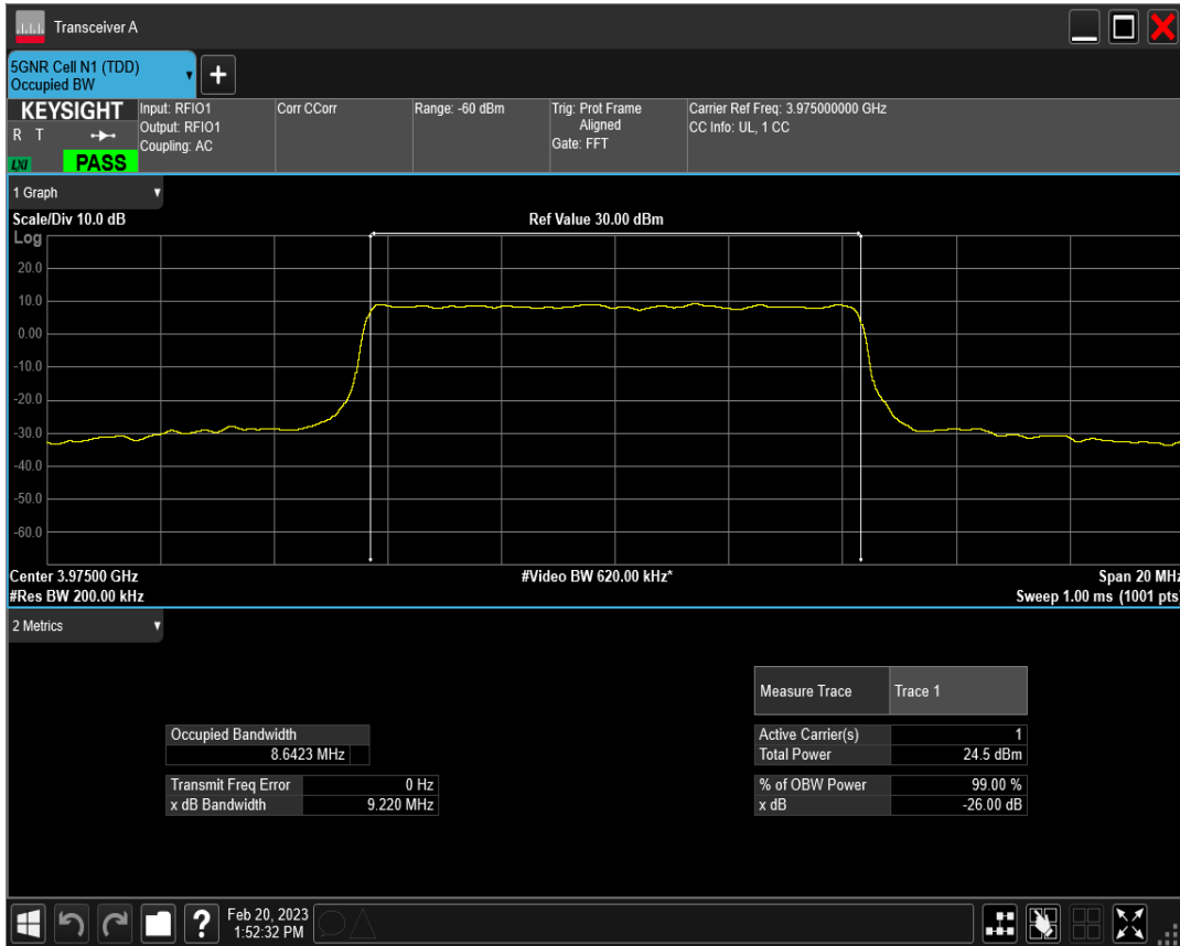
n77(3700-3980) SCS=30kHz DFT_QAM64 BW=10MHz Channel=665000 RB=24@0
