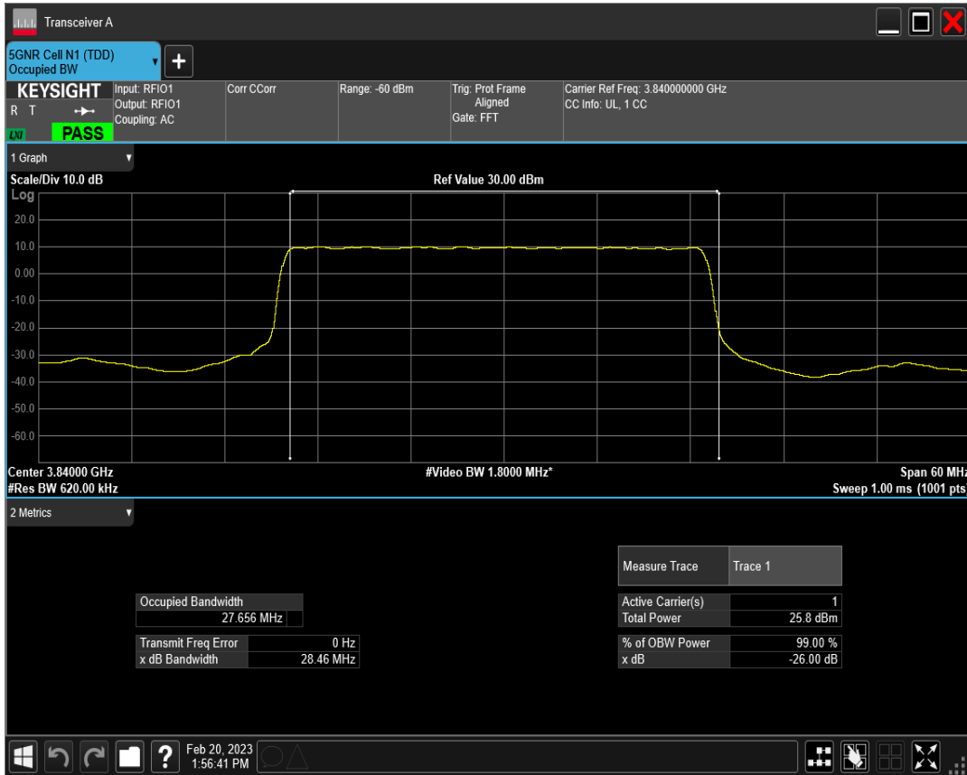
n77(3700-3980) SCS=30kHz DFT_QPSK BW=30MHz Channel=656000 RB=75@0
