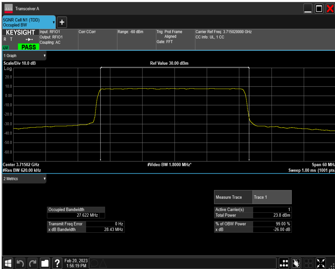
n77(3700-3980) SCS=30kHz DFT_QAM256 BW=30MHz Channel=647668 RB=75@0
