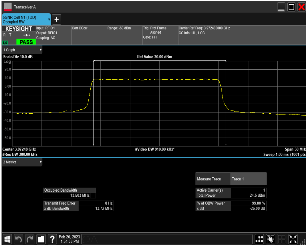
n77(3700-3980) SCS=30kHz DFT_QAM64 BW=15MHz Channel=664832 RB=36@0
