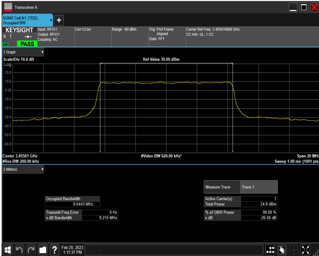
n77(3450-3550) SCS=30kHz DFT_QAM64 BW=10MHz Channel=630334 RB=24@0
