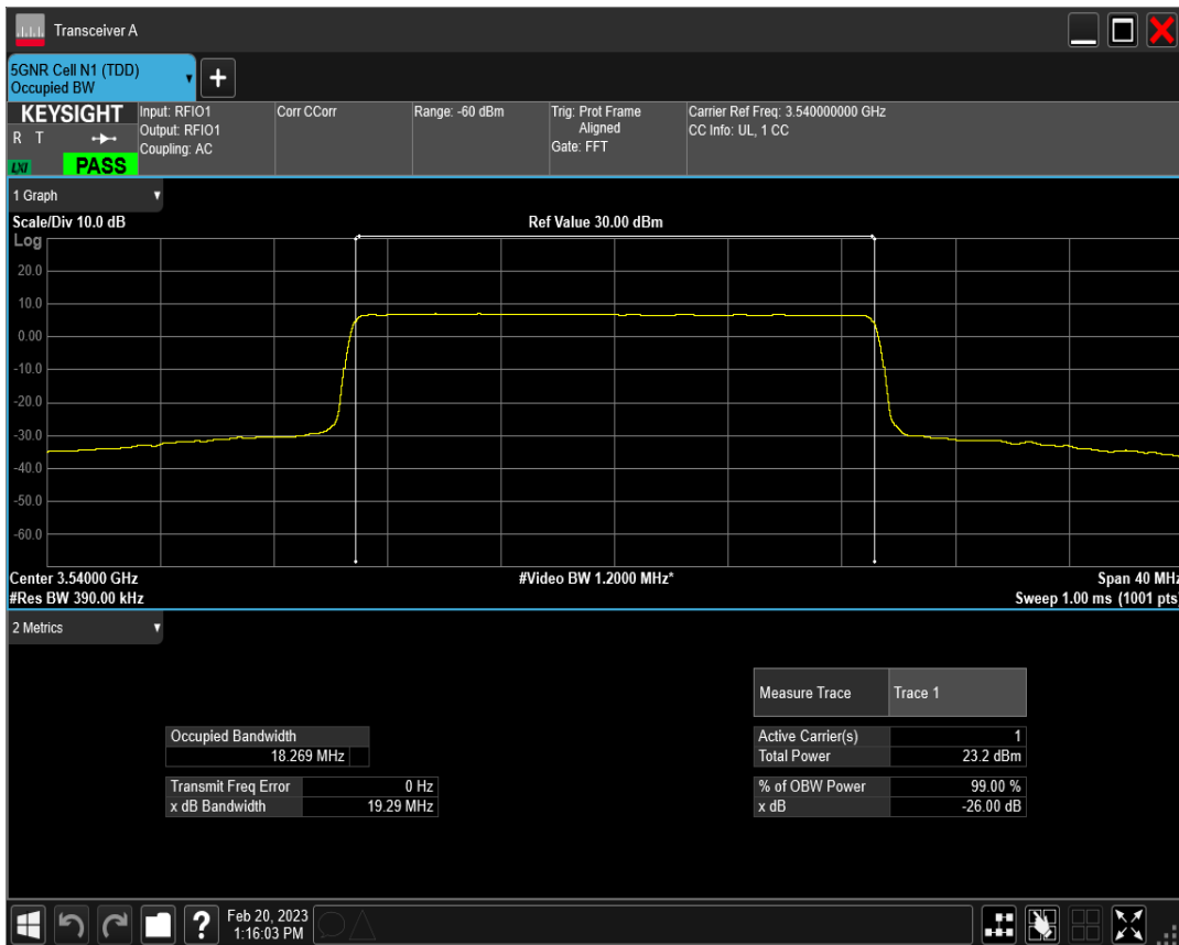
n77(3450-3550) SCS=30kHz DFT_BPSK BW=30MHz Channel=631000 RB=75 @0
