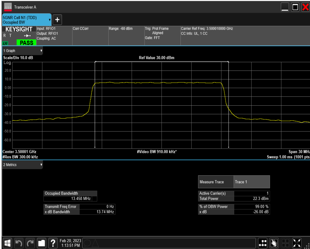
n77(3450-3550) SCS=30kHz CP_QPSK BW=15MHz Channel=633334 RB=38@0
