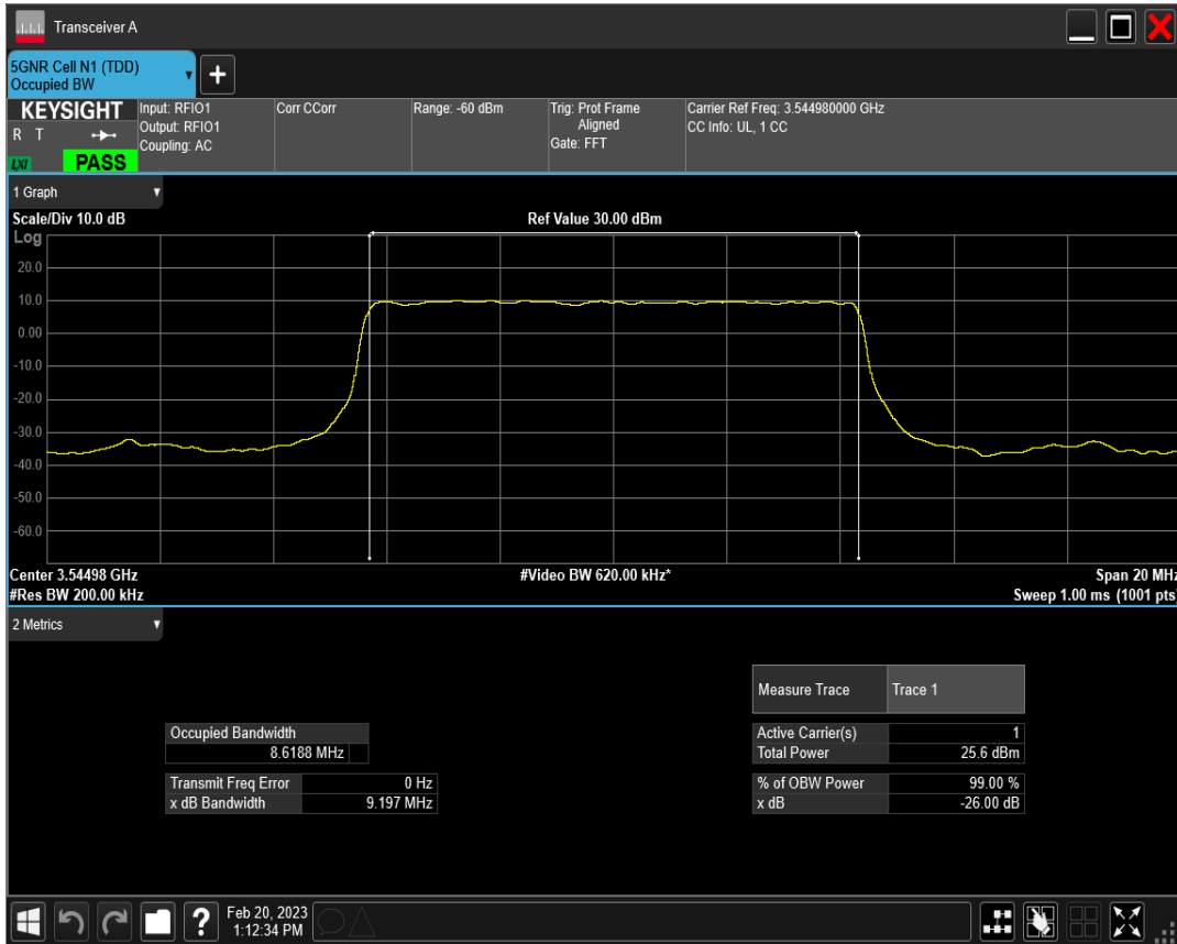
n77(3450-3550) SCS=30kHz DFT_QPSK BW=10MHz Channel=636332 RB=24@0
