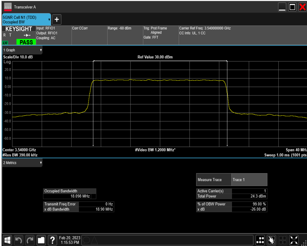
n77(3450-3550) SCS=30kHz DFT_QAM64 BW=20MHz Channel=636000 RB=50@0
