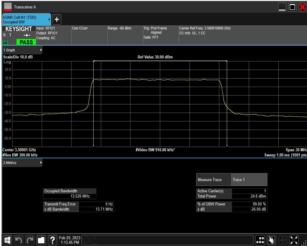
n77(3450-3550) SCS=30kHz DFT_QAM64 BW=15MHz Channel=633334 RB=36@0
