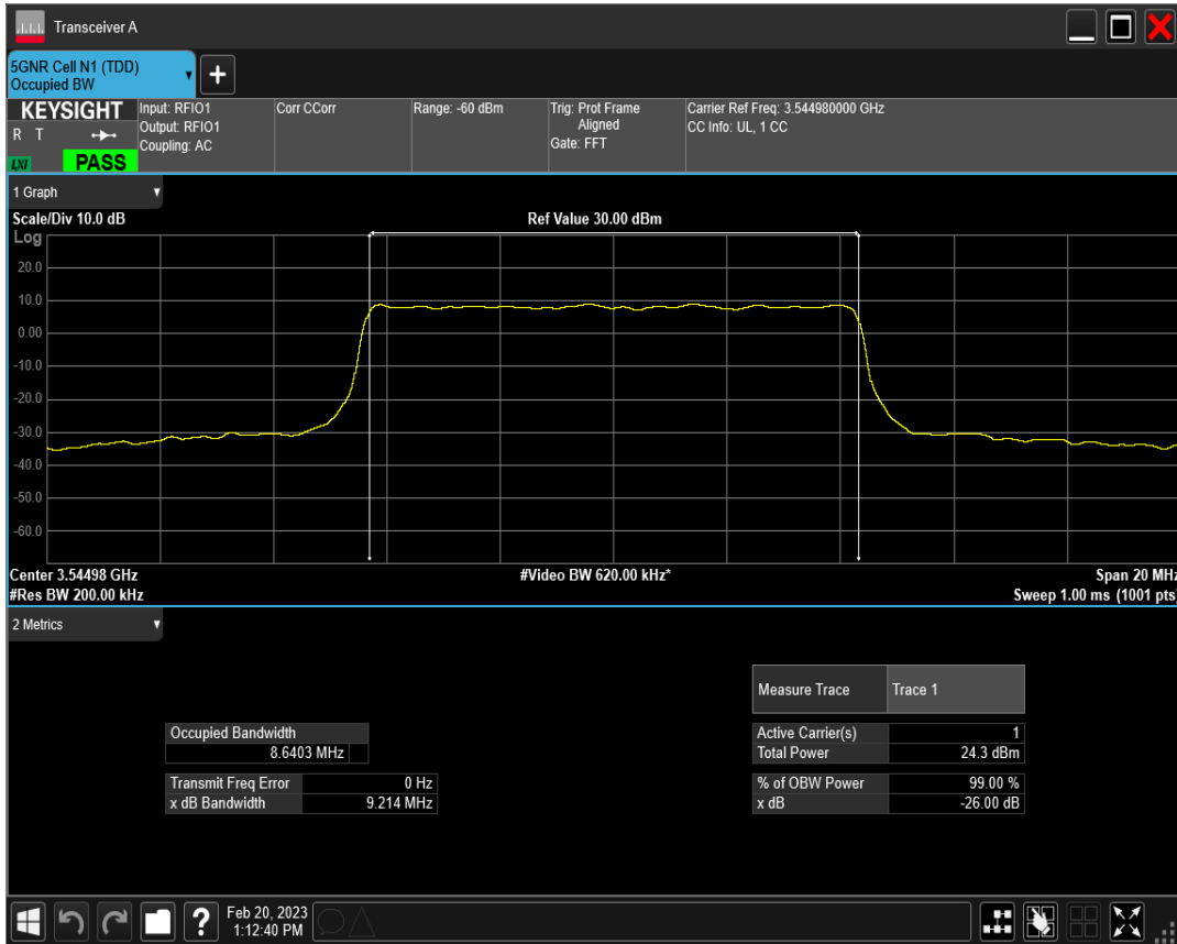
n77(3450-3550) SCS=30kHz DFT_QAM64 BW=10MHz Channel=636332 RB=24@0
