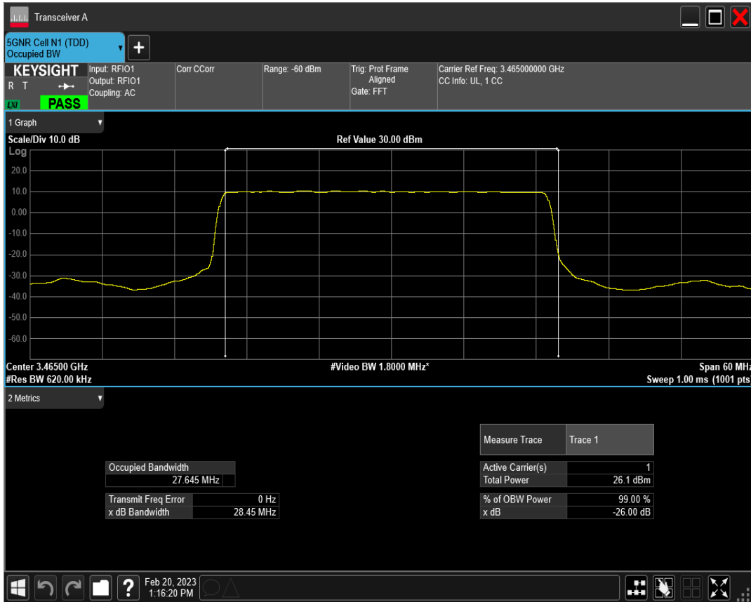
n77(3450-3550) SCS=30kHz DFT_QPSK BW=30MHz Channel=631000 RB=75@0
