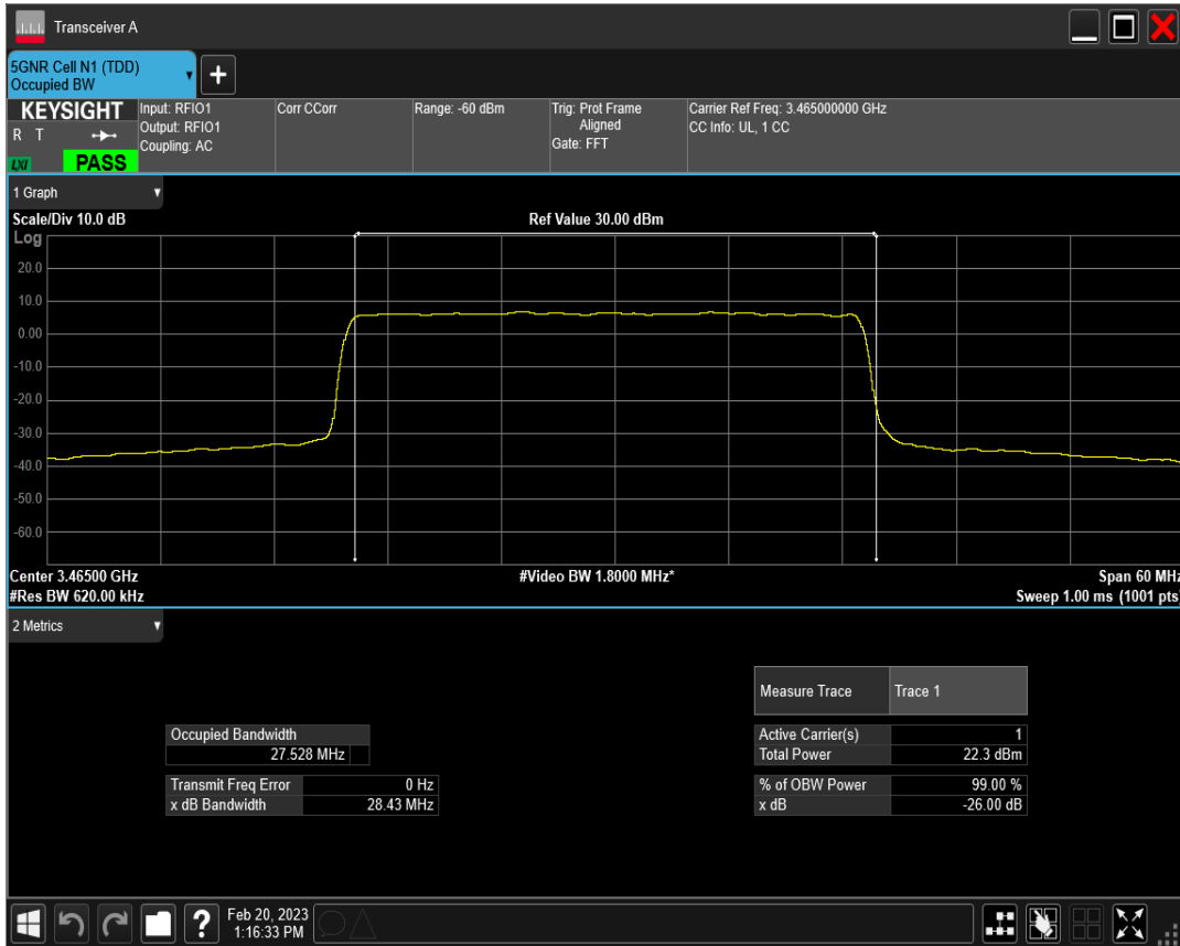
n77(3450-3550) SCS=30kHz CP_QPSK BW=30MHz Channel=631000 RB=78@0
