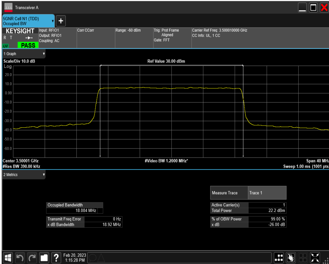
n77(3450-3550) SCS=30kHz CP_QPSK BW=20MHz Channel=633334 RB=51 @0
