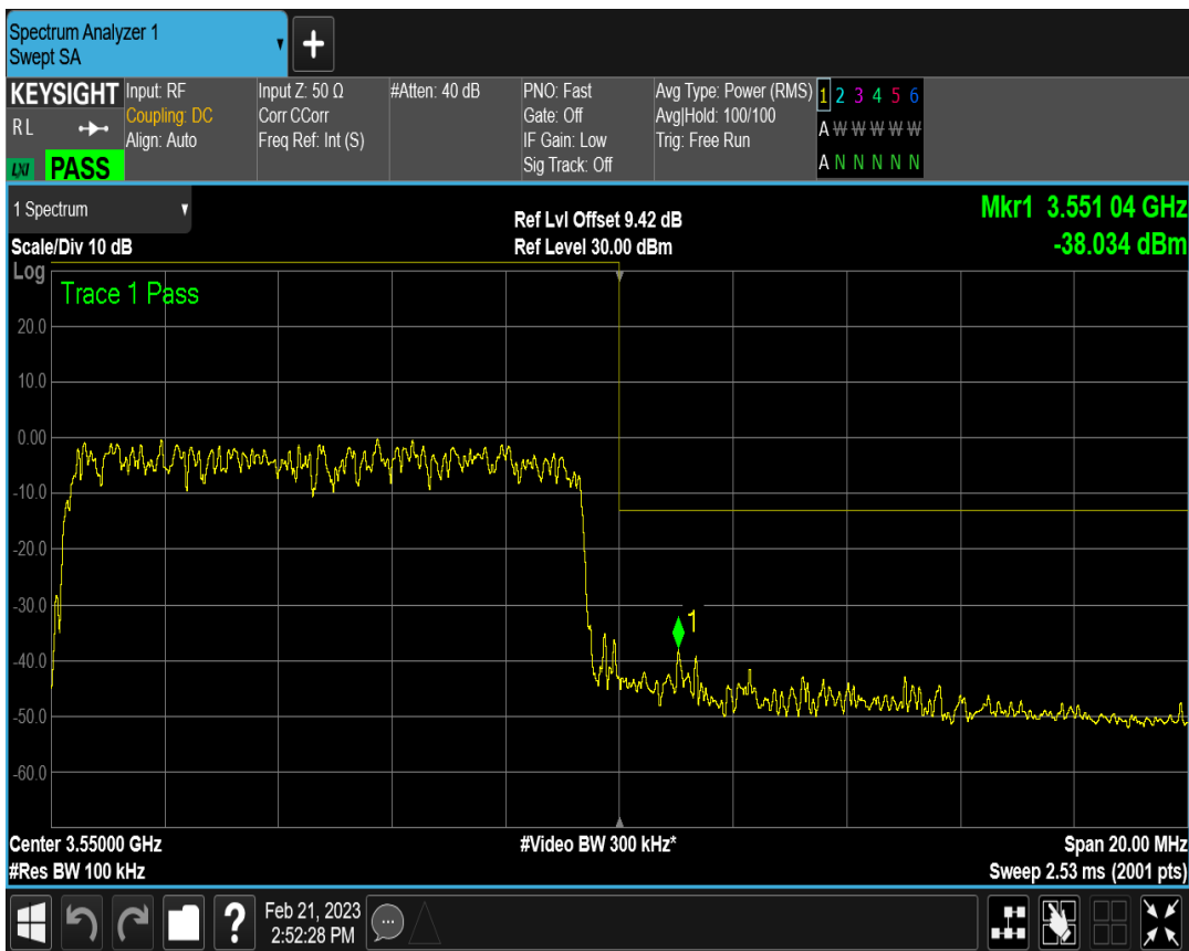
n77(3450-3550) SCS=15kHz DFT_QPSK BW=10MHz Channel=636332 RB=1@51
