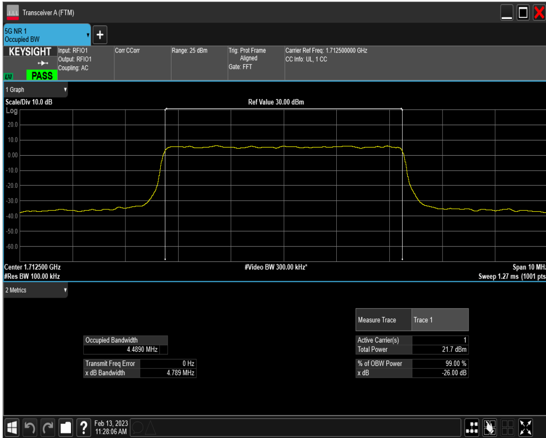
n66 SCS=15kHz DFT_QAM16 BW=5MHz Channel=342500 RB=25@0
