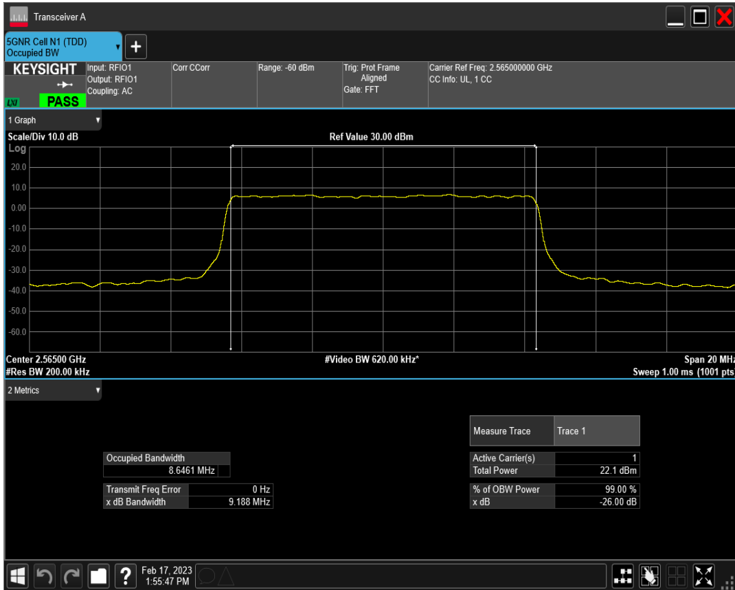
n7 SCS=30kHz DFT_QAM16 BW=10MHz Channel=513000 RB=24@0
