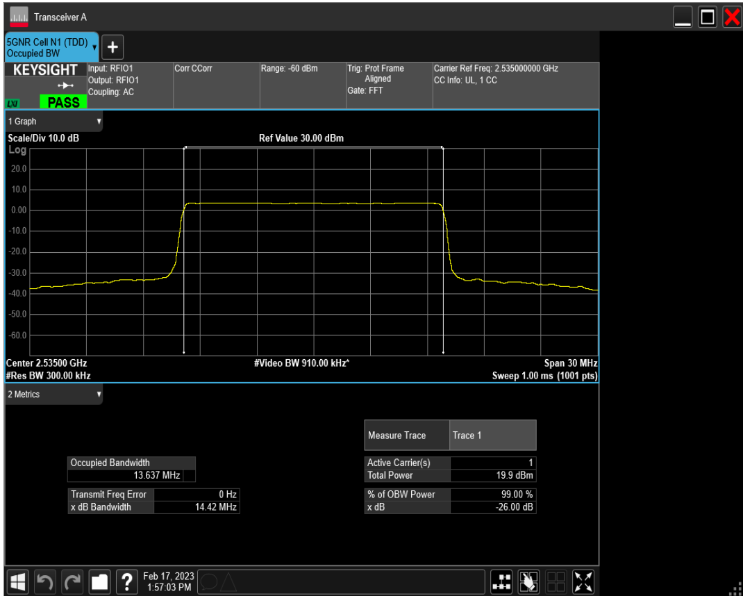
n7 SCS=30kHz DFT_BPSK BW=15MHz Channel=512500 RB=36@0
