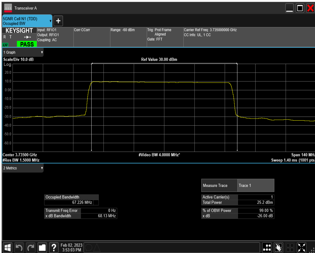
n78(3700-3800) SCS=30kHz DFT_QAM64 BW=70MHz Channel=649000 RB=180@0
