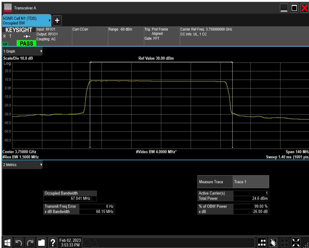
n78(3700-3800) SCS=30kHz CP_QPSK BW=70MHz Channel=650000 RB=189@0
