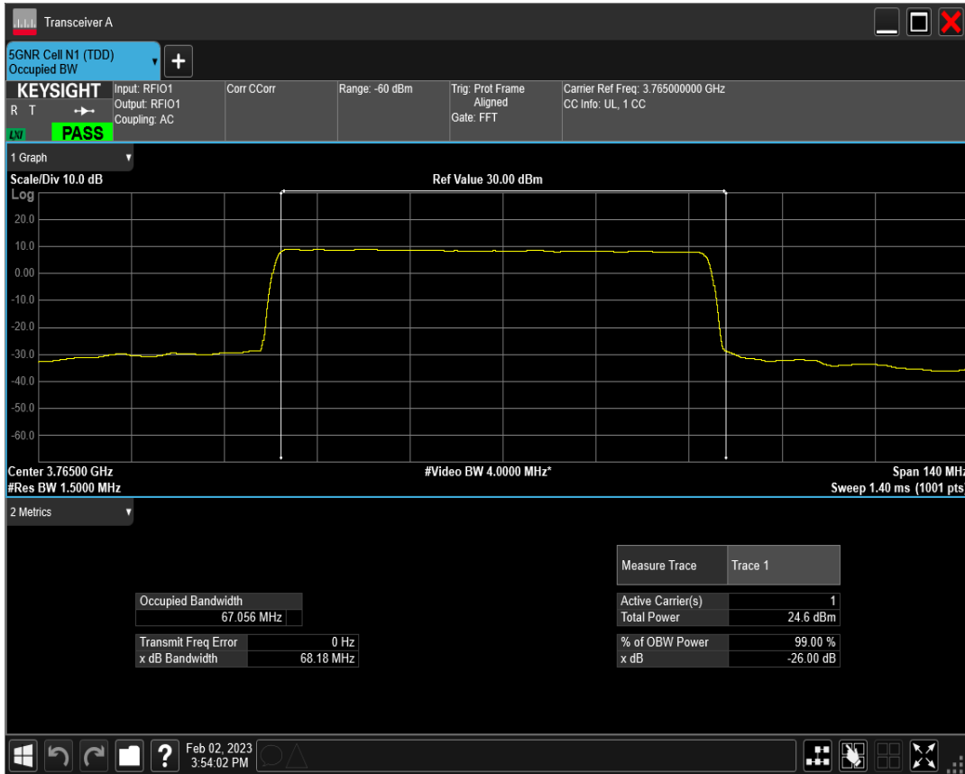
n78(3700-3800) SCS=30kHz CP_QPSK BW=70MHz Channel=651000 RB=189@0
