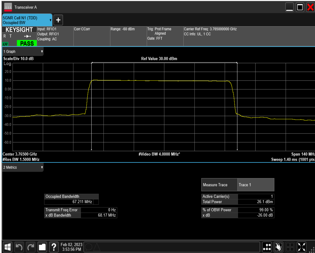
n78(3700-3800) SCS=30kHz DFT_QAM16 BW=70MHz Channel=651000 RB=180@0
