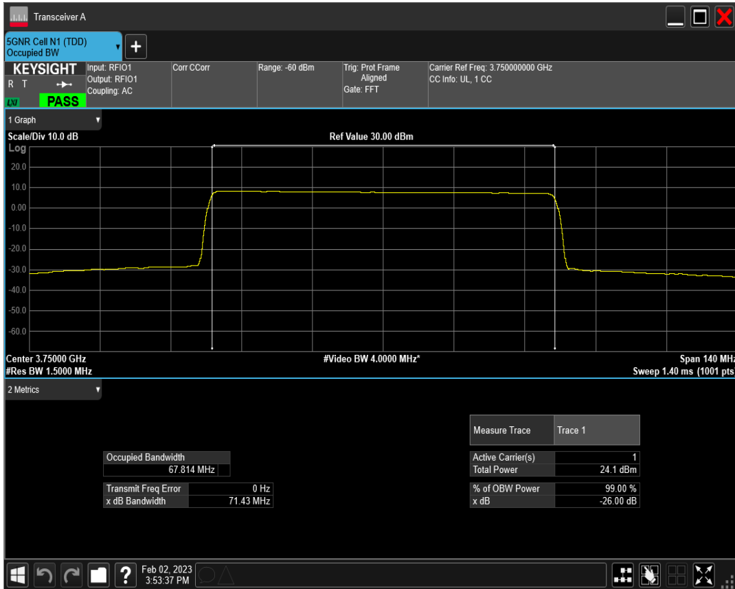
n78(3700-3800) SCS=30kHz DFT_BPSK BW=70MHz Channel=651000 RB=180@0
