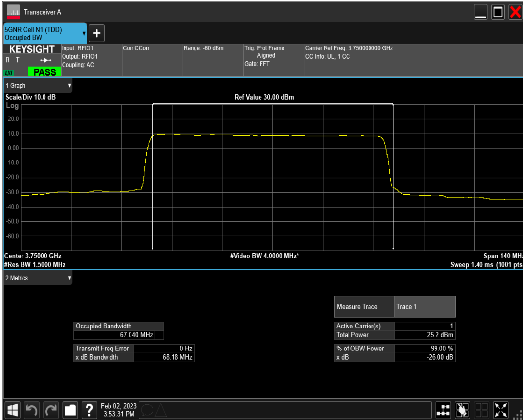
n78(3700-3800) SCS=30kHz DFT_QAM64 BW=70MHz Channel=650000 RB=180@0
