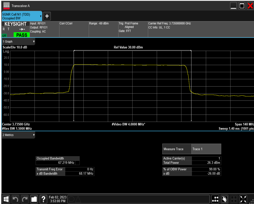
n78(3700-3800) SCS=30kHz DFT_QAM16 BW=70MHz Channel=649000 RB=180@0
