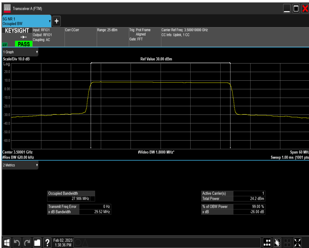
n77(3450-3550) SCS=30kHz DFT_BPSK BW=30MHz Channel=635666 RB=75@0
