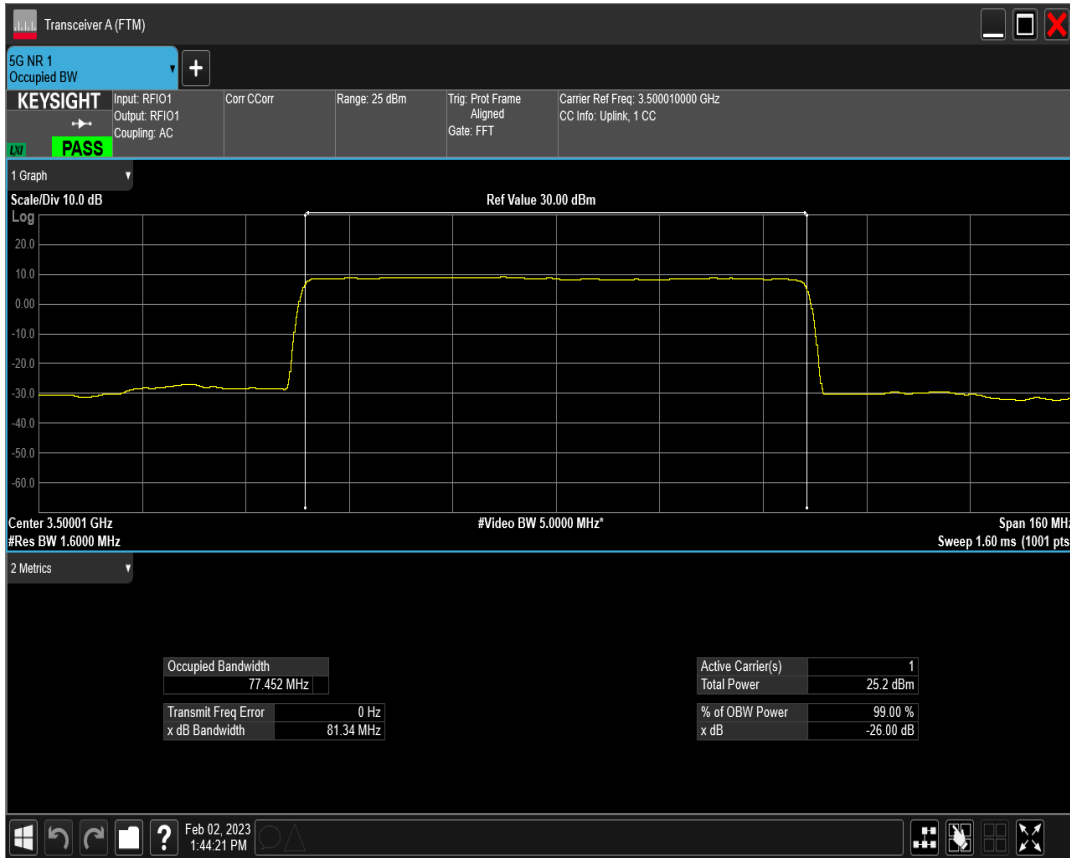
n77(3450-3550) SCS=30kHz DFT_QAM64 BW=80MHz Channel=633334 RB=216@0
