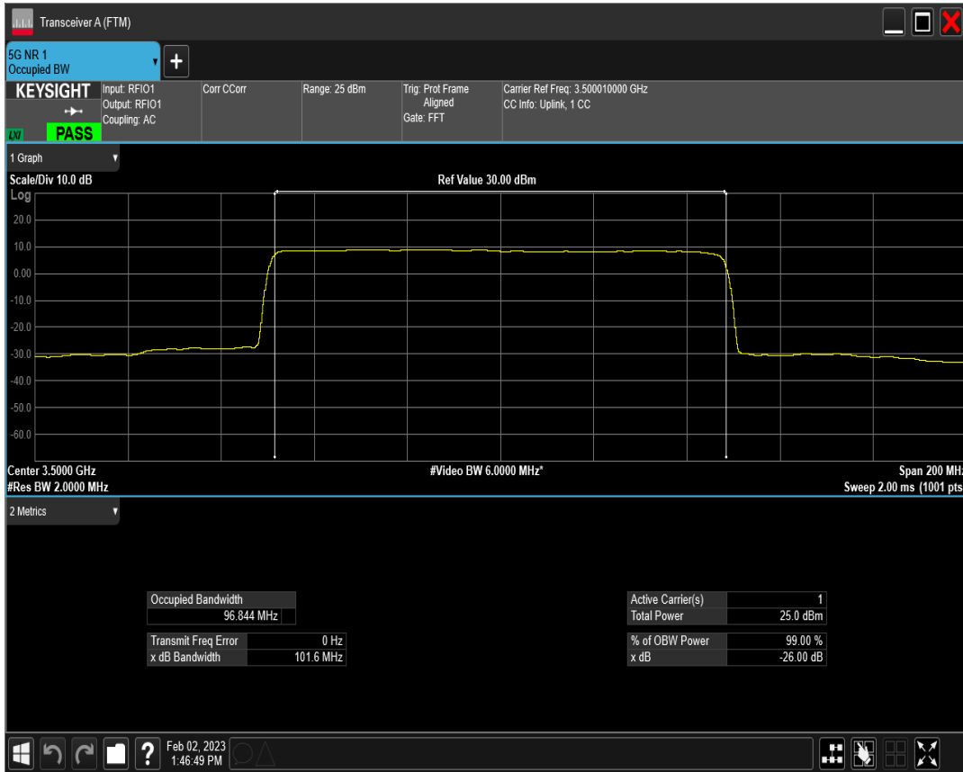
n77(3450-3550) SCS=30kHz DFT_QAM64 BW=100MHz Channel=633334 RB=270@0
