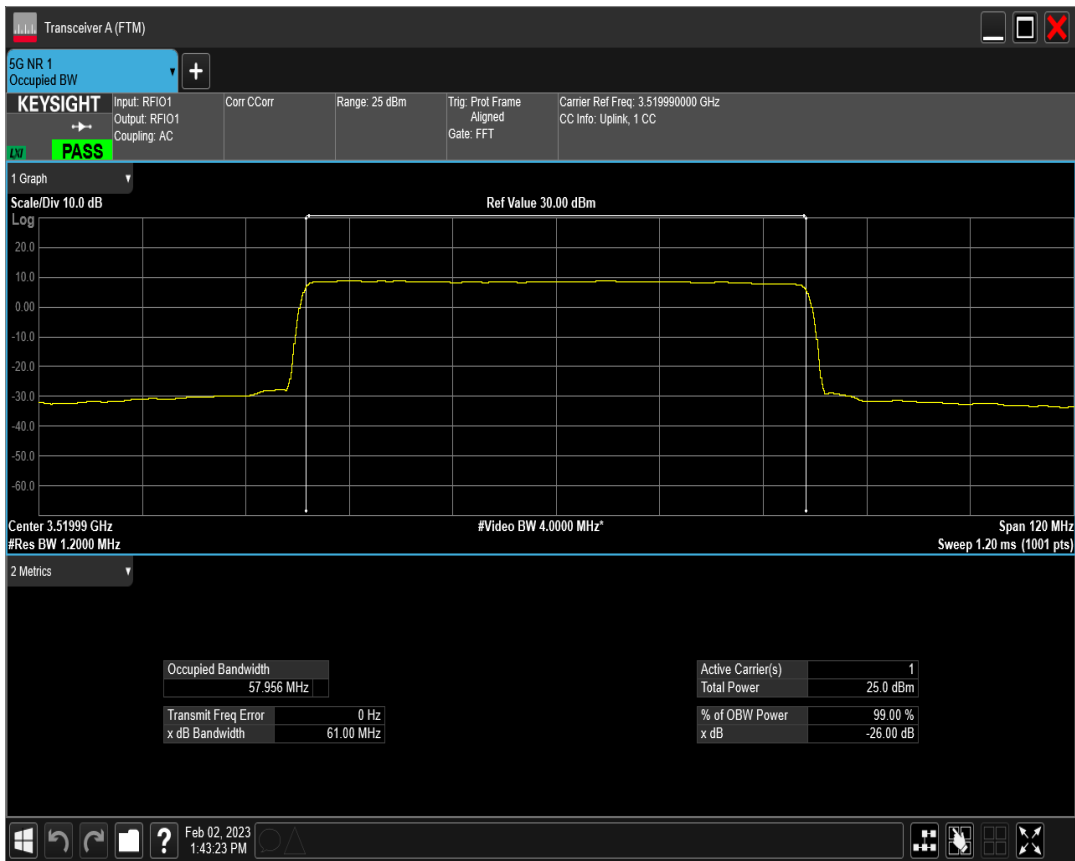
n77(3450-3550) SCS=30kHz DFT_QAM64 BW=60MHz Channel=634666 RB=162@0
