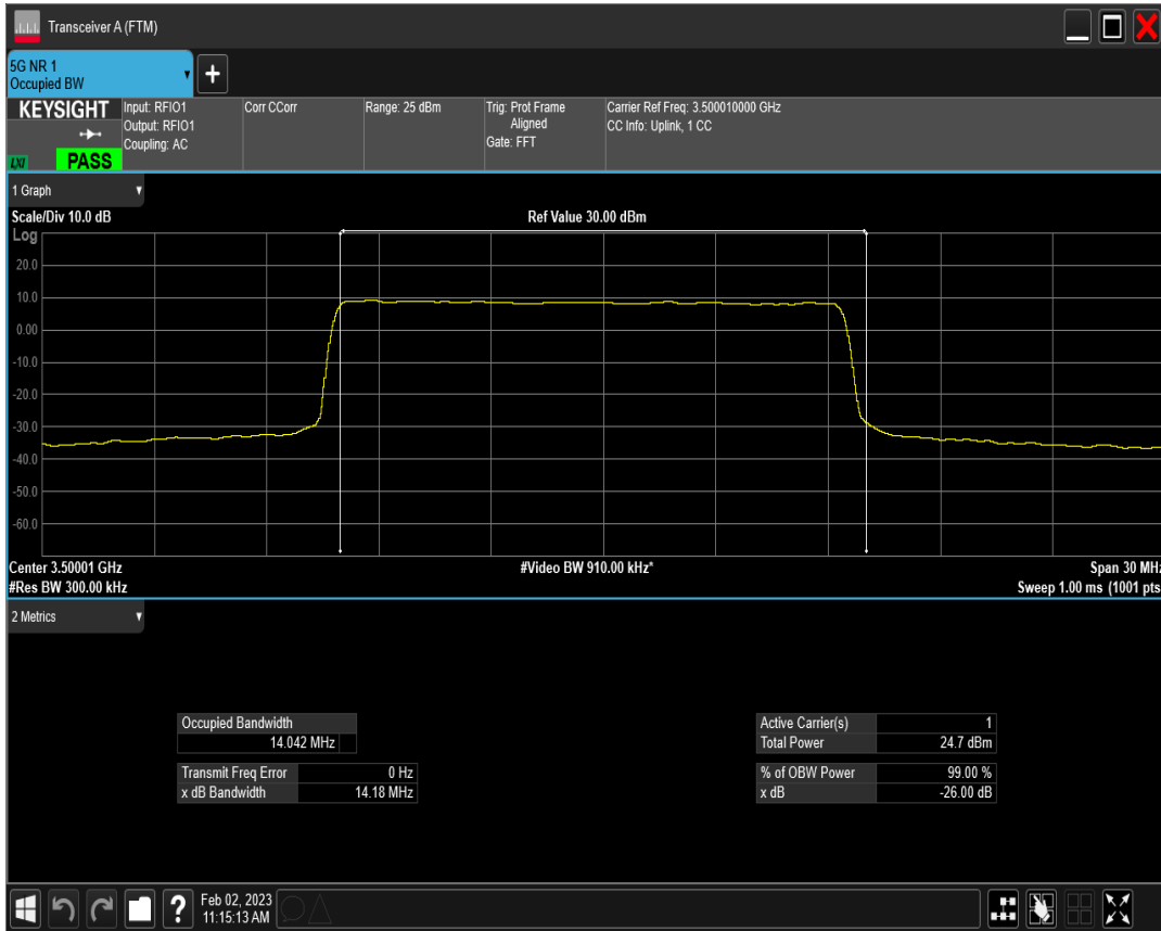
n77(3450-3550) SCS=15kHz DFT_QAM64 BW=15MHz Channel=633334 RB=75@0
