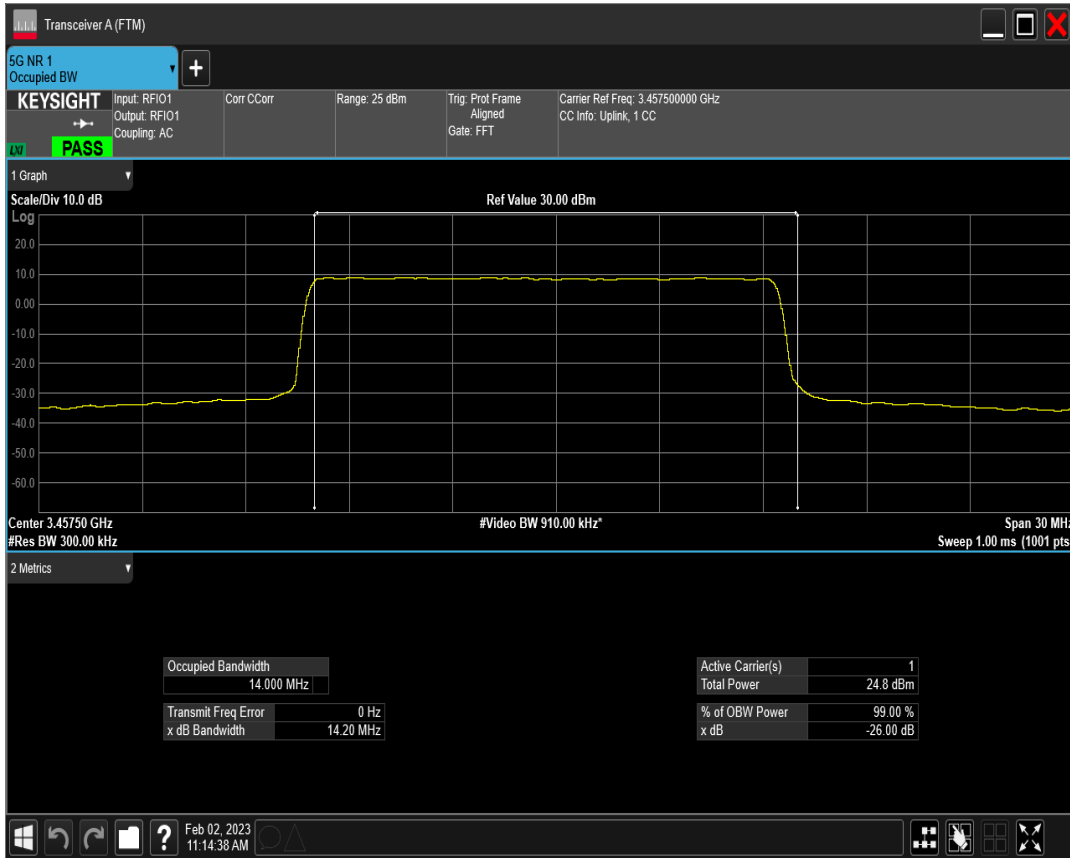
n77(3450-3550) SCS=15kHz DFT_QAM64 BW=15MHz Channel=630500 RB=75@0
