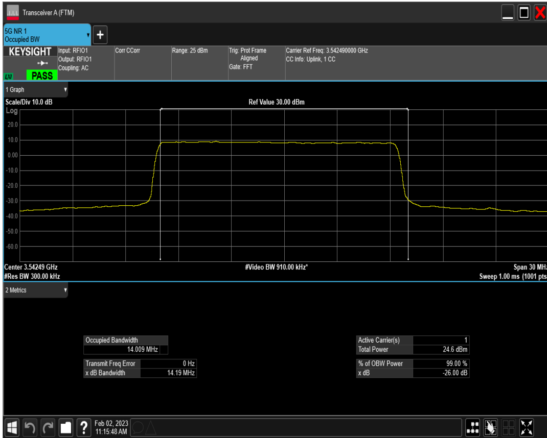
n77(3450-3550) SCS=15kHz DFT_QAM64 BW=15MHz Channel=636166 RB=75@0
