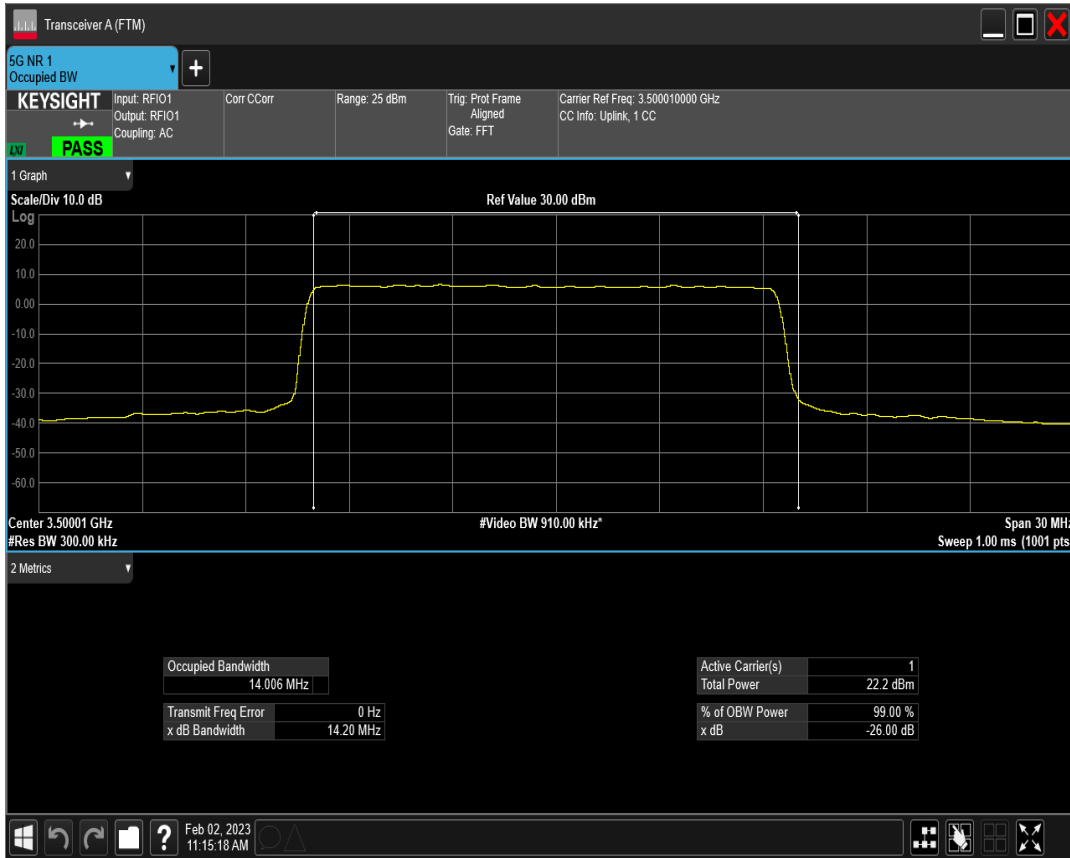
n77(3450-3550) SCS=15kHz CP_QPSK BW=15MHz Channel=633334 RB=79@0
