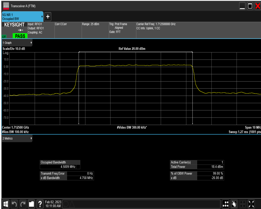
n66 SCS=15kHz DFT_QAM16 BW=5MHz Channel=342500 RB=25@0
