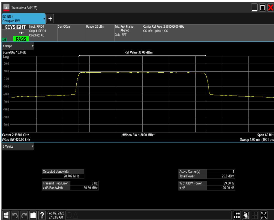
n41 SCS=15kHz DFT_QAM16 BW=30MHz Channel=518601 RB=160@0
