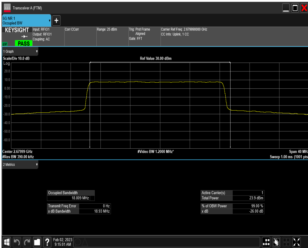
n41 SCS=15kHz DFT_QAM64 BW=20MHz Channel=535998 RB=100@0
