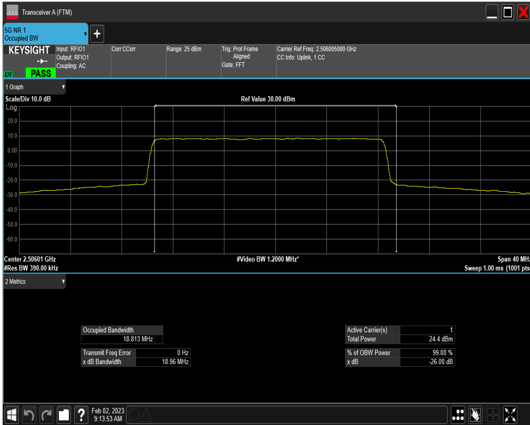
n41 SCS=15kHz DFT_QAM64 BW=20MHz Channel=501201 RB=100@0
