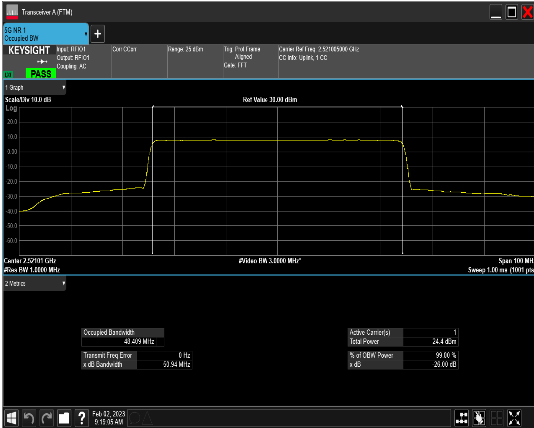
n41 SCS=15kHz DFT_QAM64 BW=50MHz Channel=504201 RB=270@0
