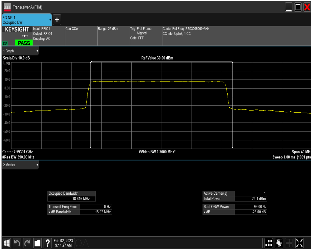
n41 SCS=15kHz DFT_QAM64 BW=20MHz Channel=518601 RB=100@0
