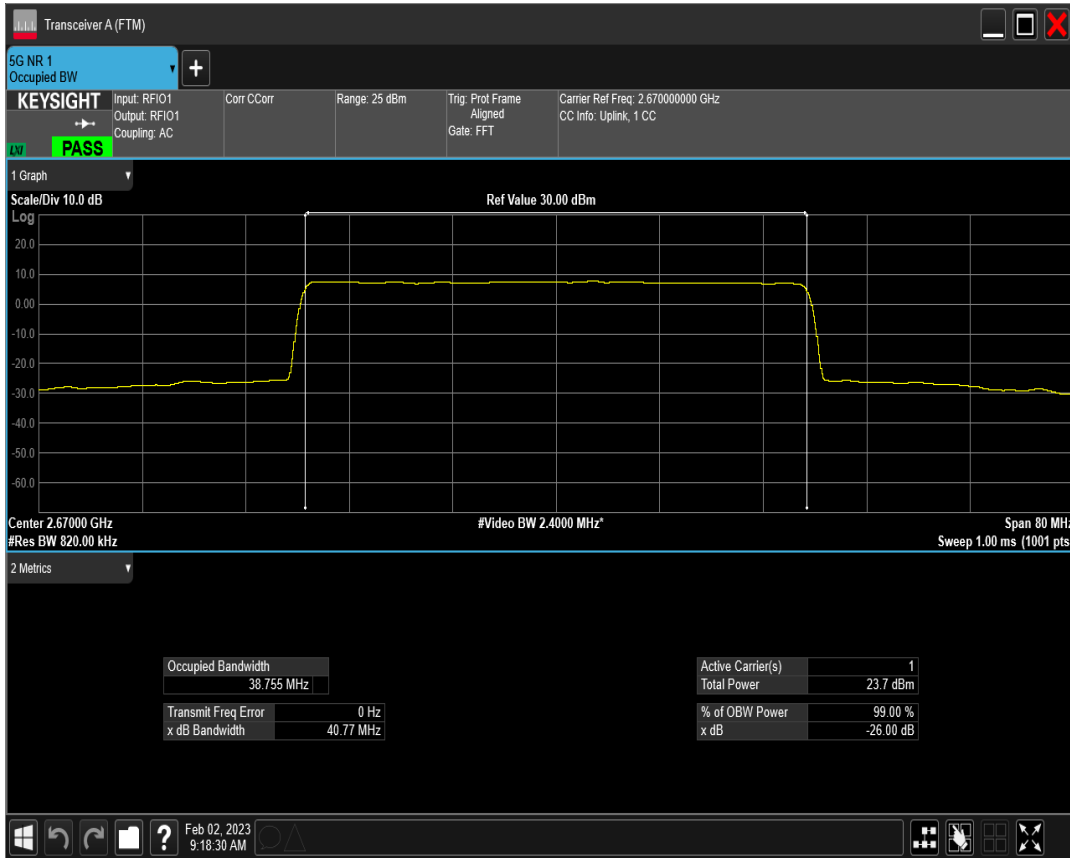
n41 SCS=15kHz DFT_QAM64 BW=40MHz Channel=534000 RB=216@0
