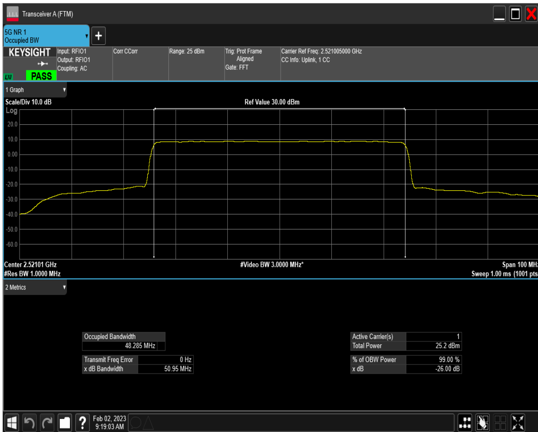
n41 SCS=15kHz DFT_QAM16 BW=50MHz Channel=504201 RB=270@0
