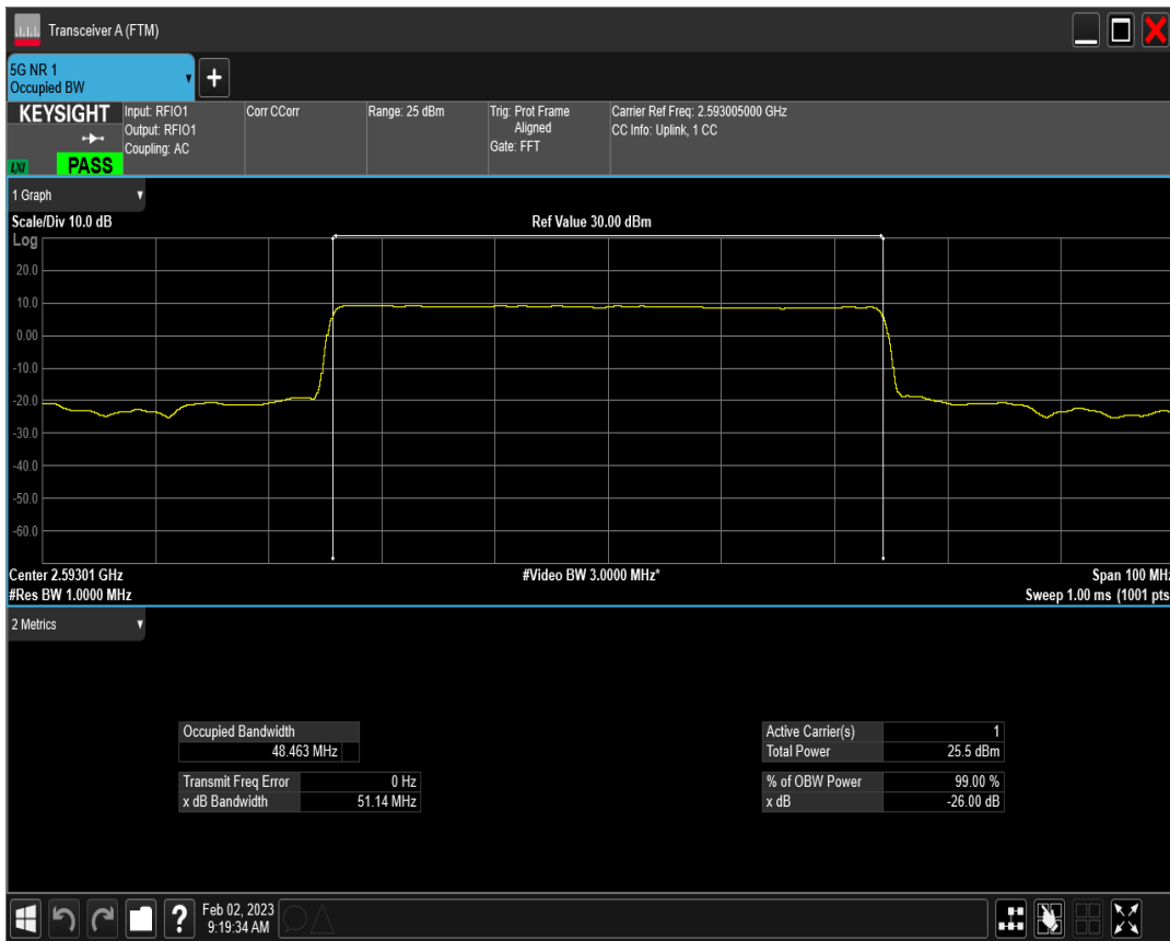
n41 SCS=15kHz DFT_QPSK BW=50MHz Channel=518601 RB=270@0
