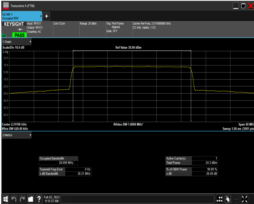
n41 SCS=15kHz DFT_QAM64 BW=30MHz Channel=502200 RB=160@0
