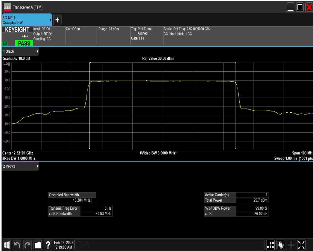
n41 SCS=15kHz DFT_QPSK BW=50MHz Channel=504201 RB=270@0
