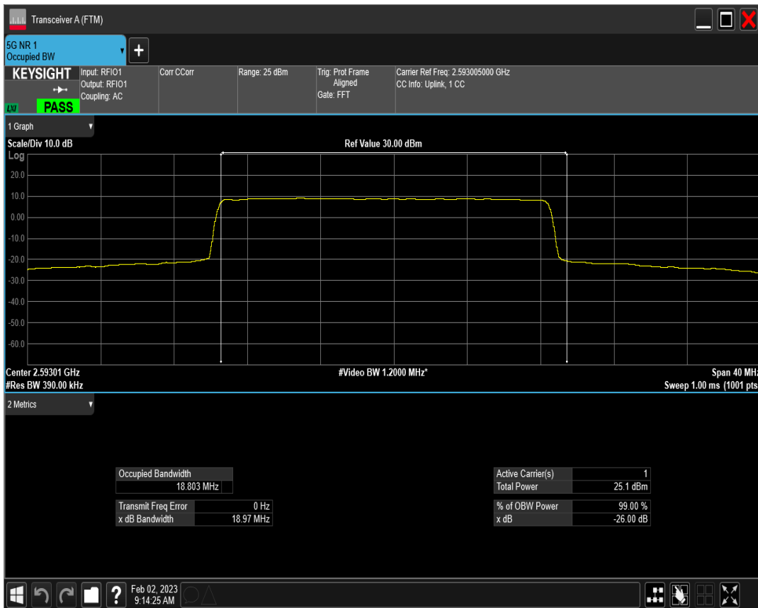
n41 SCS=15kHz DFT_QAM16 BW=20MHz Channel=518601 RB=100@0
