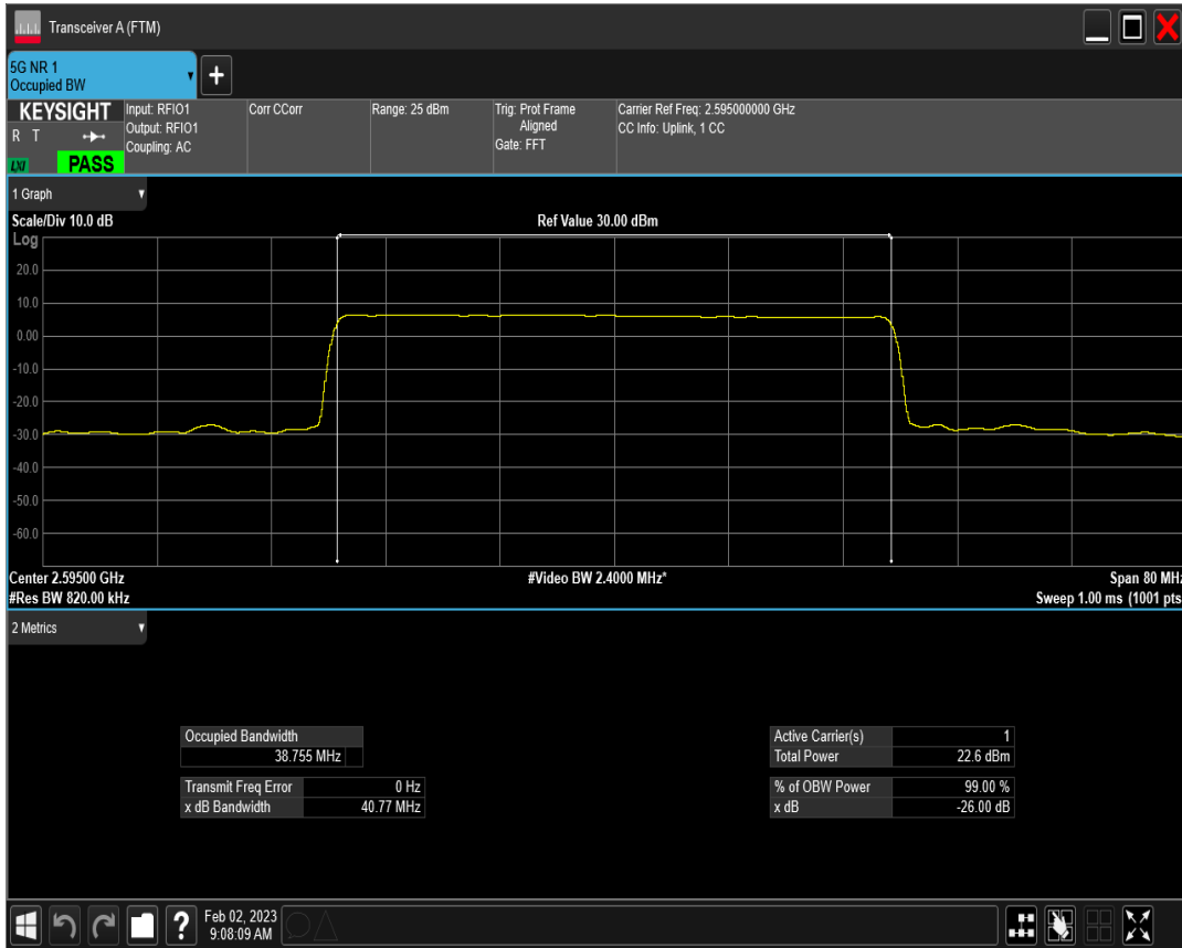
n38 SCS=15kHz DFT_QAM16 BW=40MHz Channel=519000 RB=216@0
