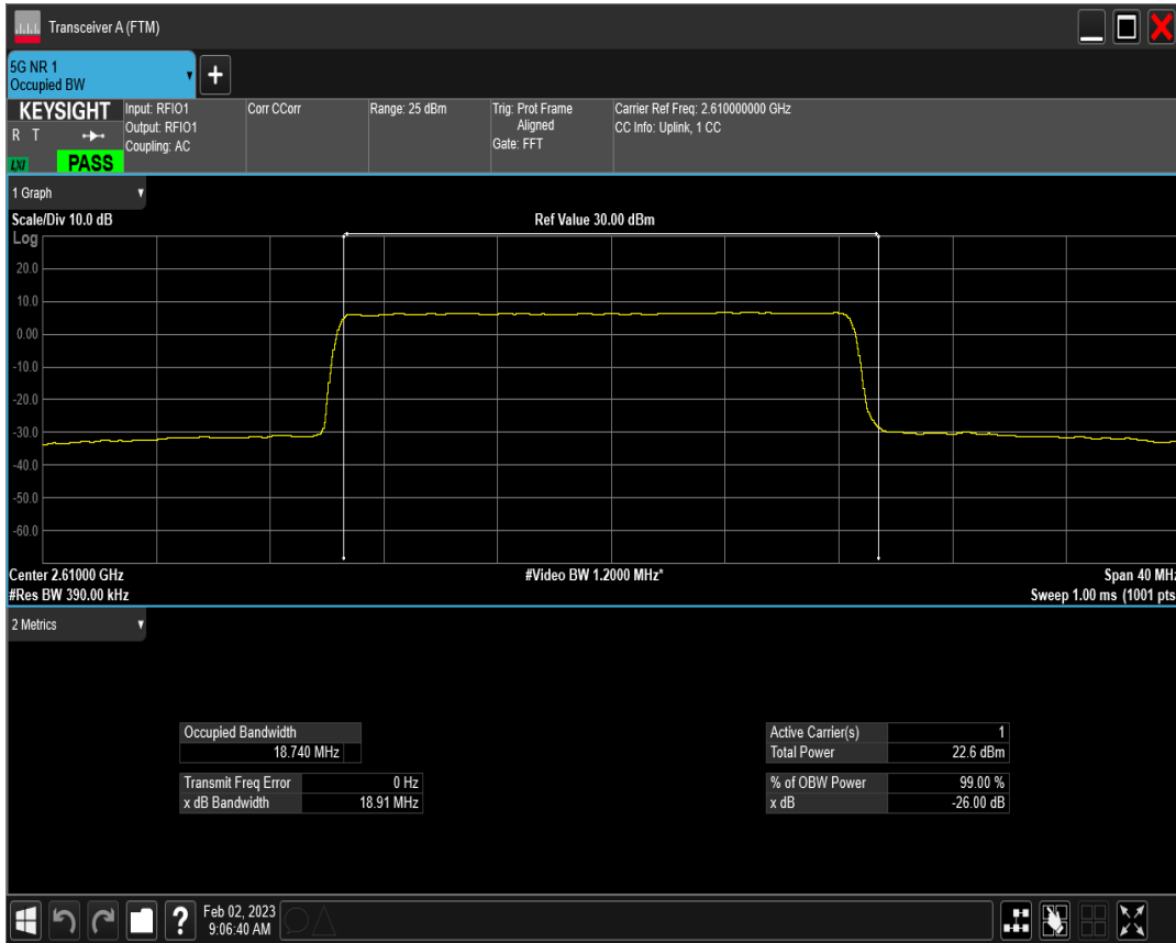
n38 SCS=15kHz DFT_QAM16 BW=20MHz Channel=522000 RB=100@0
