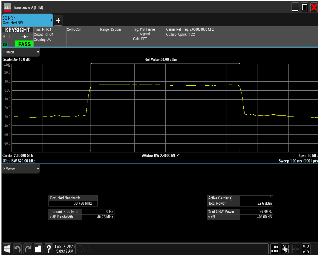
n38 SCS=15kHz DFT_QAM16 BW=40MHz Channel=520000 RB=216@0
