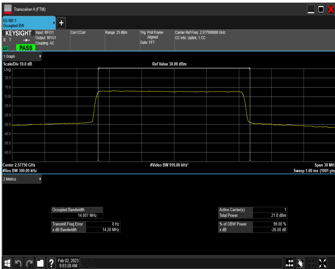
n38 SCS=15kHz DFT_QAM64 BW=15MHz Channel=515500 RB=75@0
