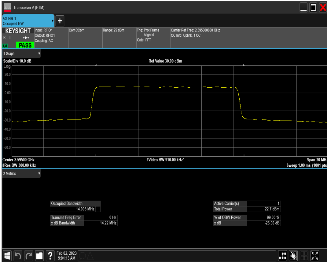
n38 SCS=15kHz DFT_QAM16 BW=15MHz Channel=519000 RB=75@0
