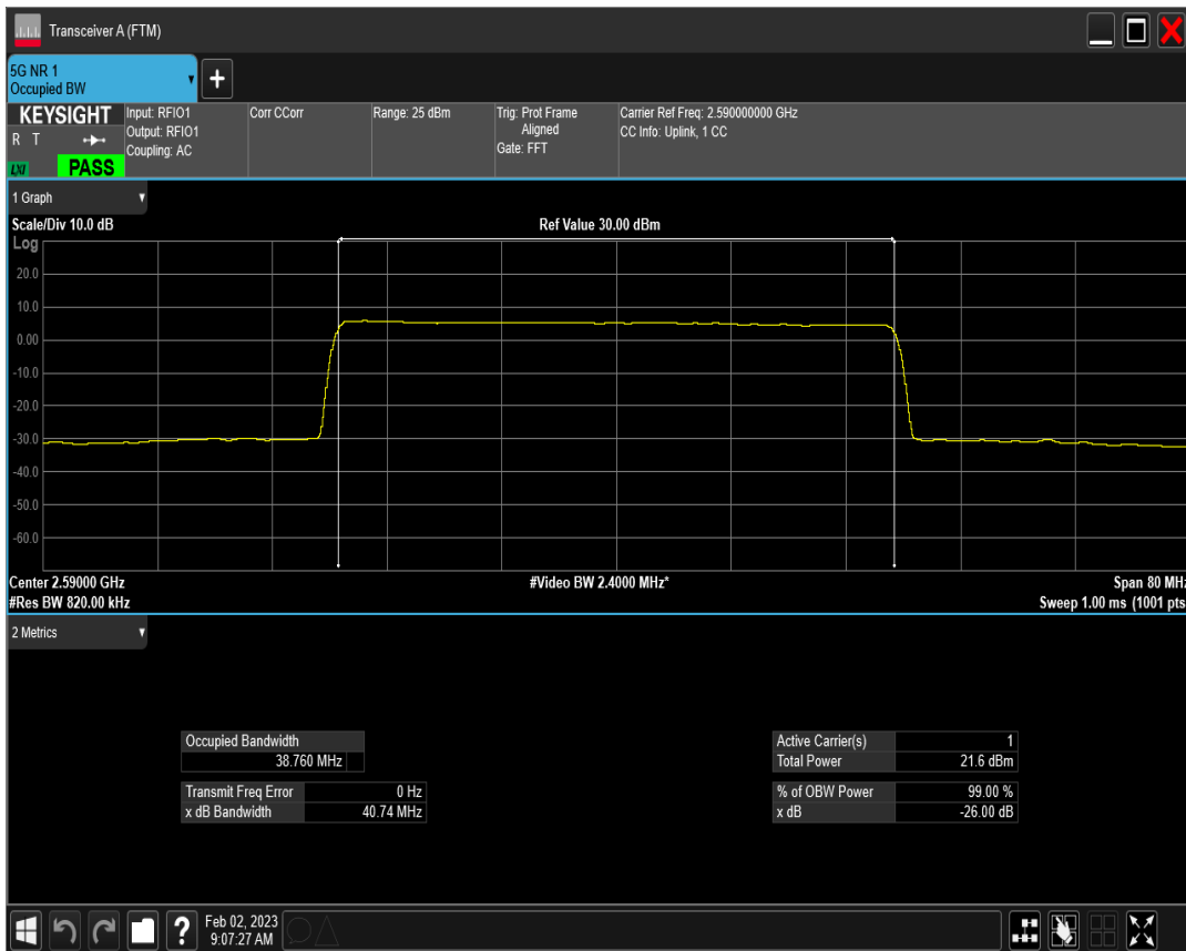
n38 SCS=15kHz DFT_QAM64 BW=40MHz Channel=518000 RB=216@0
