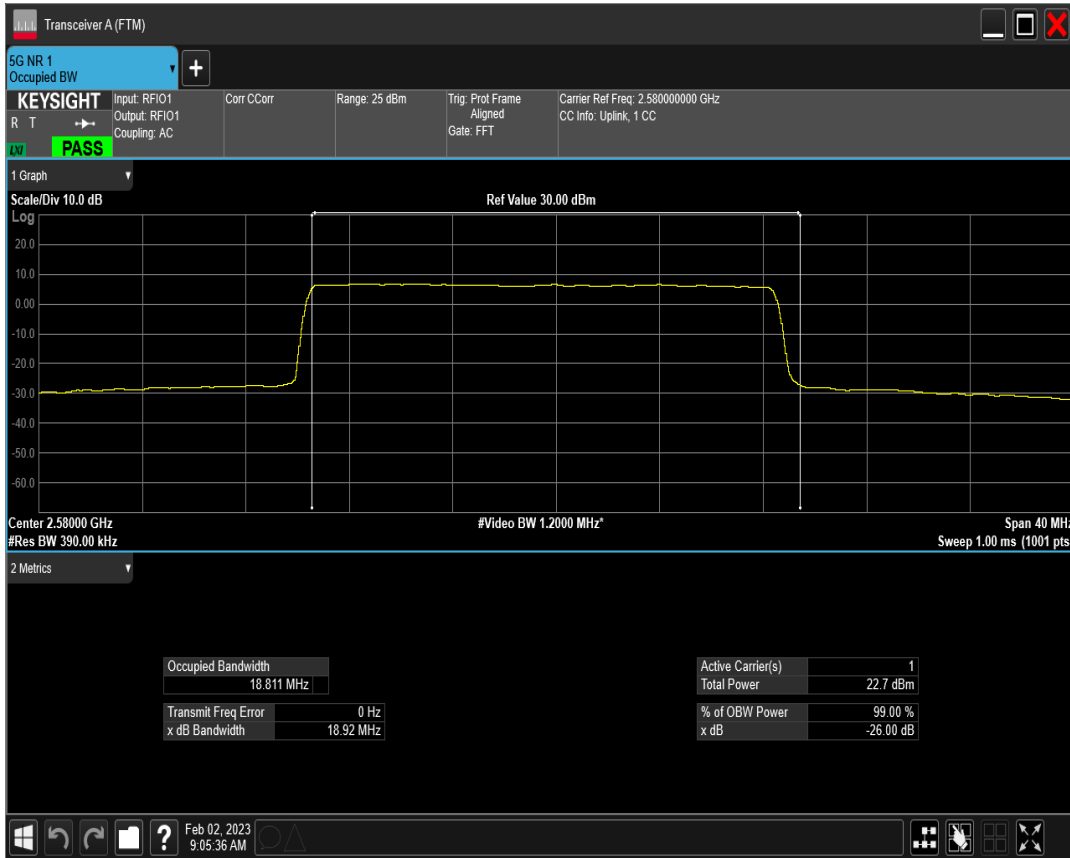
n38 SCS=15kHz DFT_QAM16 BW=20MHz Channel=516000 RB=100@0
