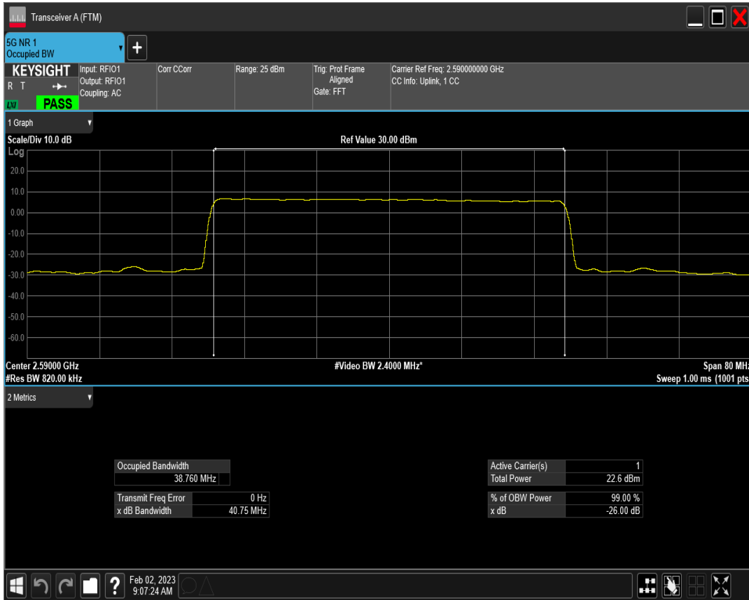
n38 SCS=15kHz DFT_QAM16 BW=40MHz Channel=518000 RB=216@0
