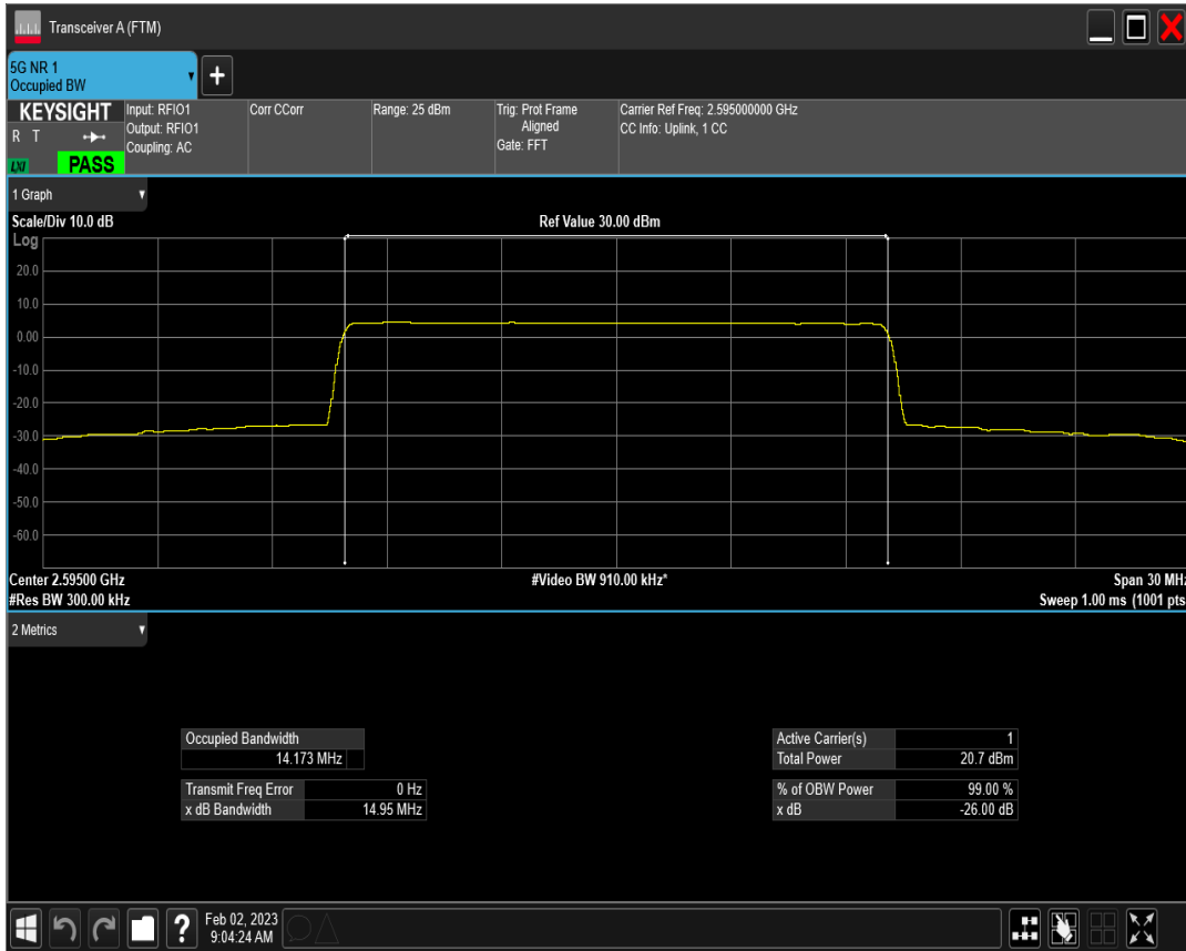
n38 SCS=15kHz DFT_BPSK BW=15MHz Channel=522500 RB=75@0
