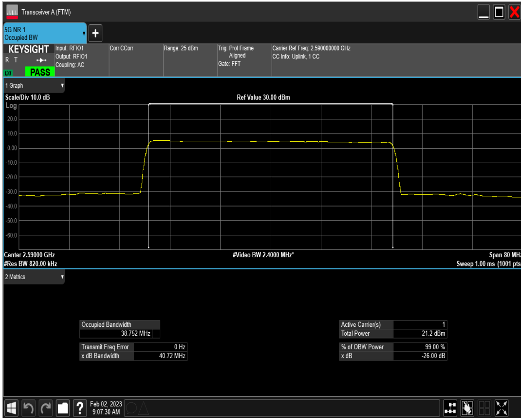
n38 SCS=15kHz DFT_QAM256 BW=40MHz Channel=518000 RB=216@0
