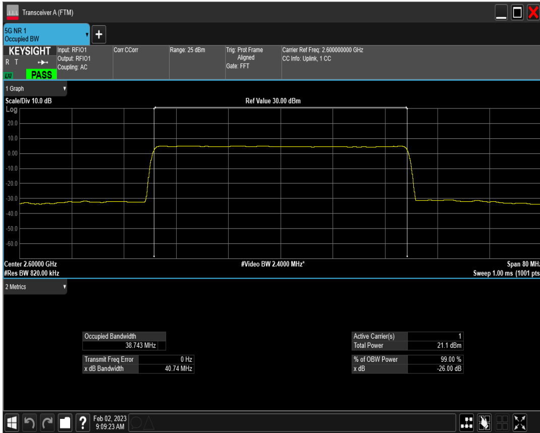
n38 SCS=15kHz DFT_QAM256 BW=40MHz Channel=520000 RB=216@0
