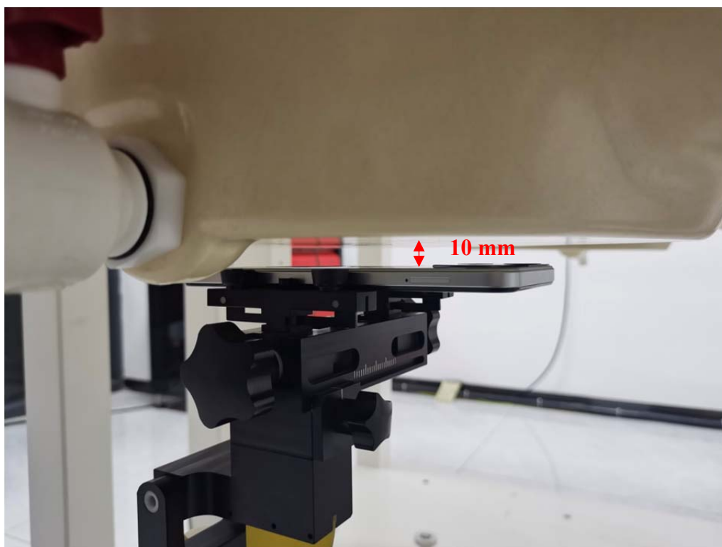
Body (Worn) Back Setup Photo (10mm)
