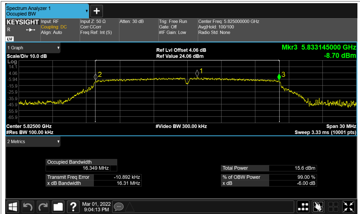
-6dB Bandwidth NVNT ac20 5745MHz Ant1
