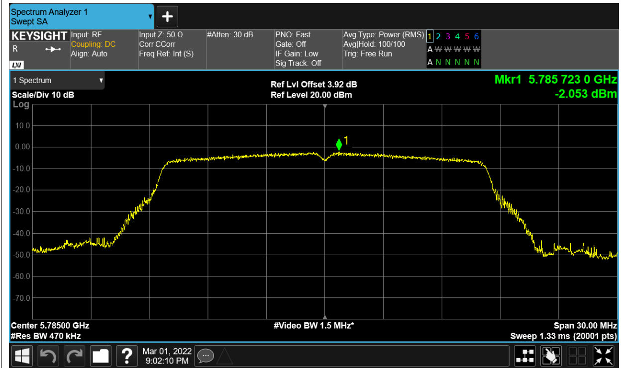
PSD NVNT a 5825MHz Ant1
