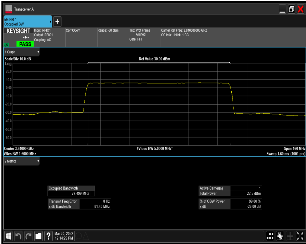
n77(3700-3980) SCS=30kHz DFT_QAM256 BW=80MHz Channel=656000 RB=216@0
