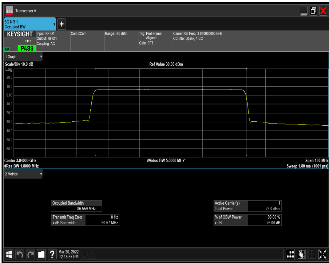
n77(3700-3980) SCS=30kHz DFT_QAM64 BW=90MHz Channel=656000 RB=240@0
