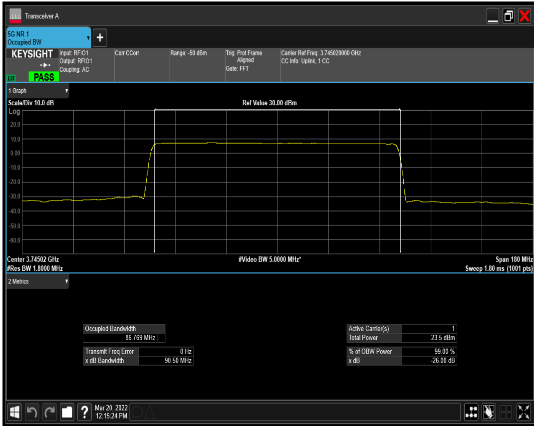
n77(3700-3980) SCS=30kHz DFT_QAM16 BW=90MHz Channel=649668 RB=240@0
