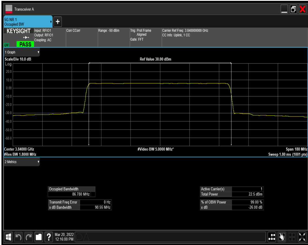
n77(3700-3980) SCS=30kHz DFT_QAM256 BW=90MHz Channel=656000 RB=240@0
