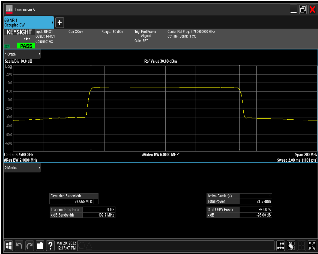
n77(3700-3980) SCS=30kHz DFT_BPSK BW=100MHz Channel=656000 RB=270@0
