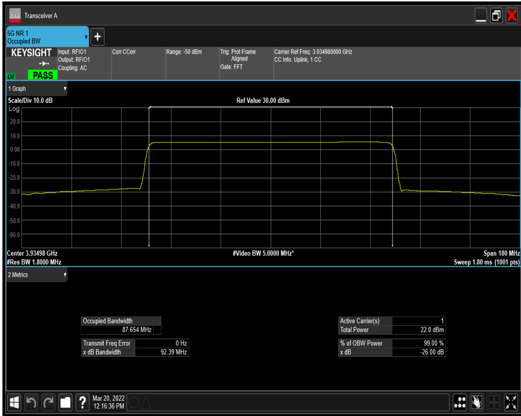
n77(3700-3980) SCS=30kHz DFT_BPSK BW=100MHz Channel=650000 RB=270@0
