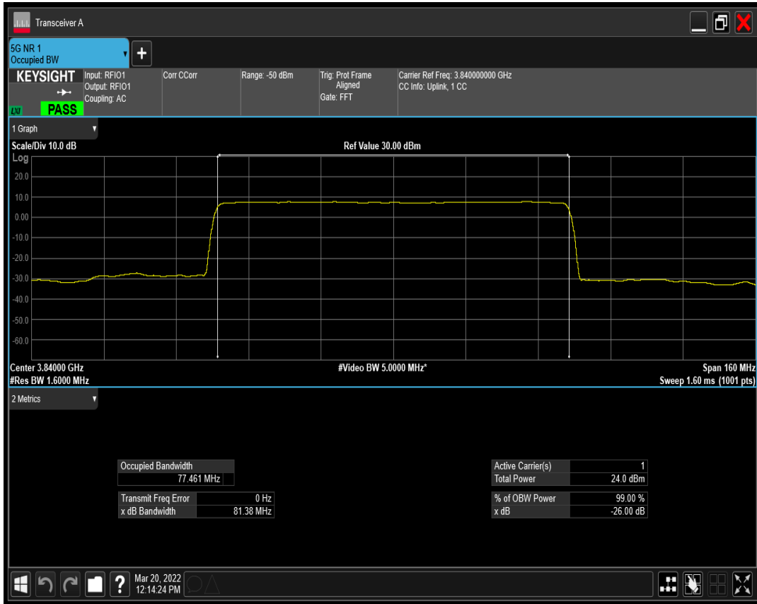
n77(3700-3980) SCS=30kHz DFT_QAM16 BW=80MHz Channel=656000 RB=216@0
