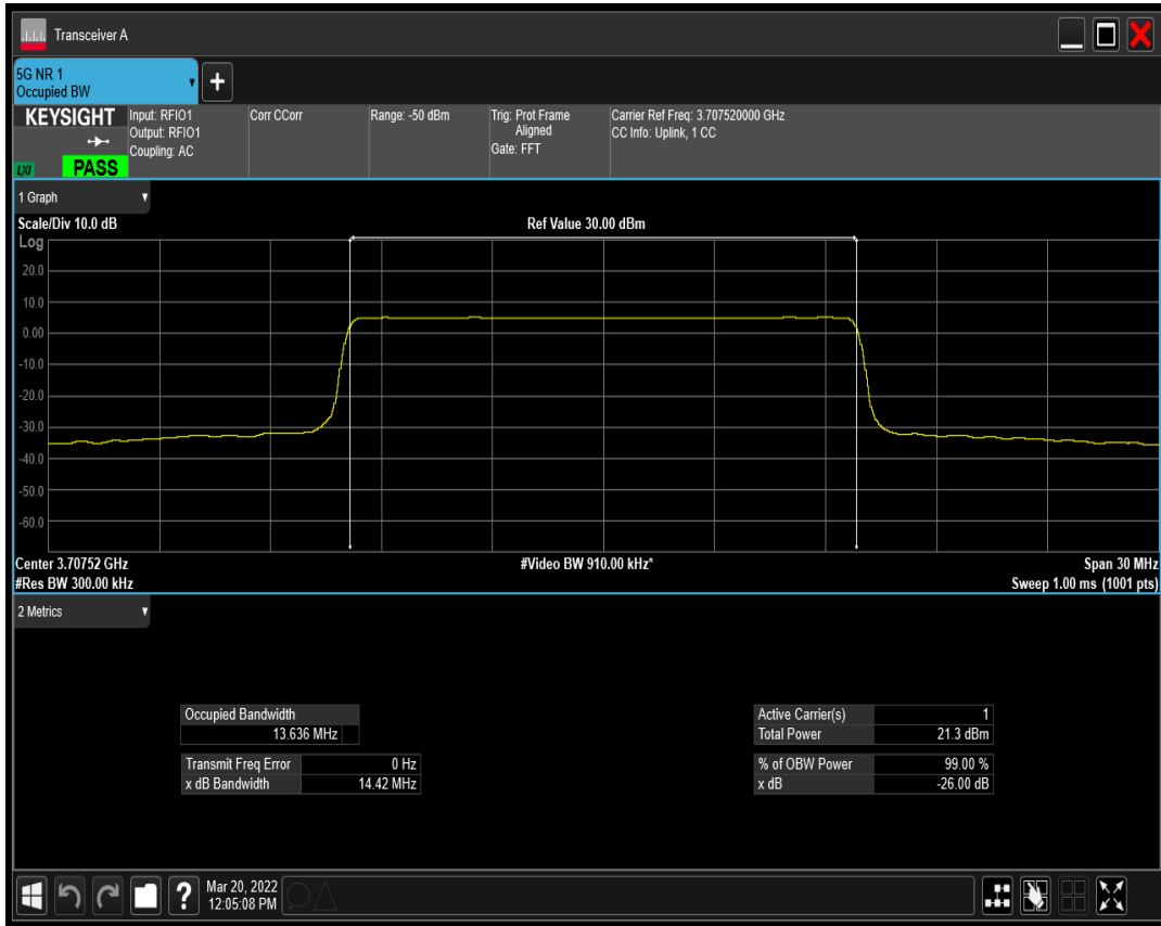
n77(3700-3980) SCS=30kHz DFT_BPSK BW=15MHz Channel=656000 RB=36@0
