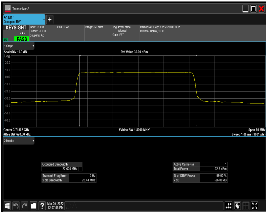
n77(3700-3980) SCS=30kHz DFT_QAM64 BW=30MHz Channel=647668 RB=75@0
