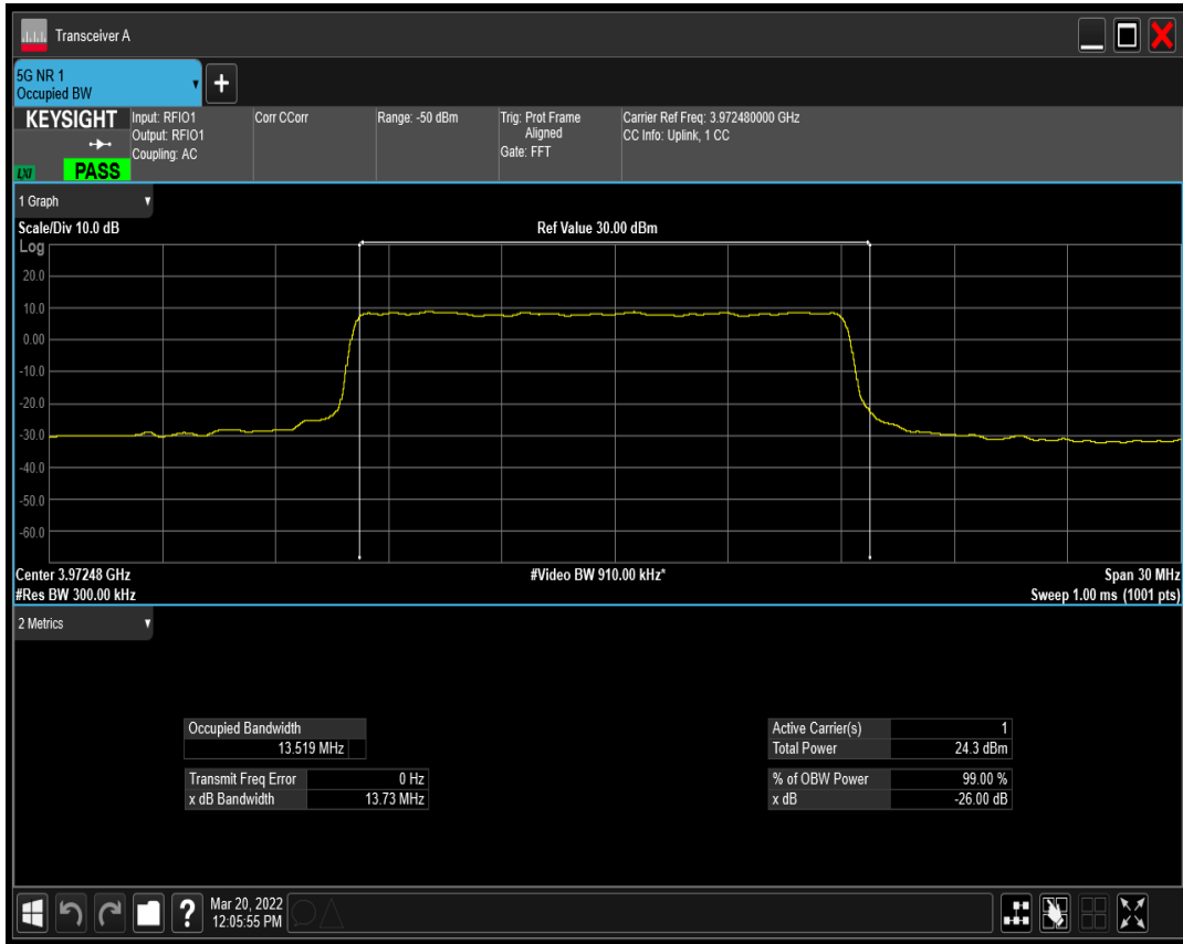
n77(3700-3980) SCS=30kHz DFT_QAM16 BW=15MHz Channel=664832 RB=36@0
