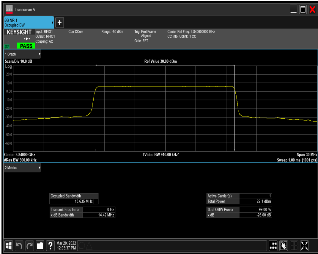
n77(3700-3980) SCS=30kHz DFT_BPSK BW=15MHz Channel=664832 RB=36@0
