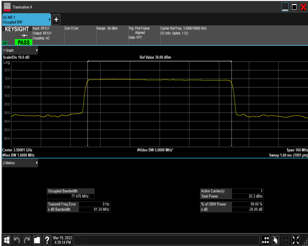
n77(3450-3550) SCS=30kHz DFT_QPSK BW=80MHz Channel=633334 RB=216@0
