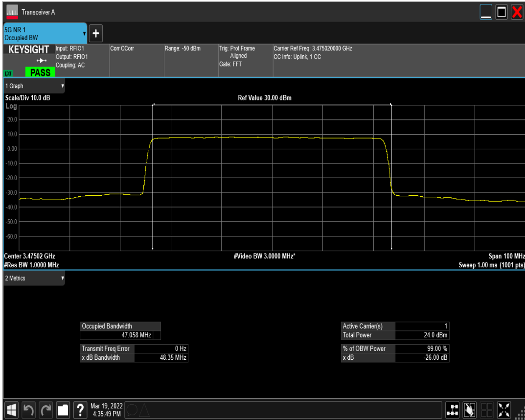
n77(3450-3550) SCS=30kHz DFT_QAM64 BW=50MHz Channel=631668 RB=128@0
