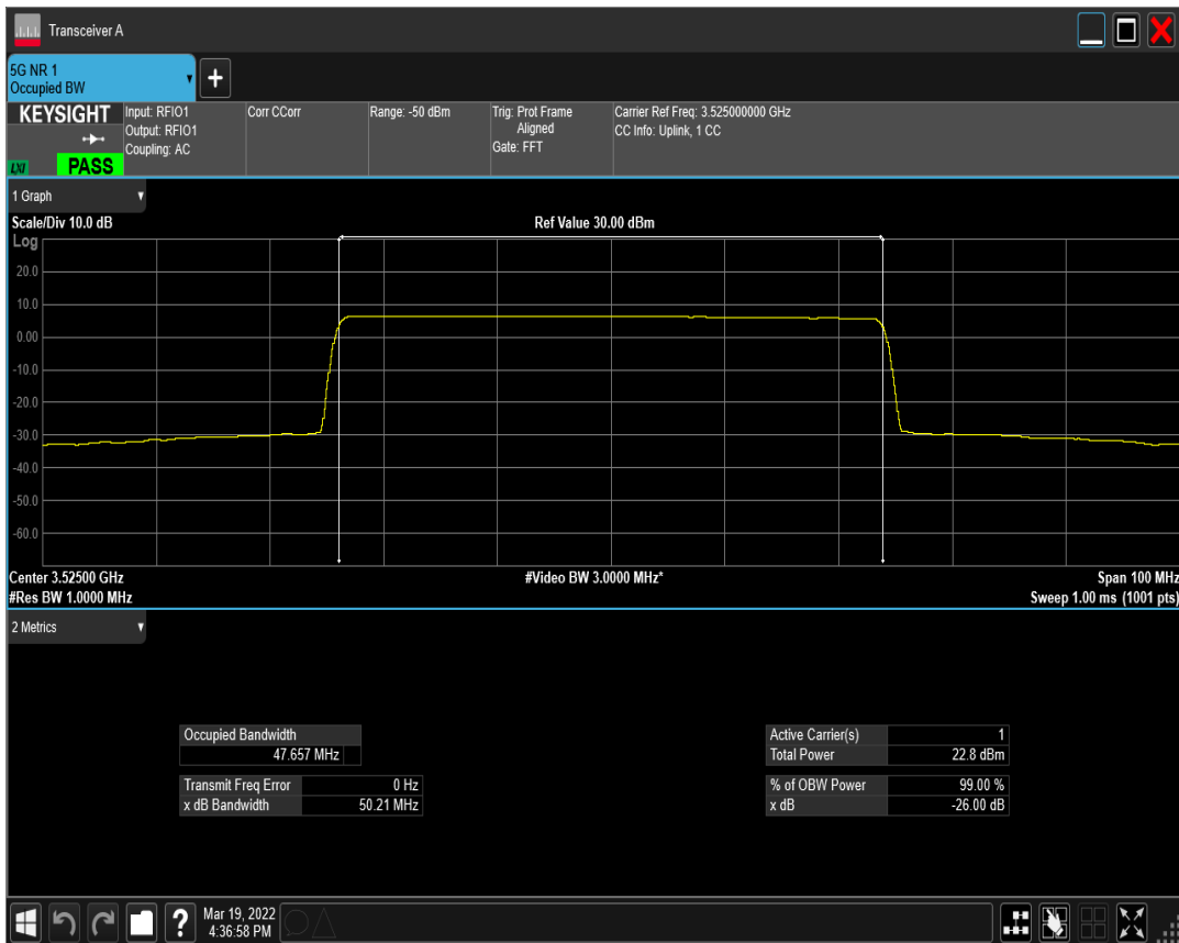
n77(3450-3550) SCS=30kHz DFT_BPSK BW=60MHz Channel=632000 RB=162@0
