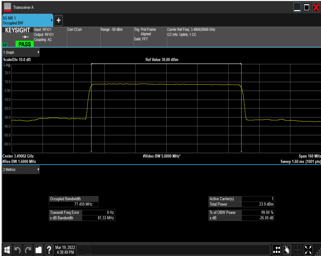
n77(3450-3550) SCS=30kHz DFT_QAM64 BW=80MHz Channel=632668 RB=216@0
