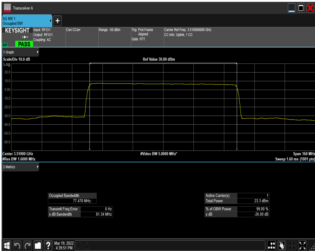
n77(3450-3550) SCS=30kHz DFT_QAM256 BW=80MHz Channel=634000 RB=216@0
