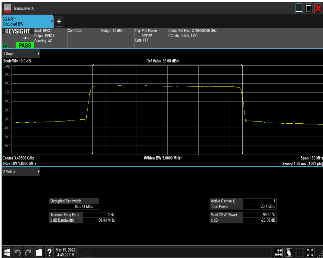
n77(3450-3550) SCS=30kHz DFT_QAM256 BW=90MHz Channel=633000 RB=240@0
