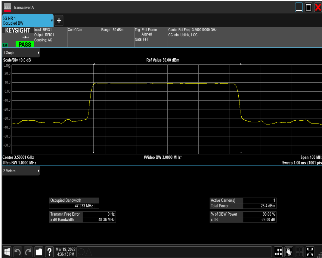
n77(3450-3550) SCS=30kHz DFT_QPSK BW=50MHz Channel=633334 RB=128@0
