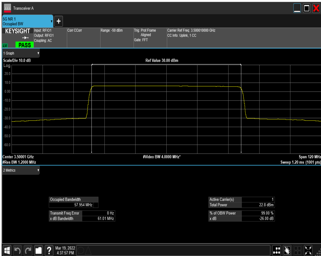
n77(3450-3550) SCS=30kHz DFT_BPSK BW=60MHz Channel=634666 RB=162@0
