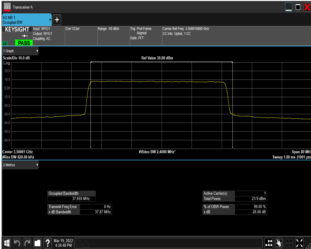
n77(3450-3550) SCS=30kHz DFT_QAM64 BW=40MHz Channel=633334 RB=100@0
