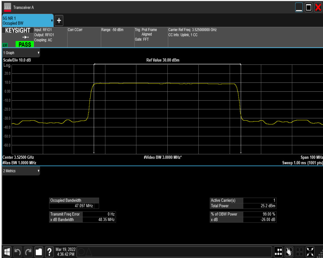
n77(3450-3550) SCS=30kHz DFT_QPSK BW=50MHz Channel=635000 RB=128@0
