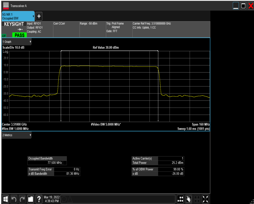
n77(3450-3550) SCS=30kHz DFT_QPSK BW=80MHz Channel=634000 RB=216@0
