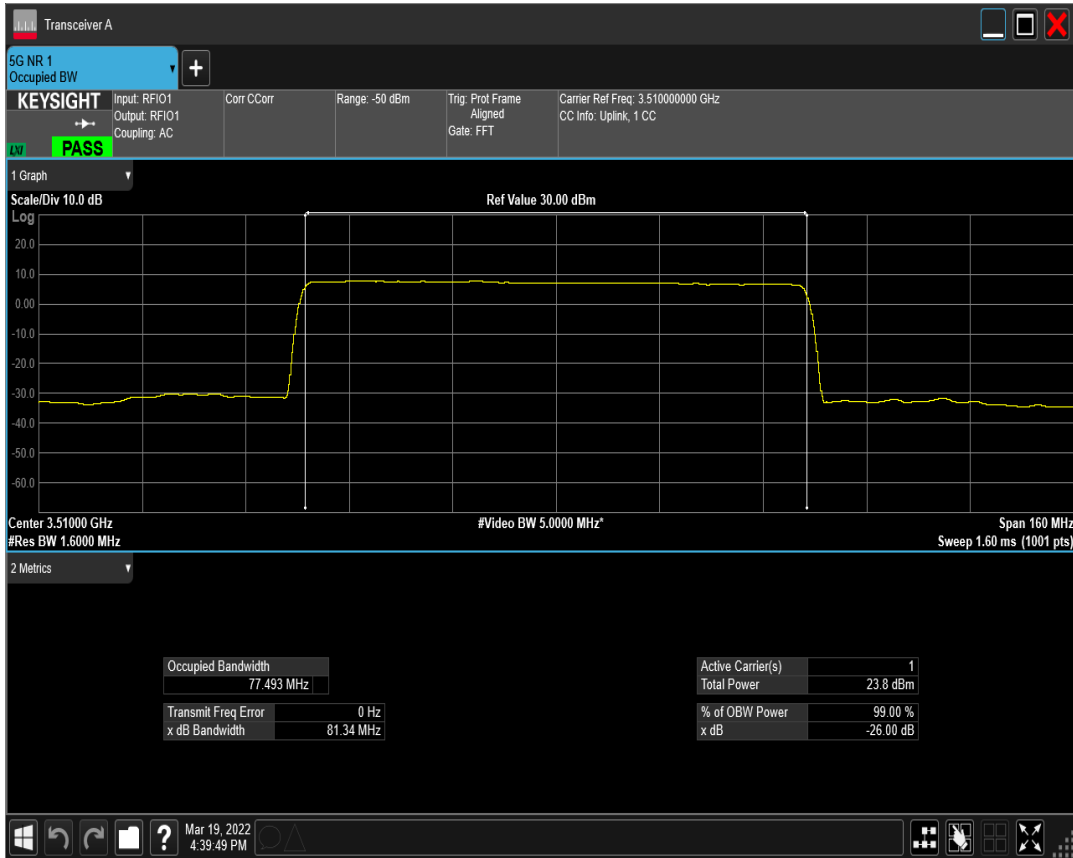
n77(3450-3550) SCS=30kHz DFT_QAM64 BW=80MHz Channel=634000 RB=216@0
