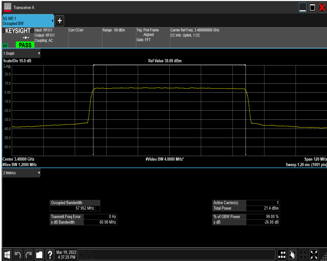
n77(3450-3550) SCS=30kHz CP_QPSK BW=60MHz Channel=632000 RB=162@0
