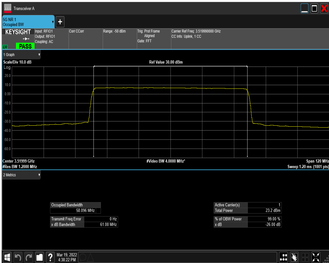
n77(3450-3550) SCS=30kHz DFT_QAM256 BW=60MHz Channel=634666 RB=162@0
