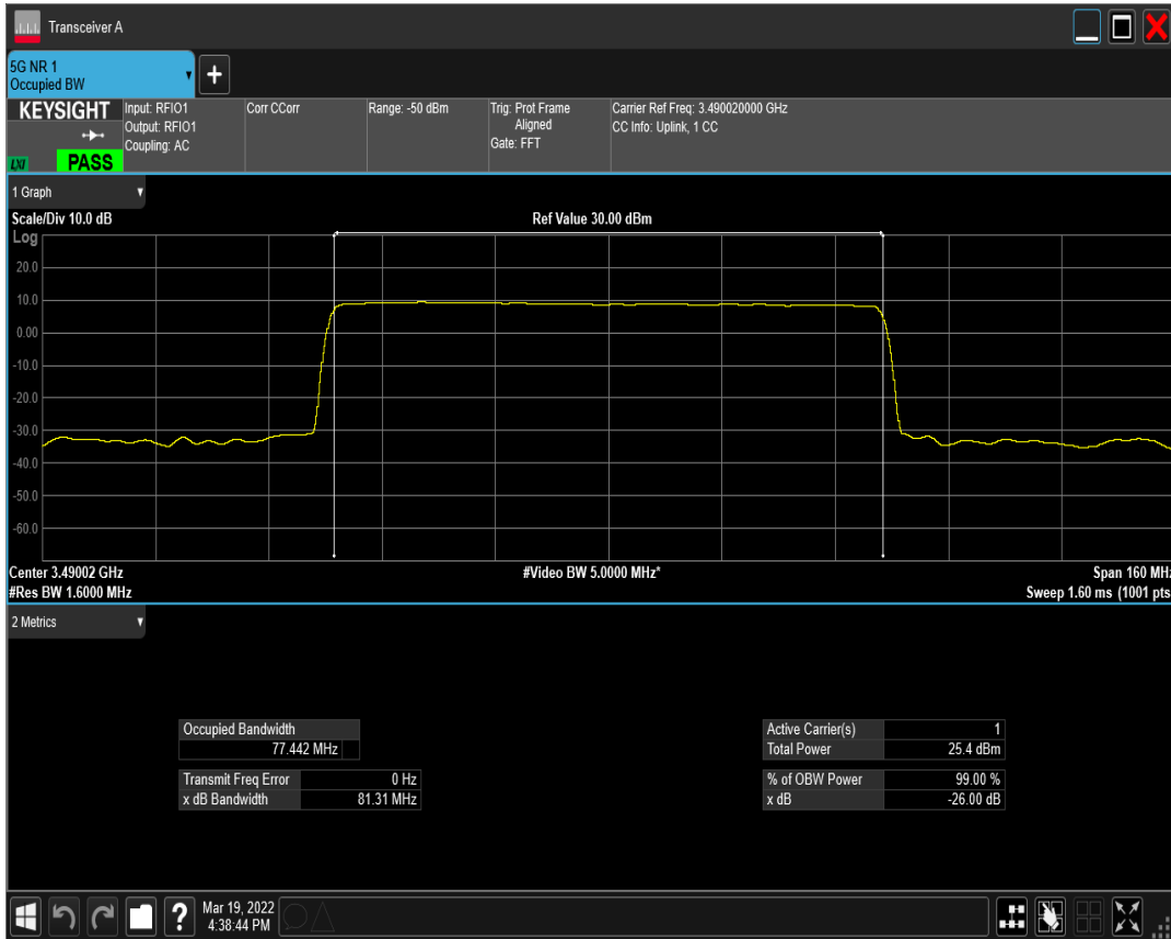
n77(3450-3550) SCS=30kHz DFT_QPSK BW=80MHz Channel=632668 RB=216@0
