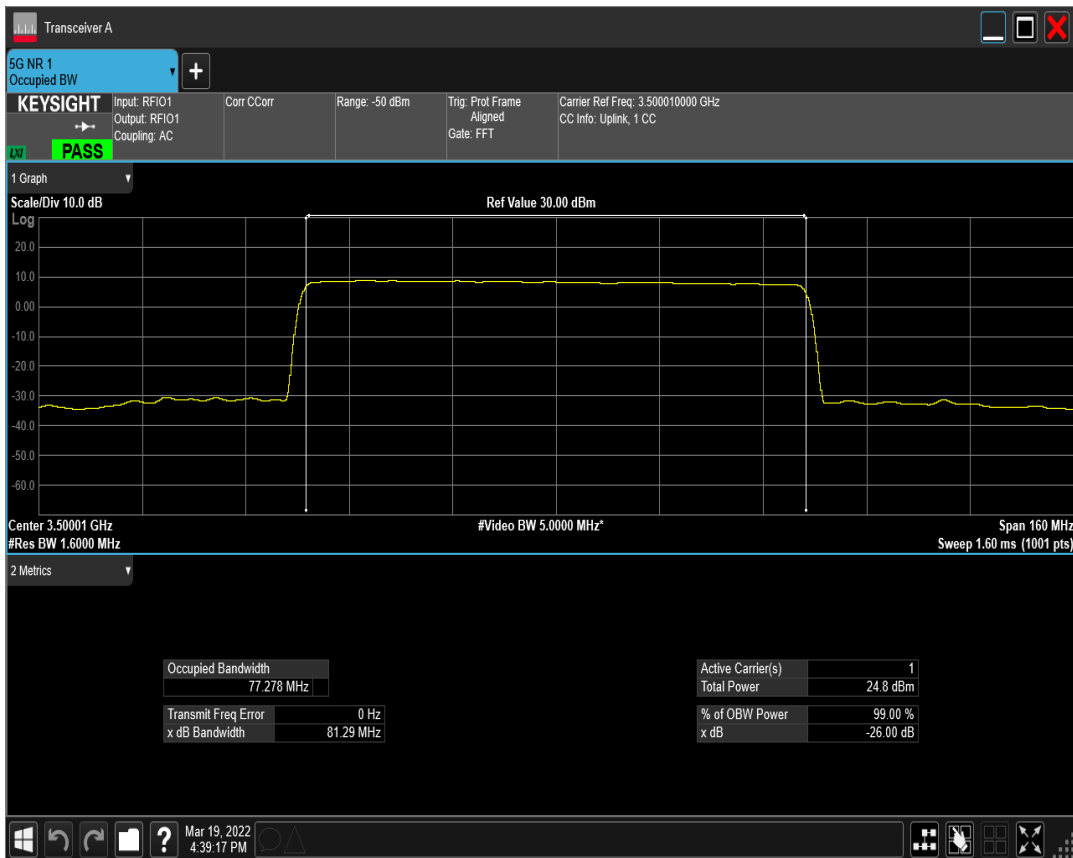
n77(3450-3550) SCS=30kHz DFT_QAM16 BW=80MHz Channel=633334 RB=216@0
