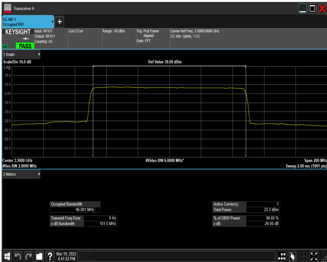
n77(3450-3550) SCS=30kHz DFT_QAM256 BW=100MHz Channel=633334 RB=270@0
