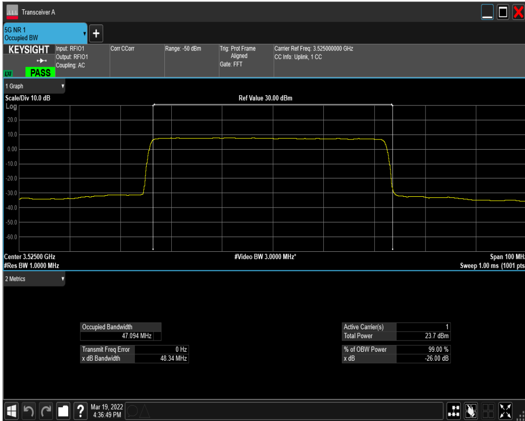
n77(3450-3550) SCS=30kHz DFT_QAM64 BW=50MHz Channel=635000 RB=128@0
