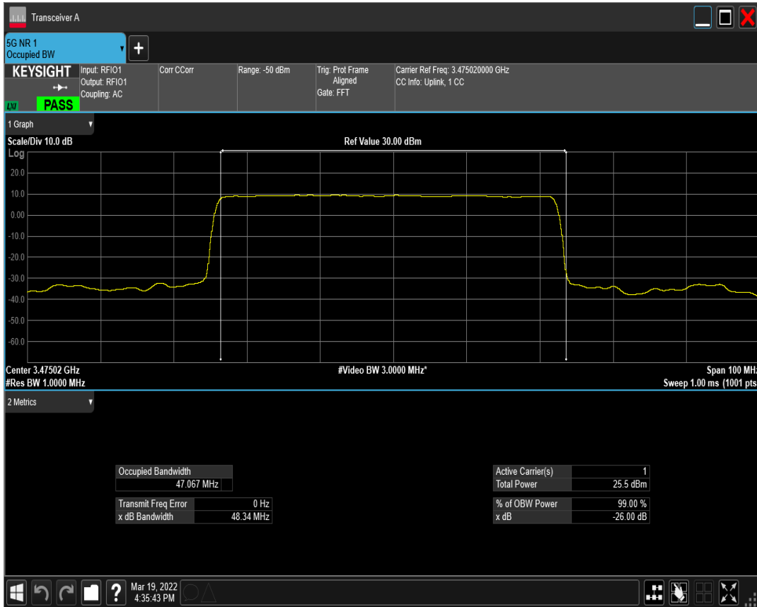
n77(3450-3550) SCS=30kHz DFT_QPSK BW=50MHz Channel=631668 RB=128@0
