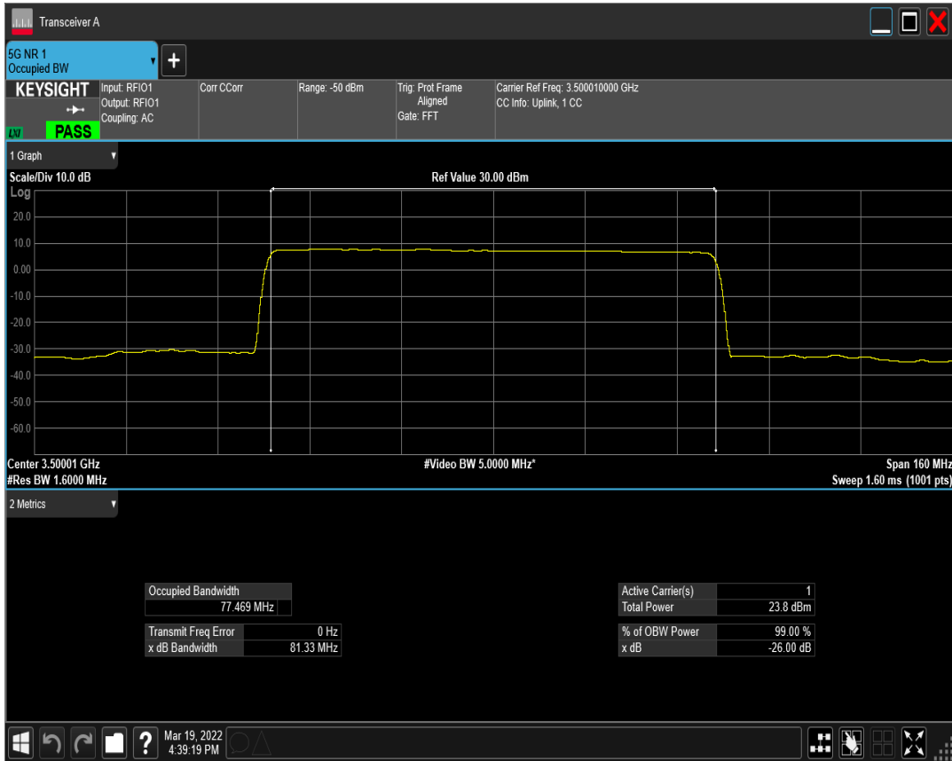
n77(3450-3550) SCS=30kHz DFT_QAM64 BW=80MHz Channel=633334 RB=216@0
