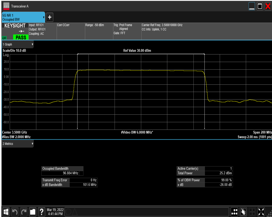
n77(3450-3550) SCS=30kHz DFT_QPSK BW=100MHz Channel=633334 RB=270@0
