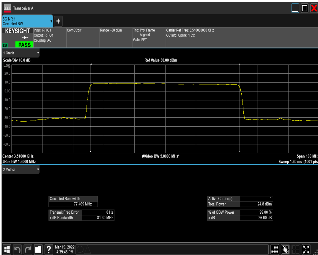
n77(3450-3550) SCS=30kHz DFT_QAM16 BW=80MHz Channel=634000 RB=216@0
