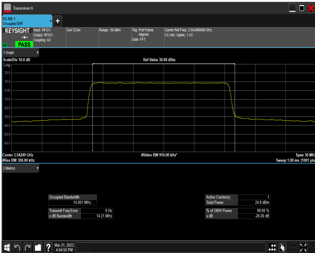
n77(3450-3550) SCS=15kHz DFT_QAM16 BW=15MHz Channel=636166 RB=75@0
