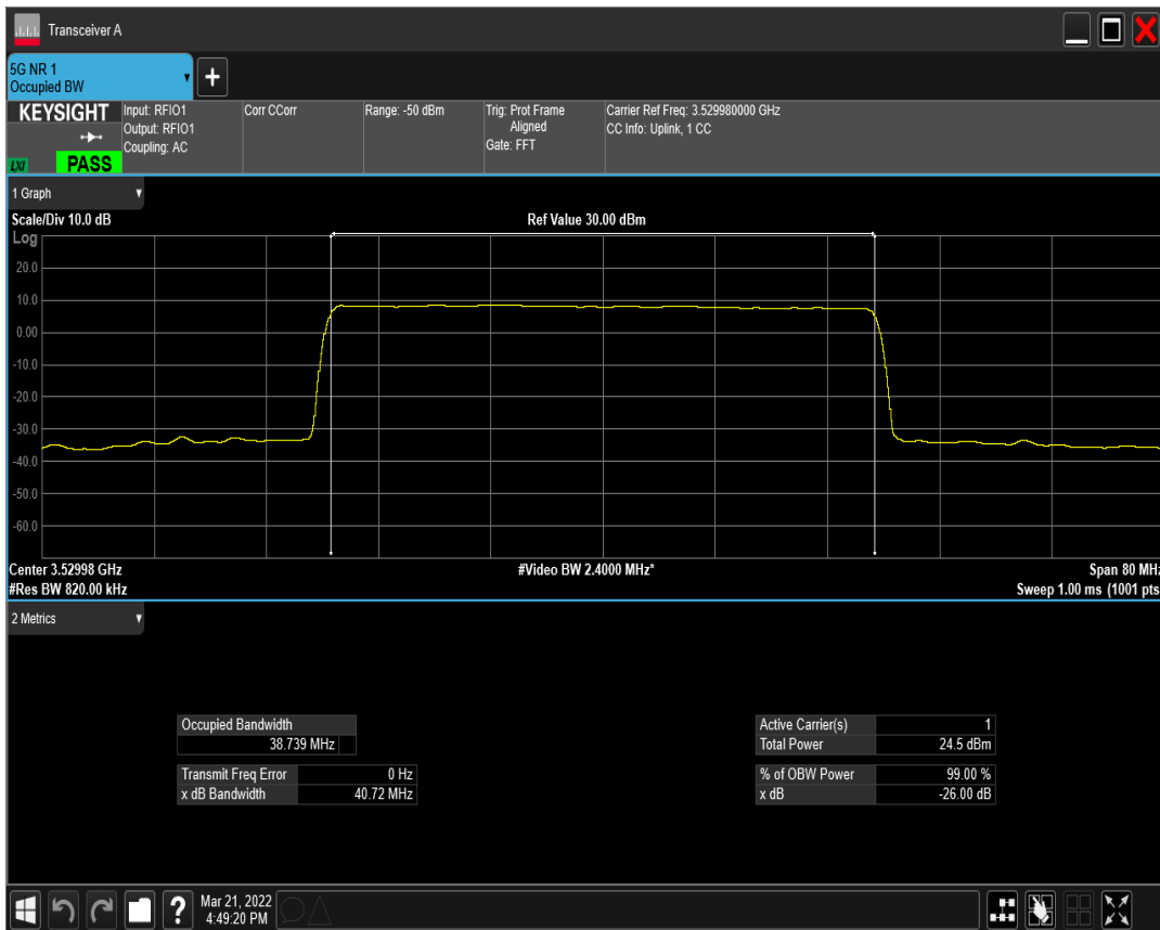
n77(3450-3550) SCS=15kHz DFT_QAM16 BW=40MHz Channel=635332 RB=216@0
