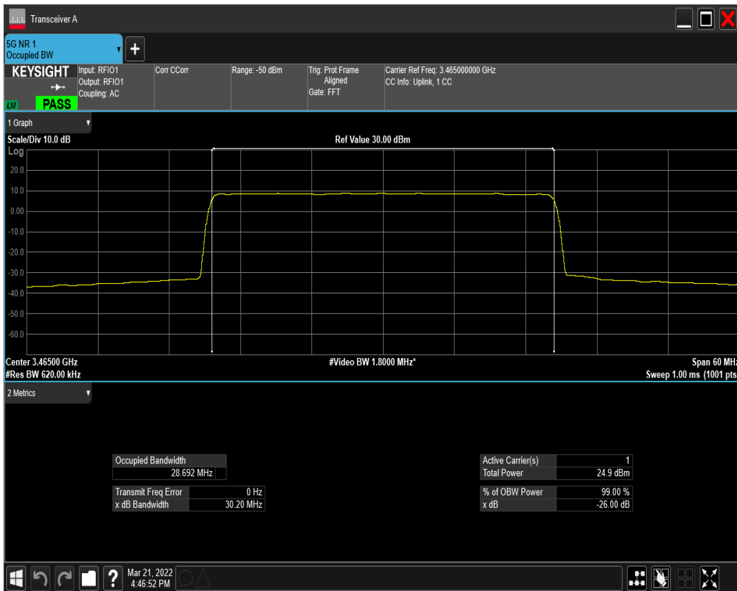
n77(3450-3550) SCS=15kHz DFT_QAM16 BW=30MHz Channel=631000 RB=160@0
