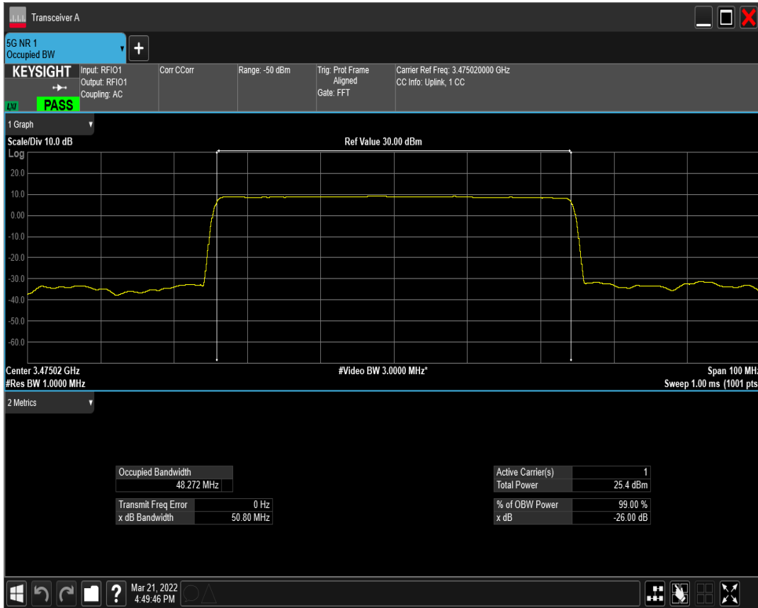
n77(3450-3550) SCS=15kHz DFT_QPSK BW=50MHz Channel=631668 RB=270@0
