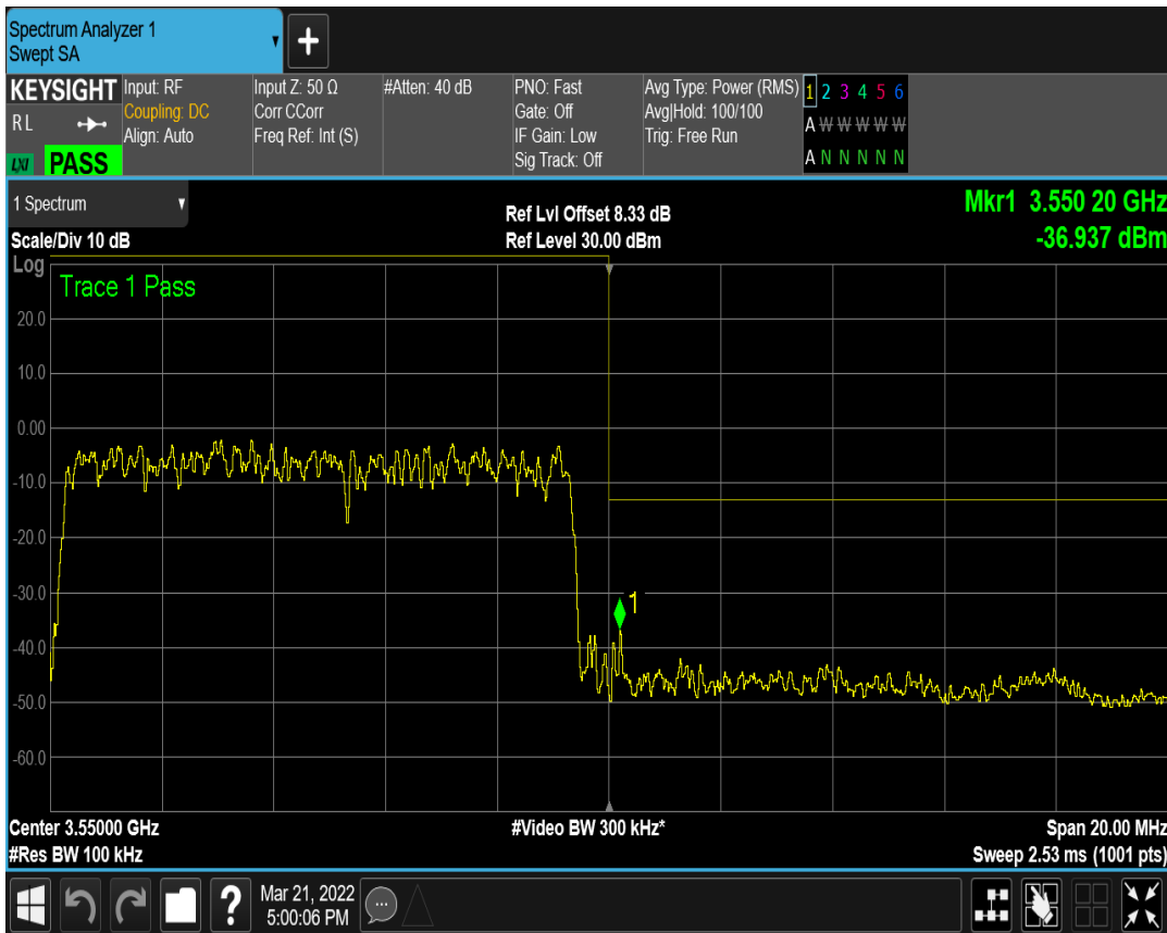
n77(3450-3550) SCS=15kHz DFT_QPSK BW=10MHz Channel=636332 RB=1@51
