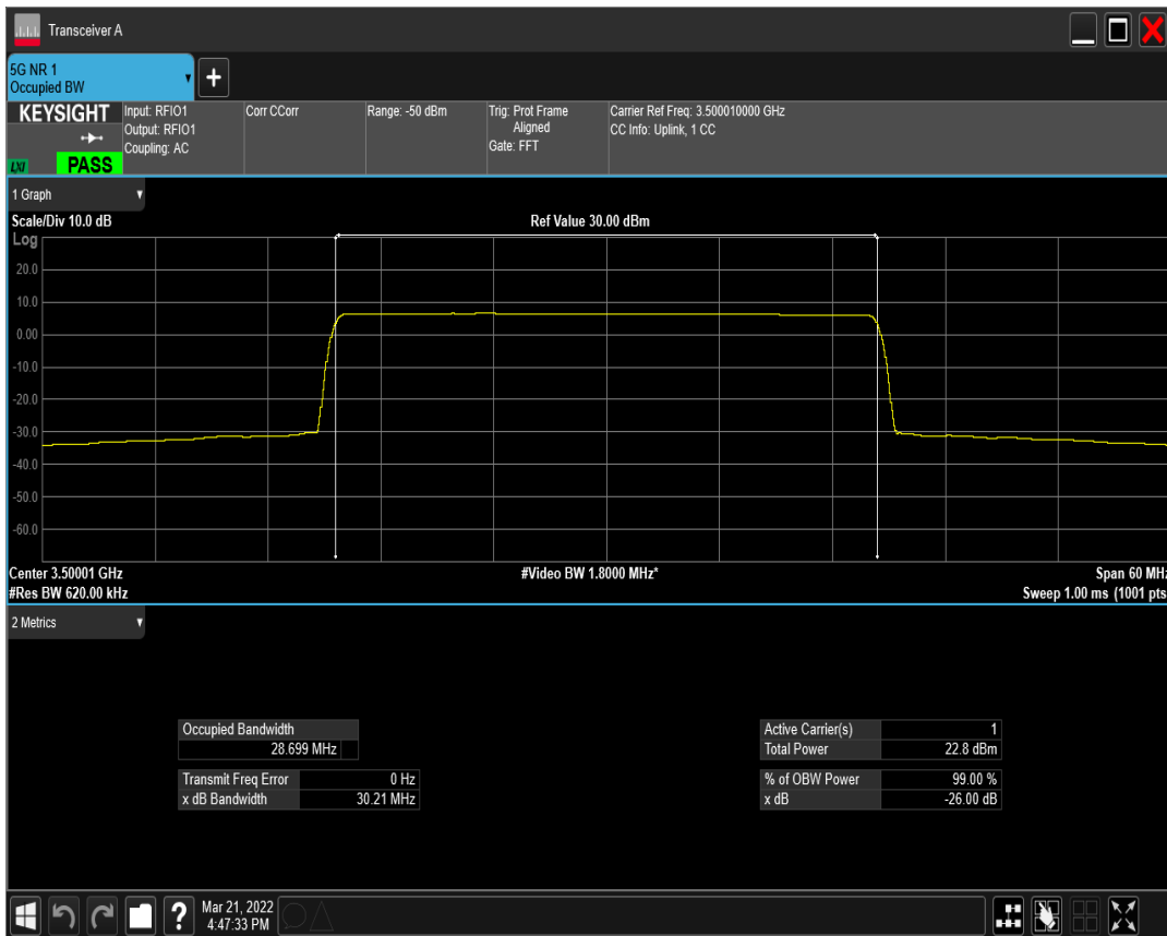
n77(3450-3550) SCS=15kHz DFT_BPSK BW=30MHz Channel=635666 RB=160@0
