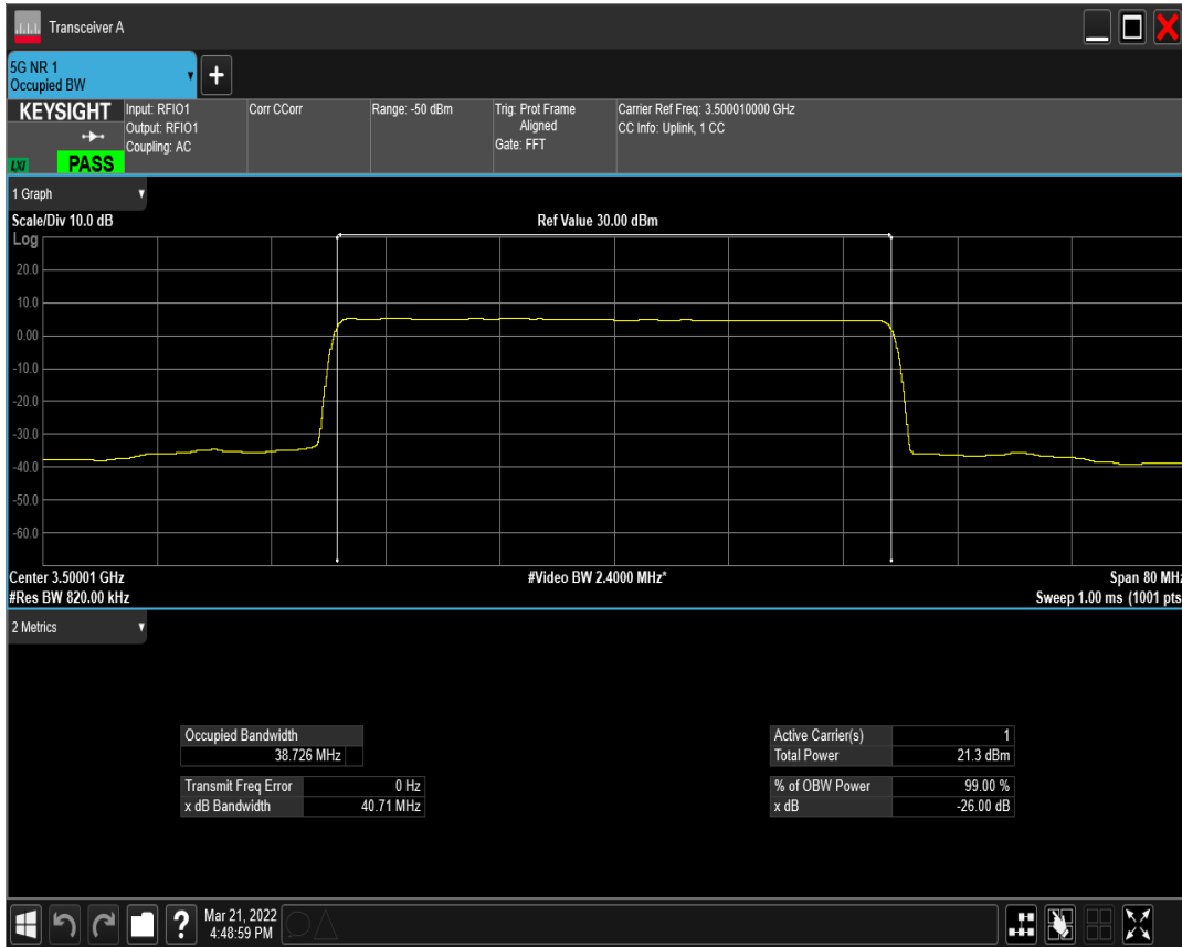
n77(3450-3550) SCS=15kHz CP_QPSK BW=40MHz Channel=633334 RB=216@0
