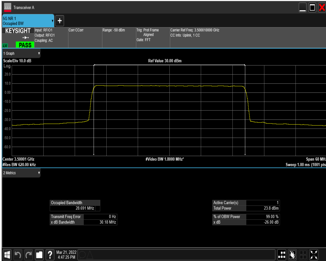
n77(3450-3550) SCS=15kHz DFT_QAM64 BW=30MHz Channel=633334 RB=160@0
