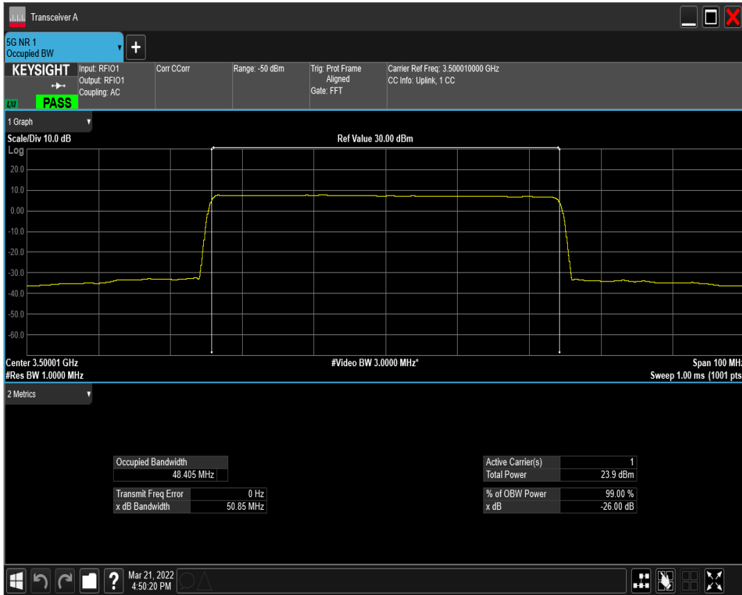
n77(3450-3550) SCS=15kHz DFT_QAM64 BW=50MHz Channel=633334 RB=270@0
