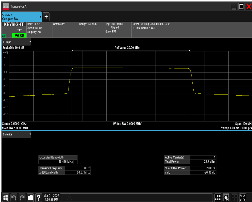
n77(3450-3550) SCS=15kHz DFT_BPSK BW=50MHz Channel=635000 RB=270@0
