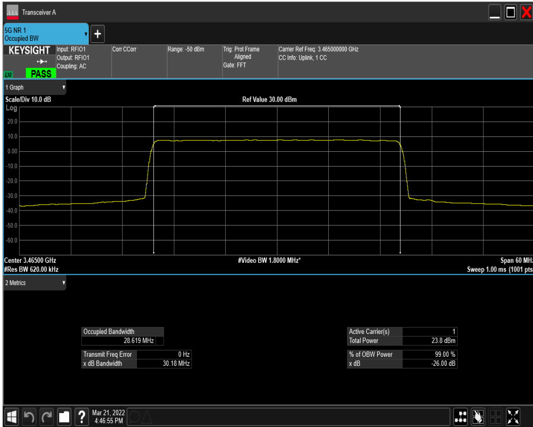
n77(3450-3550) SCS=15kHz DFT_QAM64 BW=30MHz Channel=631000 RB=160@0
