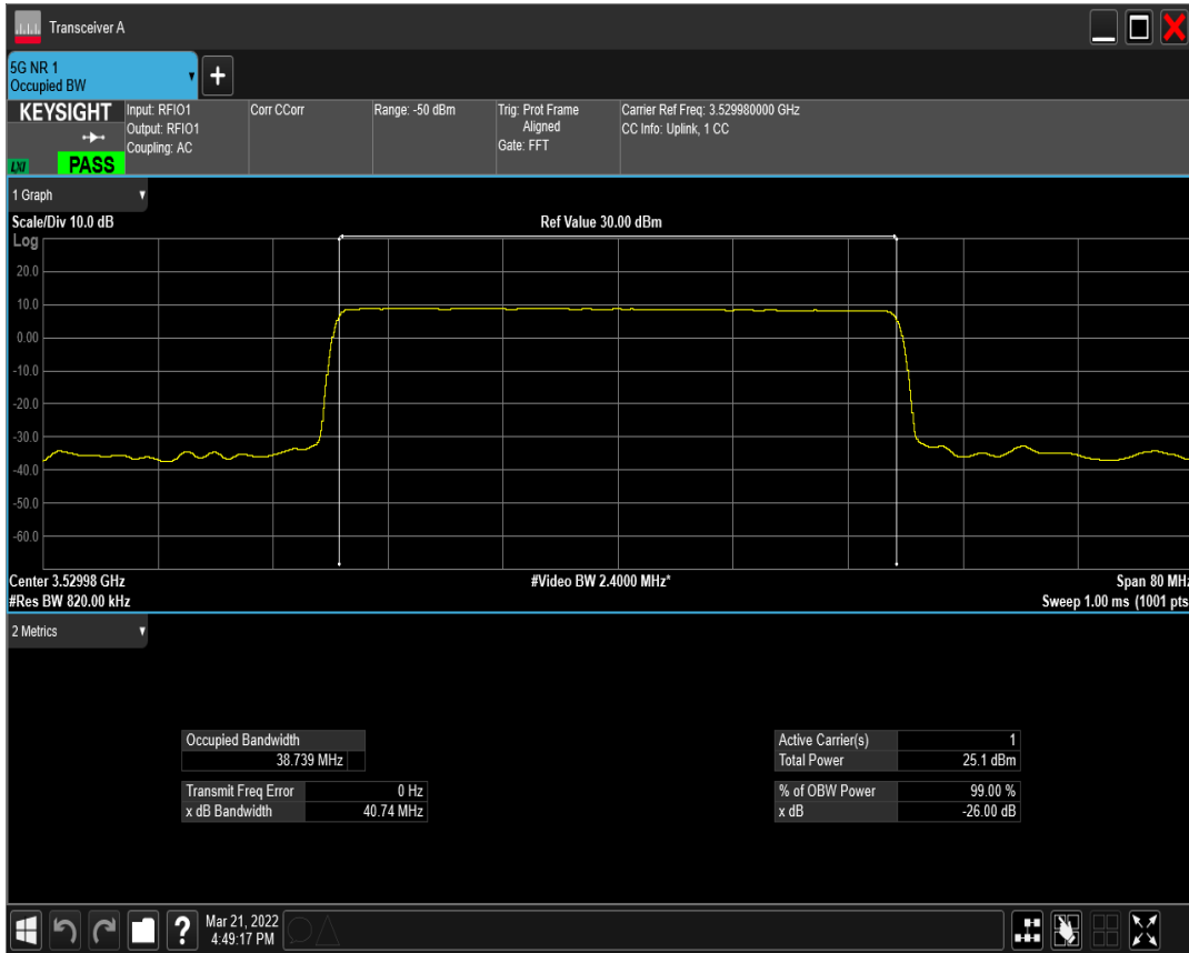
n77(3450-3550) SCS=15kHz DFT_QPSK BW=40MHz Channel=635332 RB=216@0
