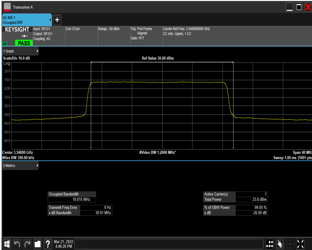
n77(3450-3550) SCS=15kHz DFT_QAM64 BW=20MHz Channel=636000 RB=100@0
