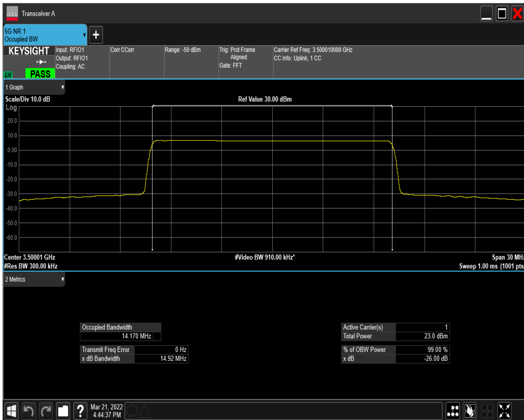
n77(3450-3550) SCS=15kHz DFT_BPSK BW=15MHz Channel=636166 RB=75@0
