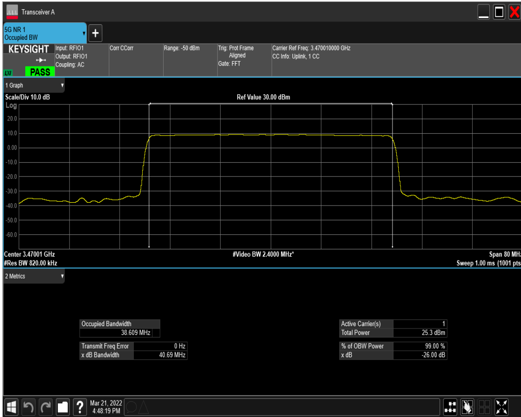
n77(3450-3550) SCS=15kHz DFT_QPSK BW=40MHz Channel=631334 RB=216@0
