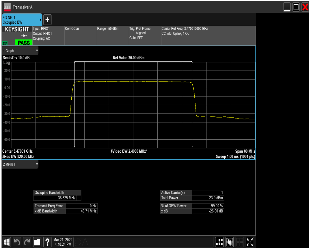
n77(3450-3550) SCS=15kHz DFT_QAM64 BW=40MHz Channel=631334 RB=216@0
