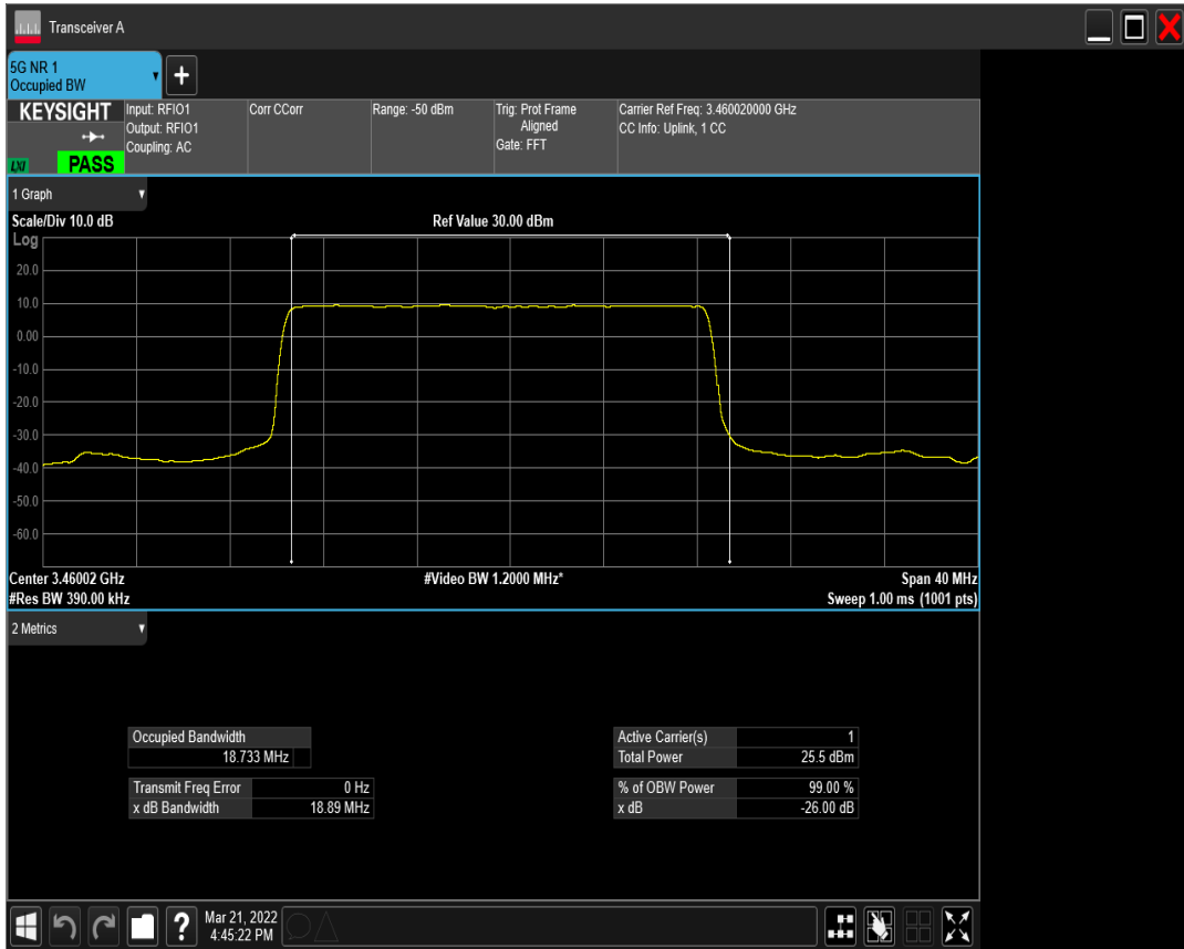
n77(3450-3550) SCS=15kHz DFT_QPSK BW=20MHz Channel=630668 RB=100@0
