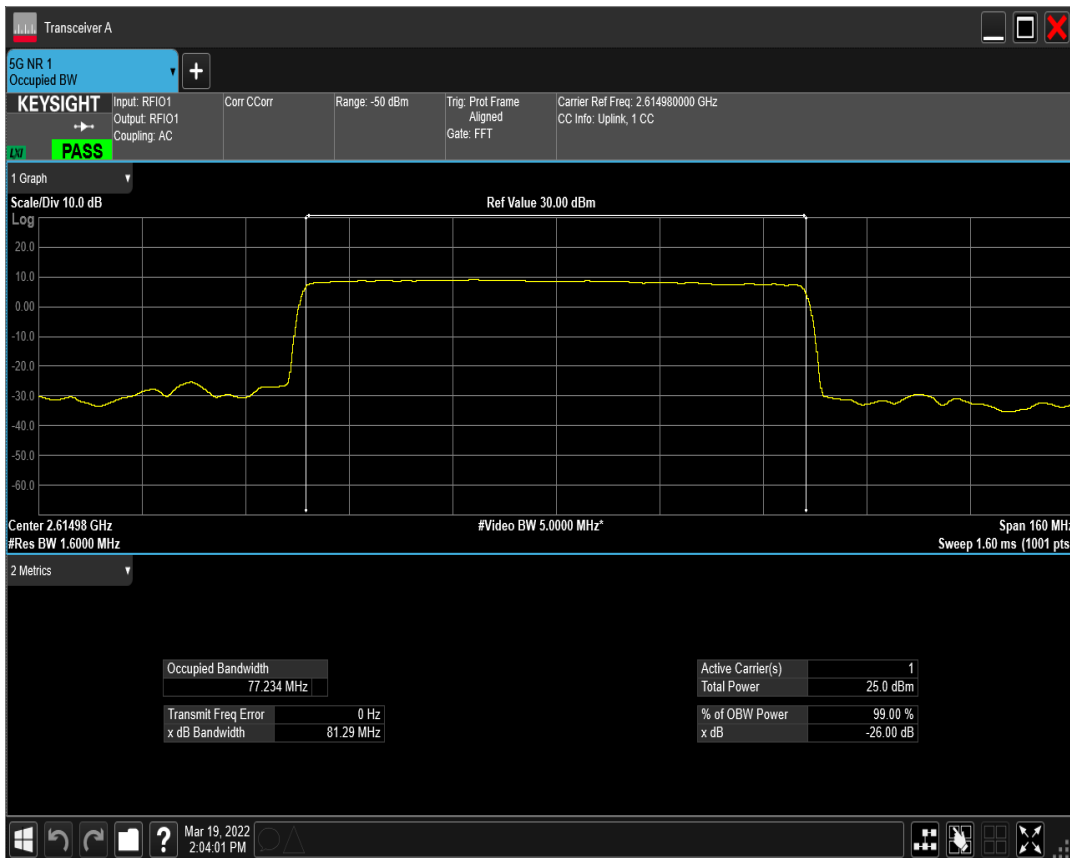
n41(2535-2655) SCS=30kHz DFT_QPSK BW=80MHz Channel=522996 RB=216@0
