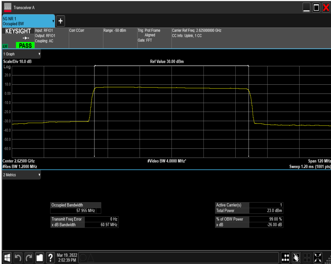
n41(2535-2655) SCS=30kHz DFT_QAM256 BW=60MHz Channel=525000 RB=162@0
