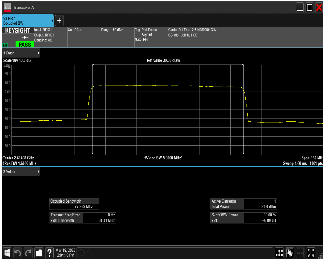
n41(2535-2655) SCS=30kHz DFT_QAM256 BW=80MHz Channel=522996 RB=216@0
