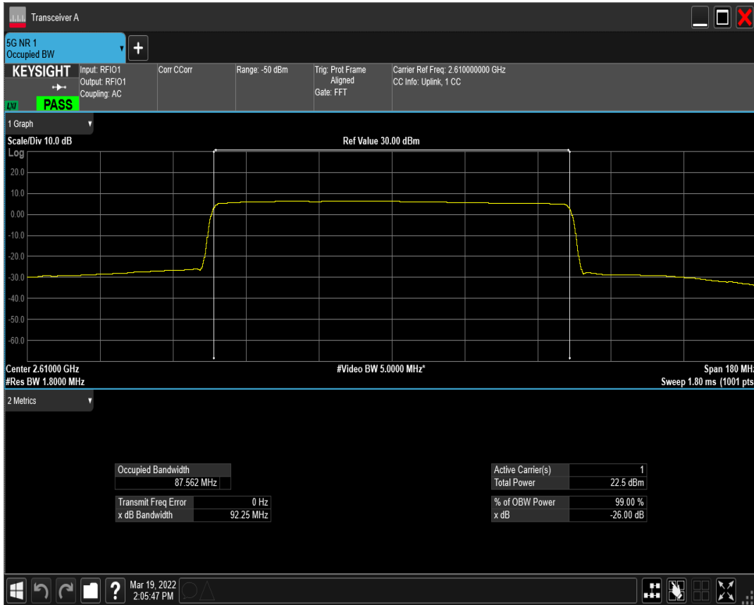
n41(2535-2655) SCS=30kHz DFT_BPSK BW=100MHz Channel=517002 RB=270@0
