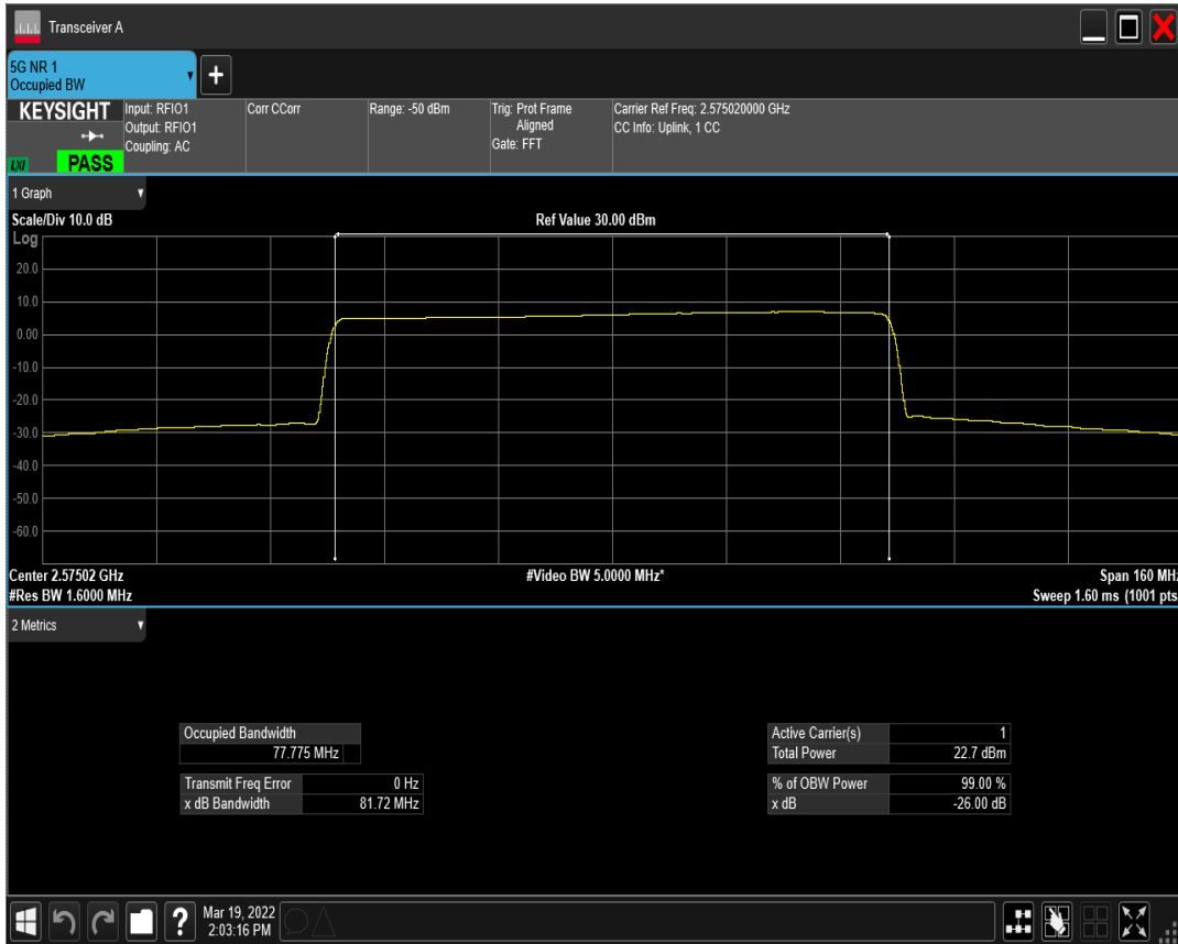
n41(2535-2655) SCS=30kHz DFT_BPSK BW=80MHz Channel=519000 RB=216@0
