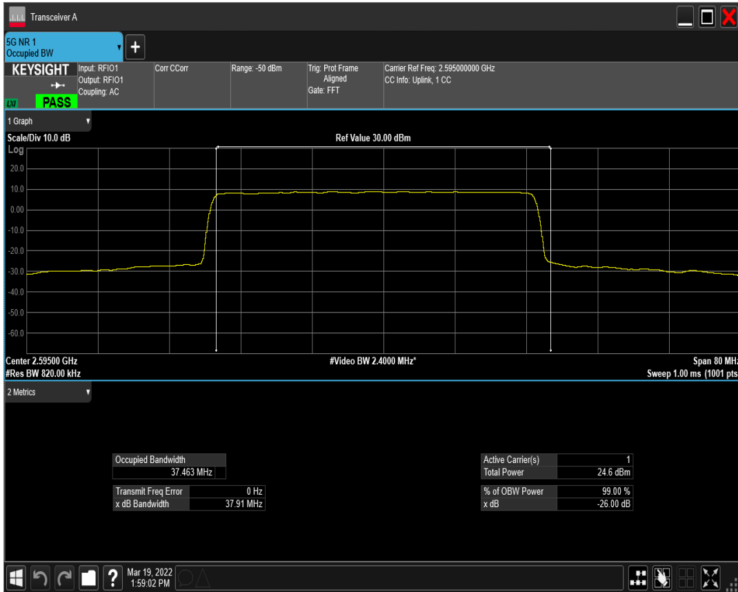
n41(2535-2655) SCS=30kHz DFT_QAM16 BW=40MHz Channel=519000 RB=100@0
