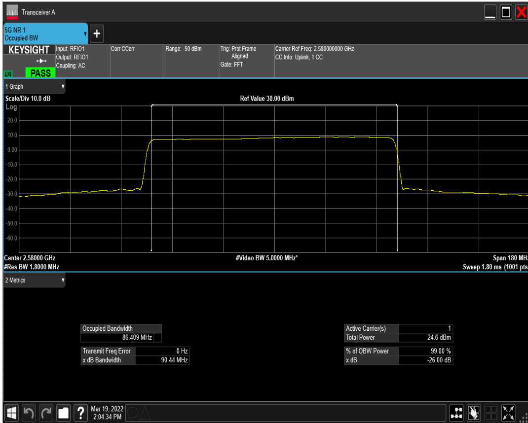
n41(2535-2655) SCS=30kHz DFT_QAM16 BW=90MHz Channel=516000 RB=240@0
