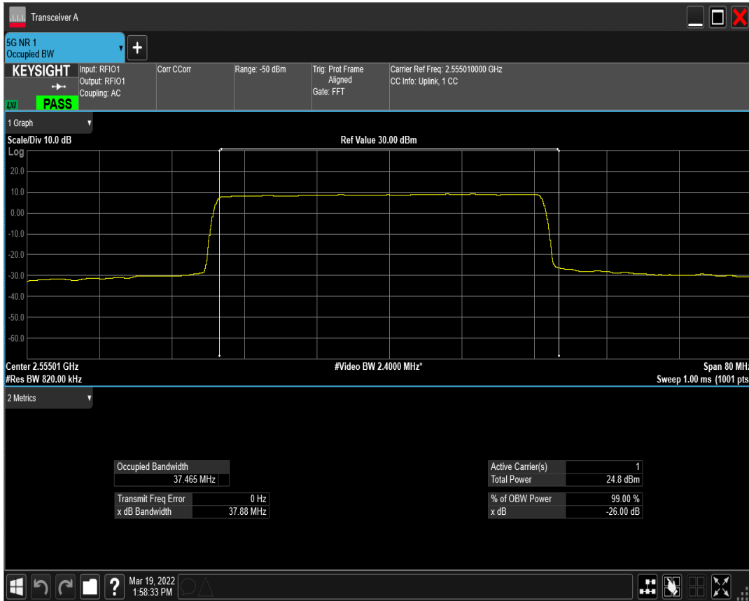
n41(2535-2655) SCS=30kHz DFT_QAM16 BW=40MHz Channel=511002 RB=100@0
