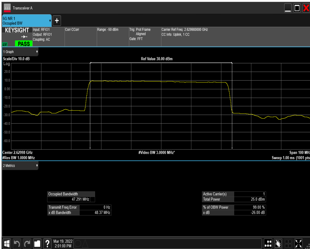
n41(2535-2655) SCS=30kHz DFT_QPSK BW=50MHz Channel=525996 RB=128@0
