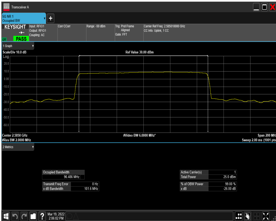
n41(2535-2655) SCS=30kHz DFT_QPSK BW=100MHz Channel=517002 RB=270@0
