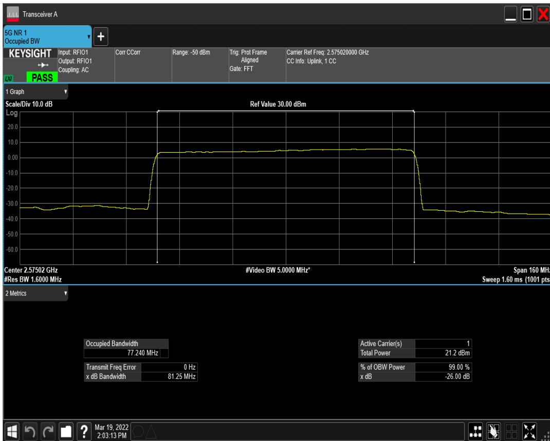
n41(2535-2655) SCS=30kHz CP_QPSK BW=80MHz Channel=515004 RB=217@0
