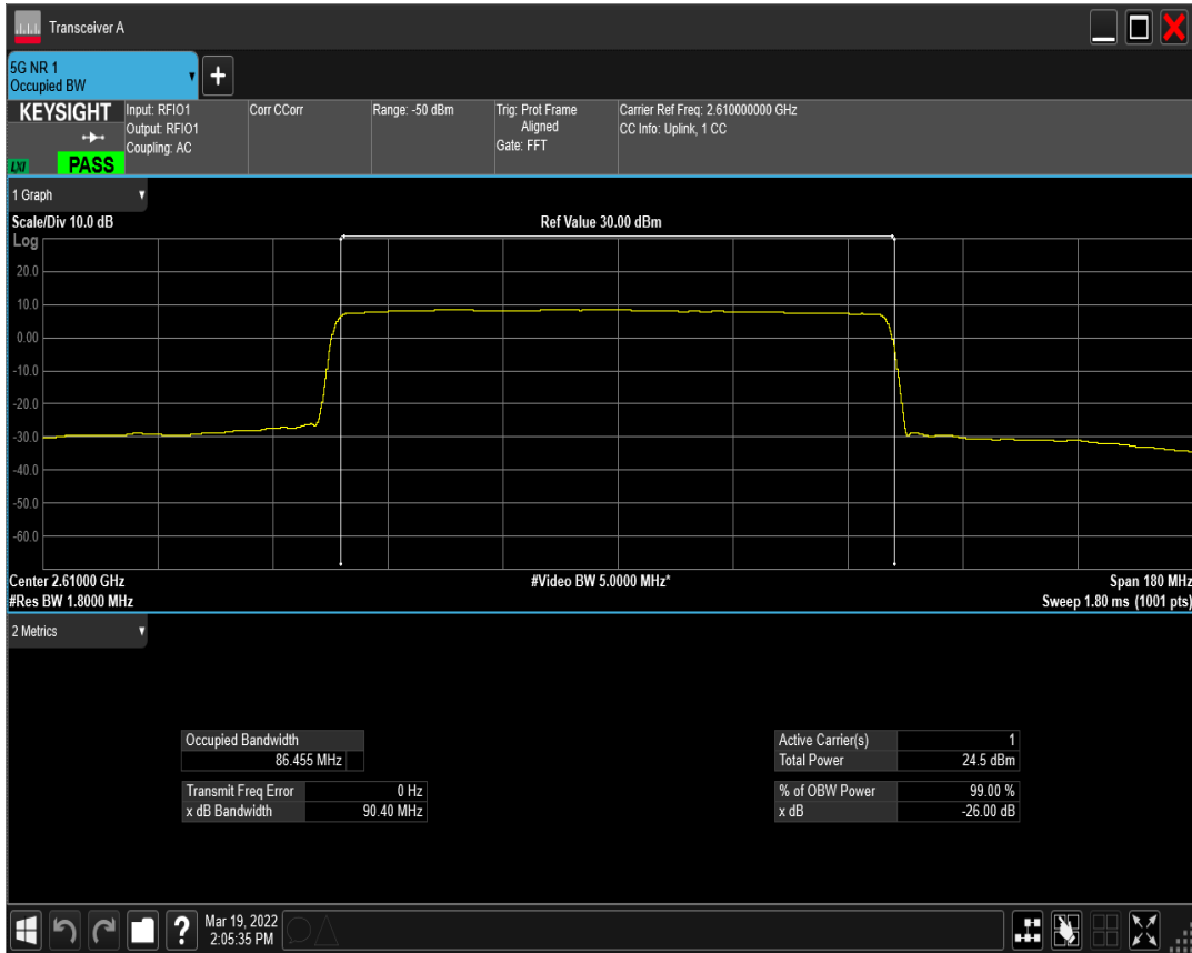
n41(2535-2655) SCS=30kHz DFT_QAM16 BW=90MHz Channel=522000 RB=240@0
