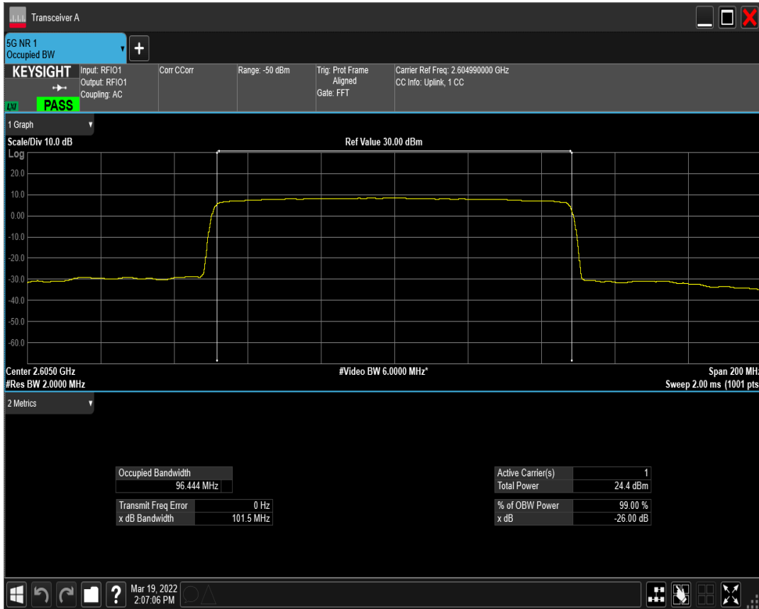
n41(2535-2655) SCS=30kHz DFT_QAM16 BW=100MHz Channel=520998 RB=270@0
