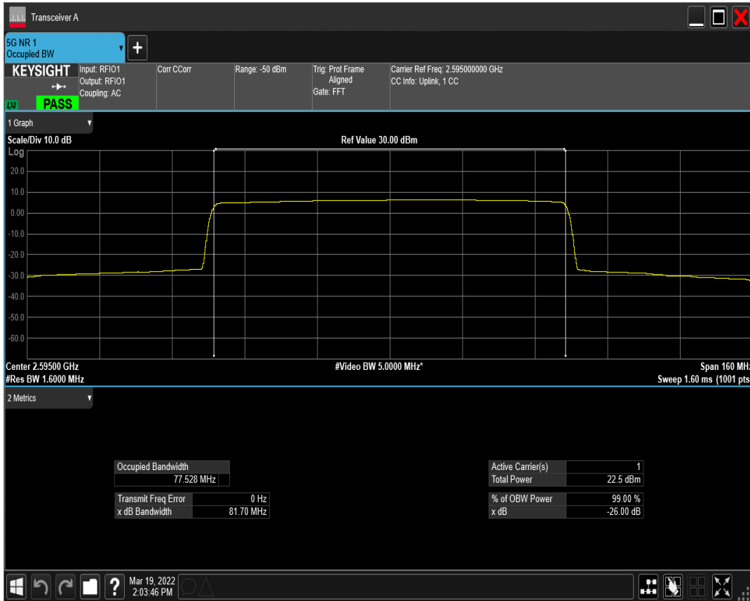
n41(2535-2655) SCS=30kHz DFT_BPSK BW=80MHz Channel=522996 RB=216@0
