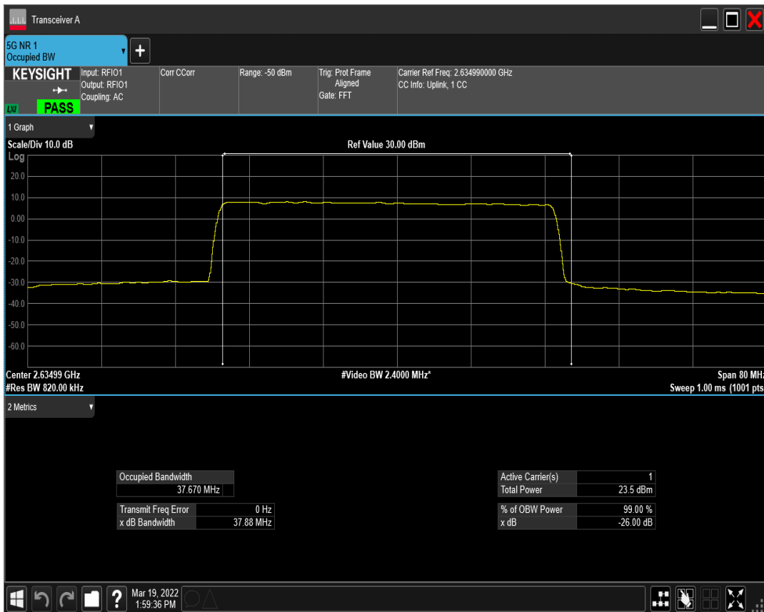
n41(2535-2655) SCS=30kHz DFT_QAM64 BW=40MHz Channel=526998 RB=100@0
