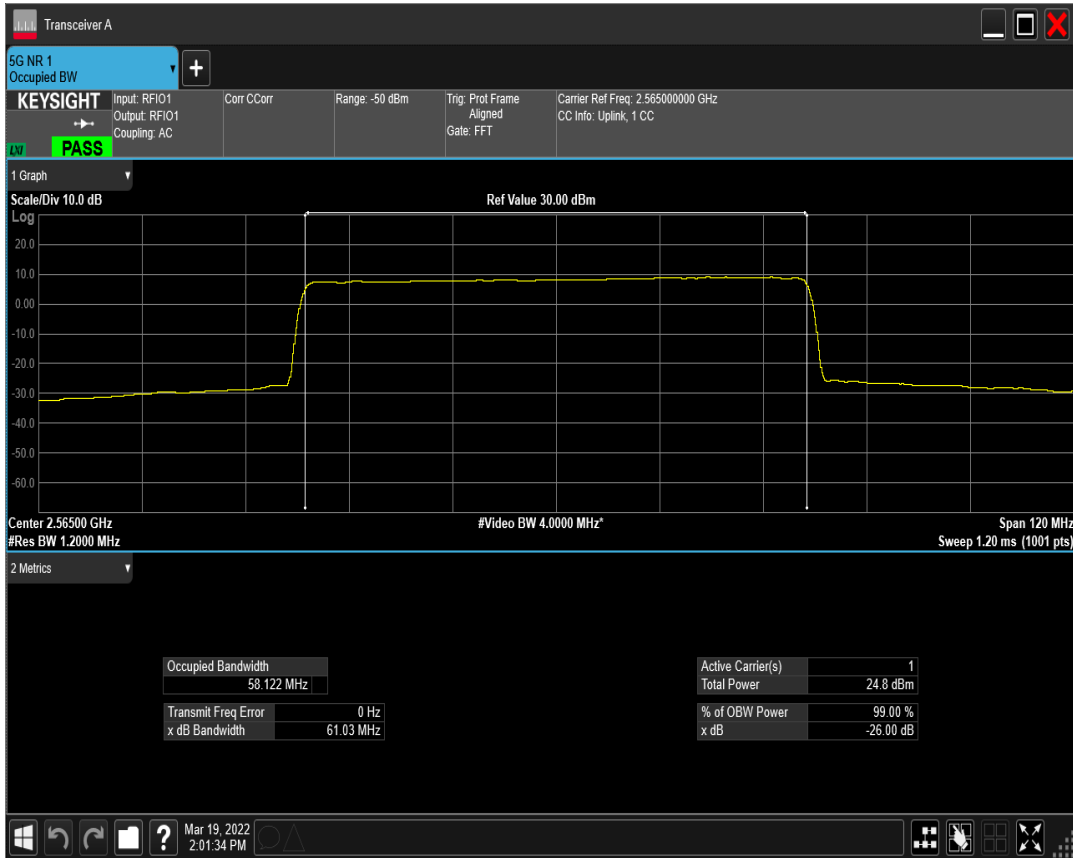
n41(2535-2655) SCS=30kHz DFT_QAM16 BW=60MHz Channel=513000 RB=162@0
