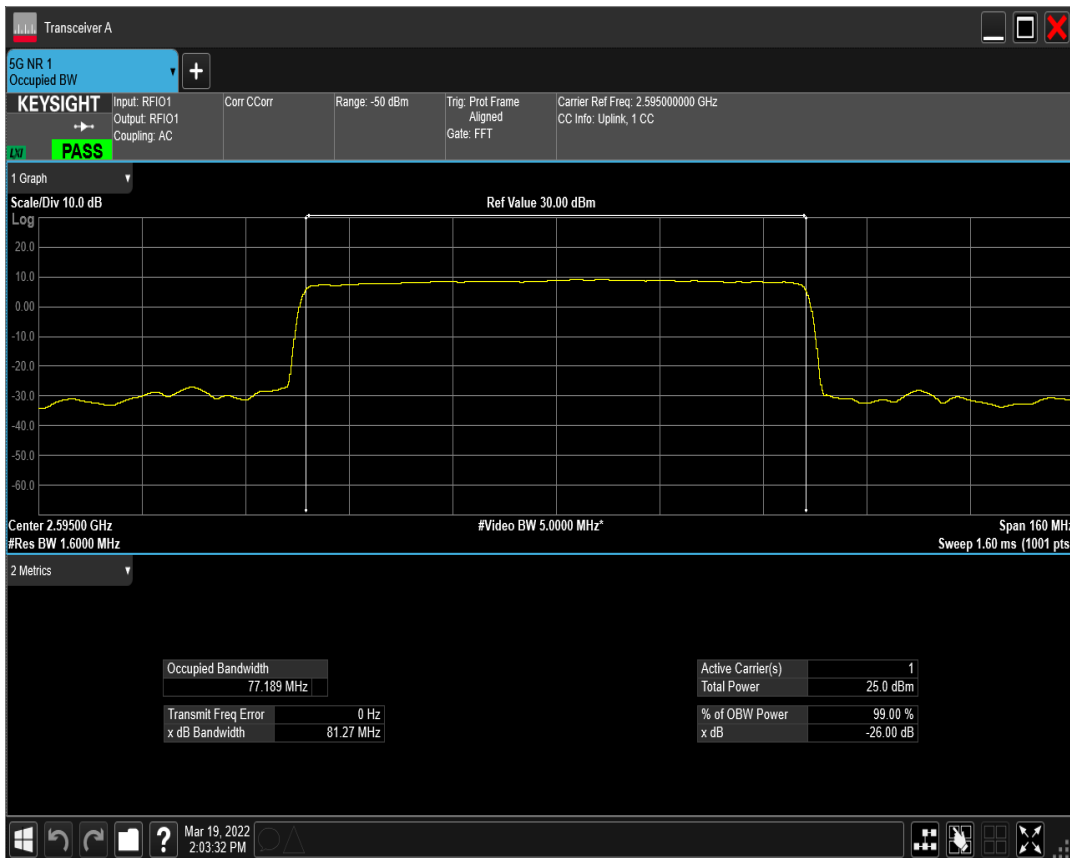
n41(2535-2655) SCS=30kHz DFT_QPSK BW=80MHz Channel=519000 RB=216@0
