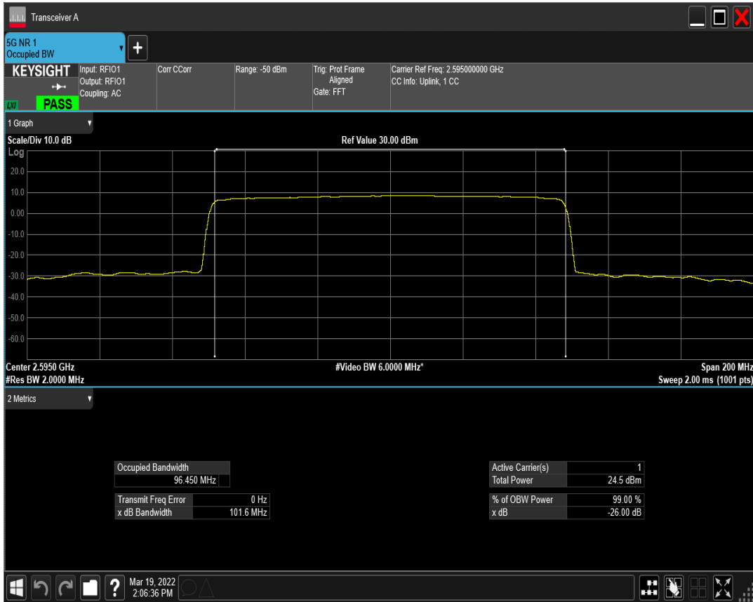
n41(2535-2655) SCS=30kHz DFT_QAM16 BW=100MHz Channel=519000 RB=270@0
