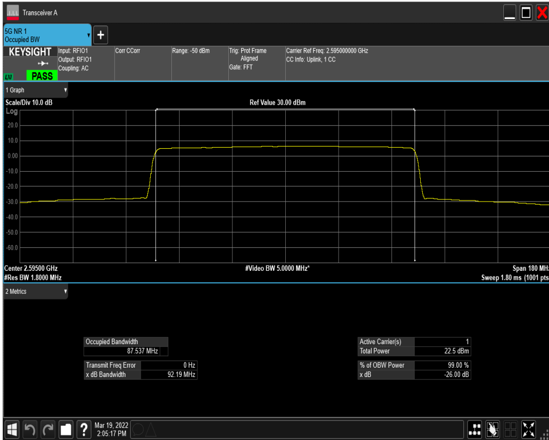
n41(2535-2655) SCS=30kHz DFT_BPSK BW=90MHz Channel=522000 RB=240@0
