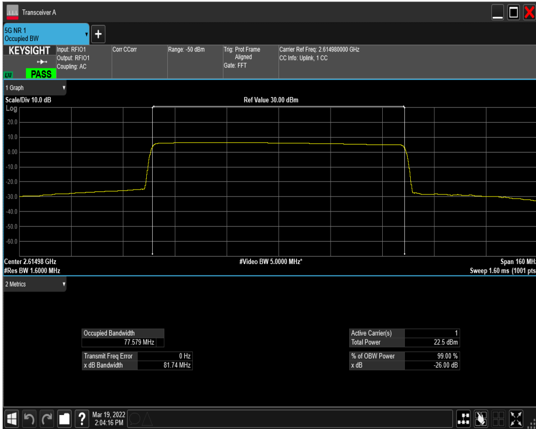
n41(2535-2655) SCS=30kHz DFT_BPSK BW=90MHz Channel=516000 RB=240@0
