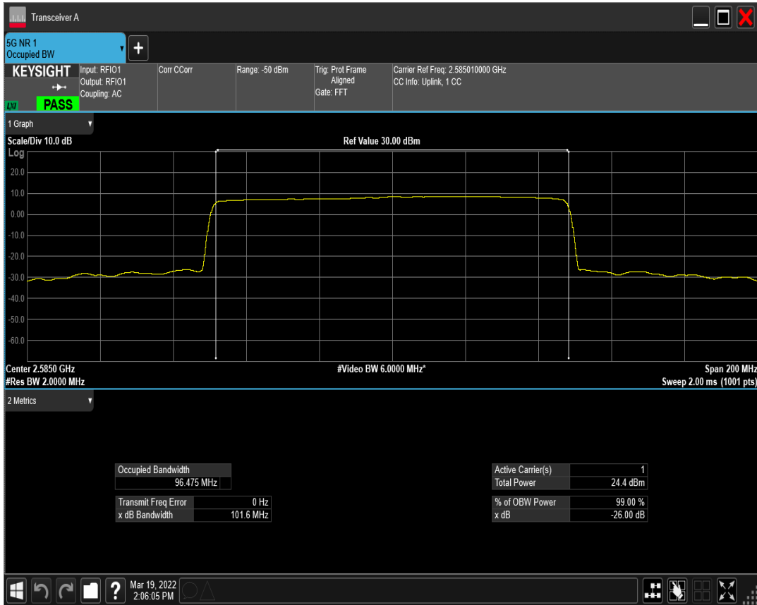
n41(2535-2655) SCS=30kHz DFT_QAM16 BW=100MHz Channel=517002 RB=270@0
