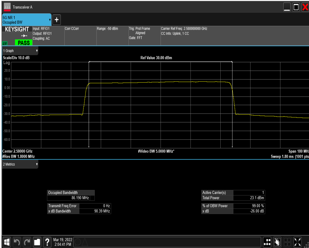
n41(2535-2655) SCS=30kHz DFT_QAM256 BW=90MHz Channel=516000 RB=240@0
