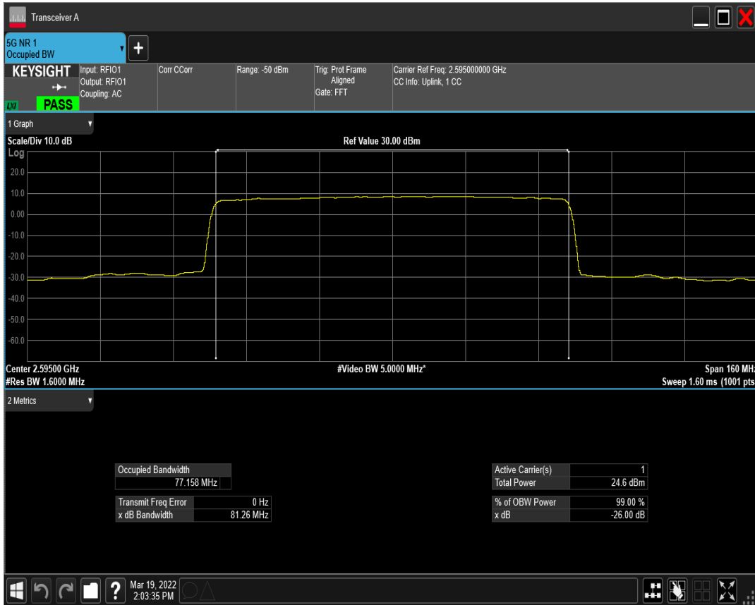
n41(2535-2655) SCS=30kHz DFT_QAM16 BW=80MHz Channel=519000 RB=216@0
