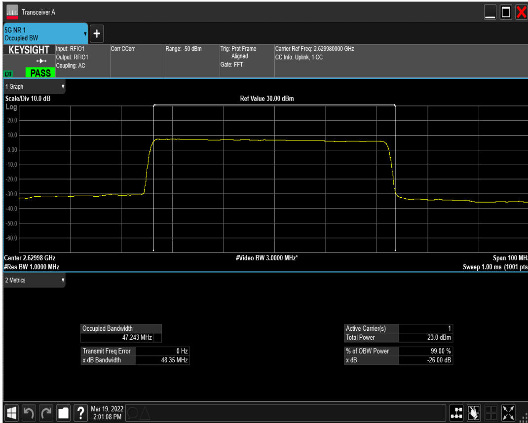
n41(2535-2655) SCS=30kHz DFT_QAM256 BW=50MHz Channel=525996 RB=128@0
