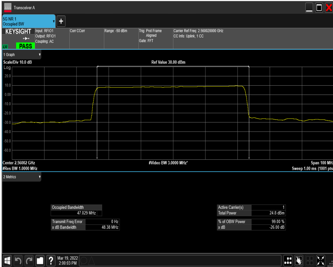
n41(2535-2655) SCS=30kHz DFT_QAM16 BW=50MHz Channel=512004 RB=128@0
