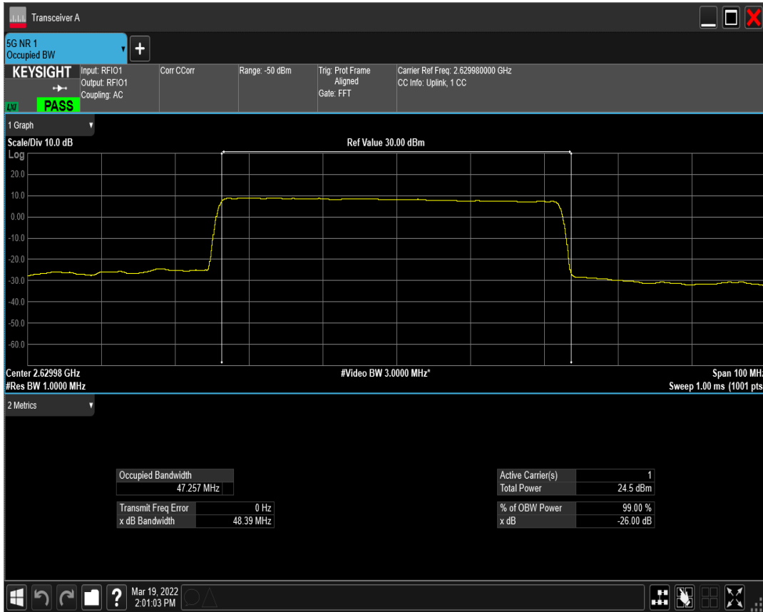
n41(2535-2655) SCS=30kHz DFT_QAM16 BW=50MHz Channel=525996 RB=128@0
