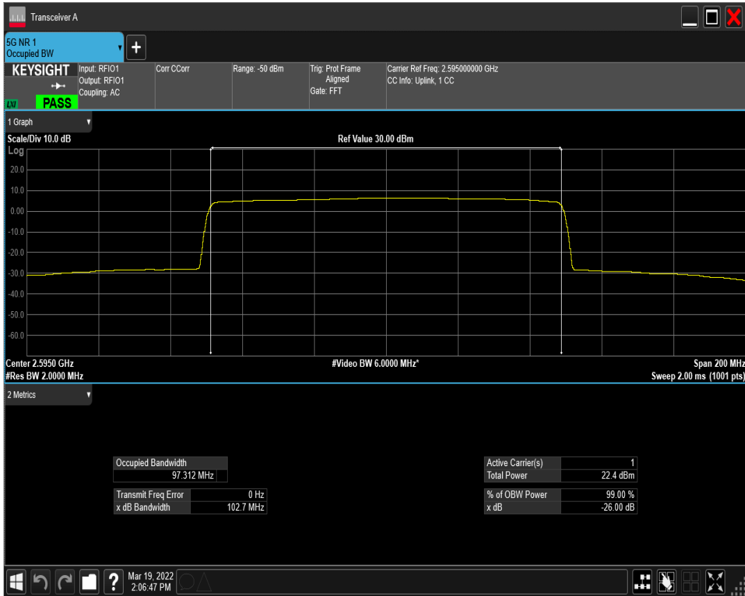
n41(2535-2655) SCS=30kHz DFT_BPSK BW=100MHz Channel=520998 RB=270@0
