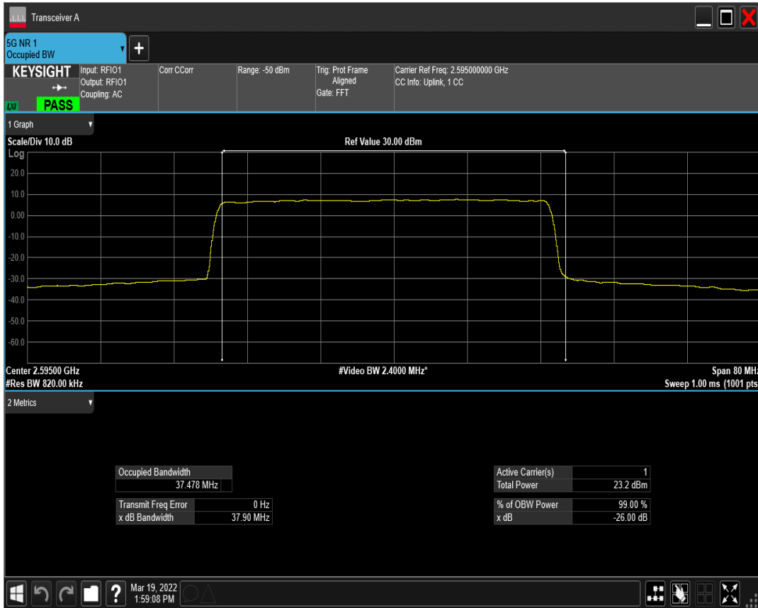
n41(2535-2655) SCS=30kHz DFT_QAM256 BW=40MHz Channel=519000 RB=100@0
