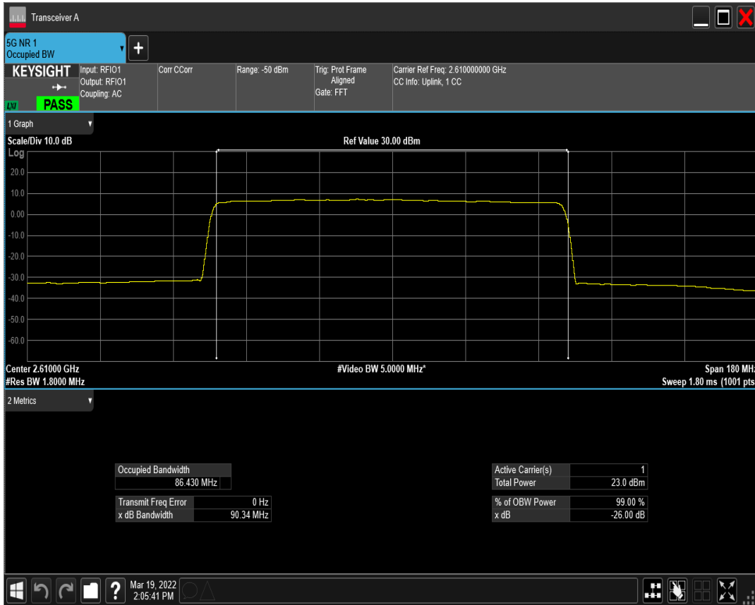
n41(2535-2655) SCS=30kHz DFT_QAM256 BW=90MHz Channel=522000 RB=240@0
