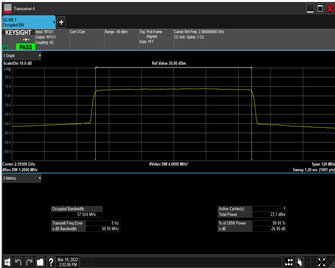
n41(2535-2655) SCS=30kHz DFT_QAM64 BW=60MHz Channel=519000 RB=162@0
