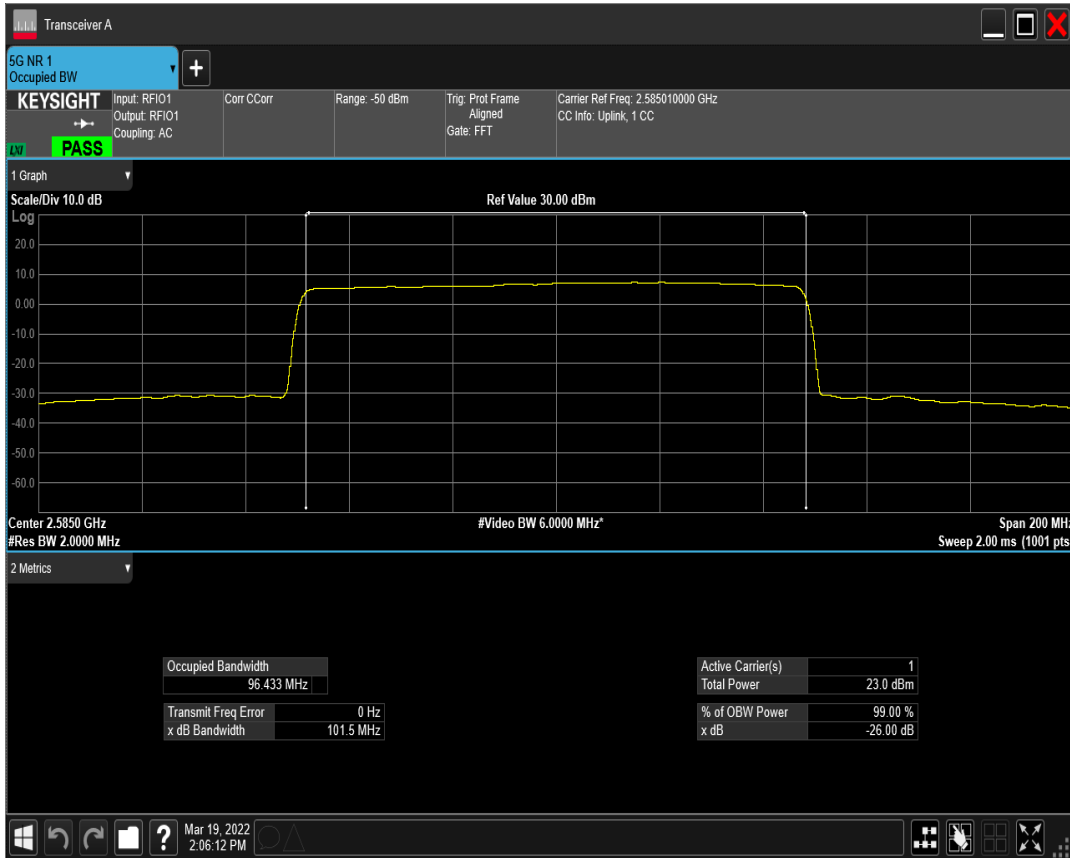
n41(2535-2655) SCS=30kHz DFT_QAM256 BW=100MHz Channel=517002 RB=270@0
