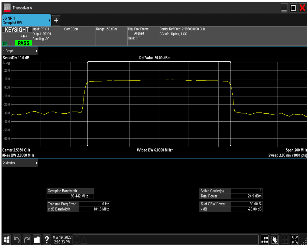
n41(2535-2655) SCS=30kHz DFT_QPSK BW=100MHz Channel=519000 RB=270@0
