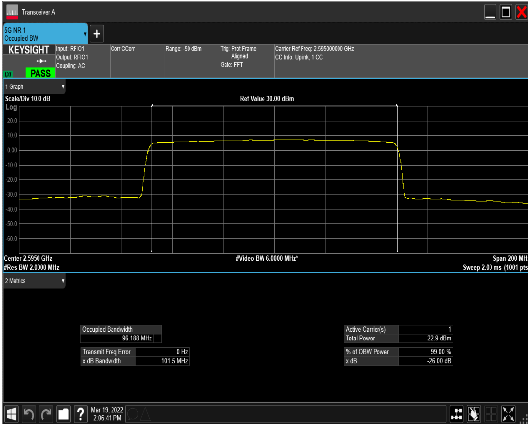
n41(2535-2655) SCS=30kHz DFT_QAM256 BW=100MHz Channel=519000 RB=270@0
