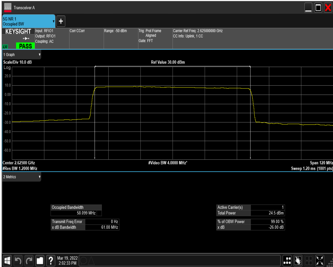
n41(2535-2655) SCS=30kHz DFT_QAM16 BW=60MHz Channel=525000 RB=162@0
