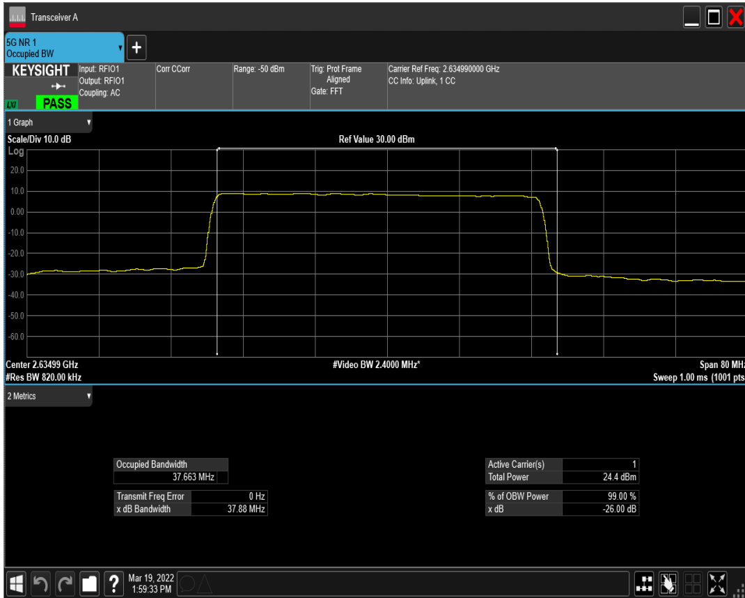
n41(2535-2655) SCS=30kHz DFT_QAM16 BW=40MHz Channel=526998 RB=100@0
