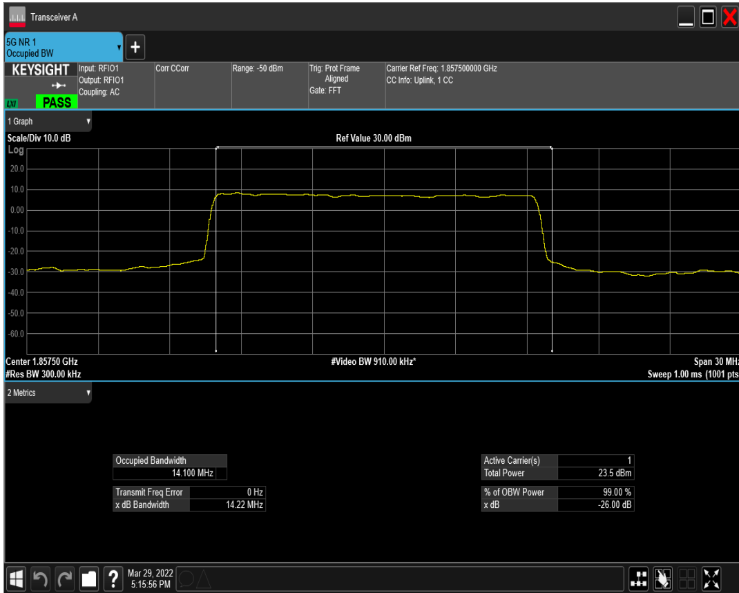
n2 SCS=15kHz DFT_QPSK BW=15MHz Channel=371500 RB=75@0
