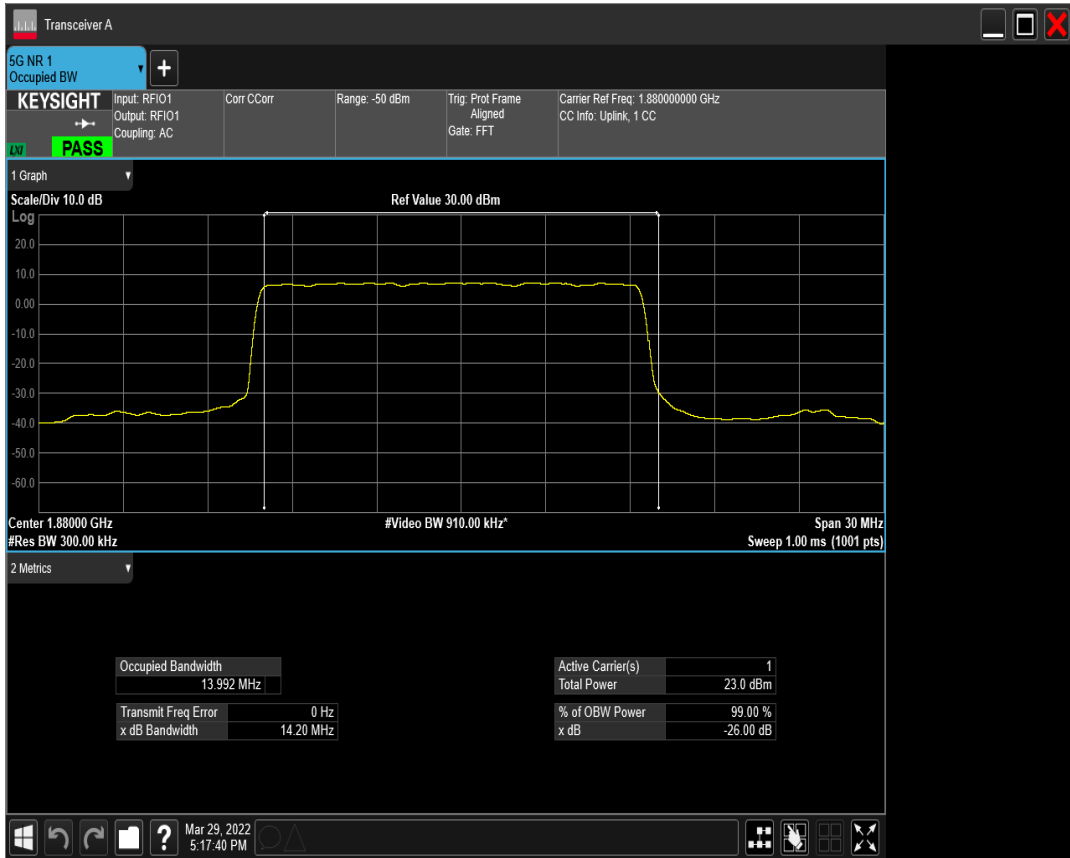
n2 SCS=15kHz DFT_QPSK BW=15MHz Channel=376000 RB=75@0
