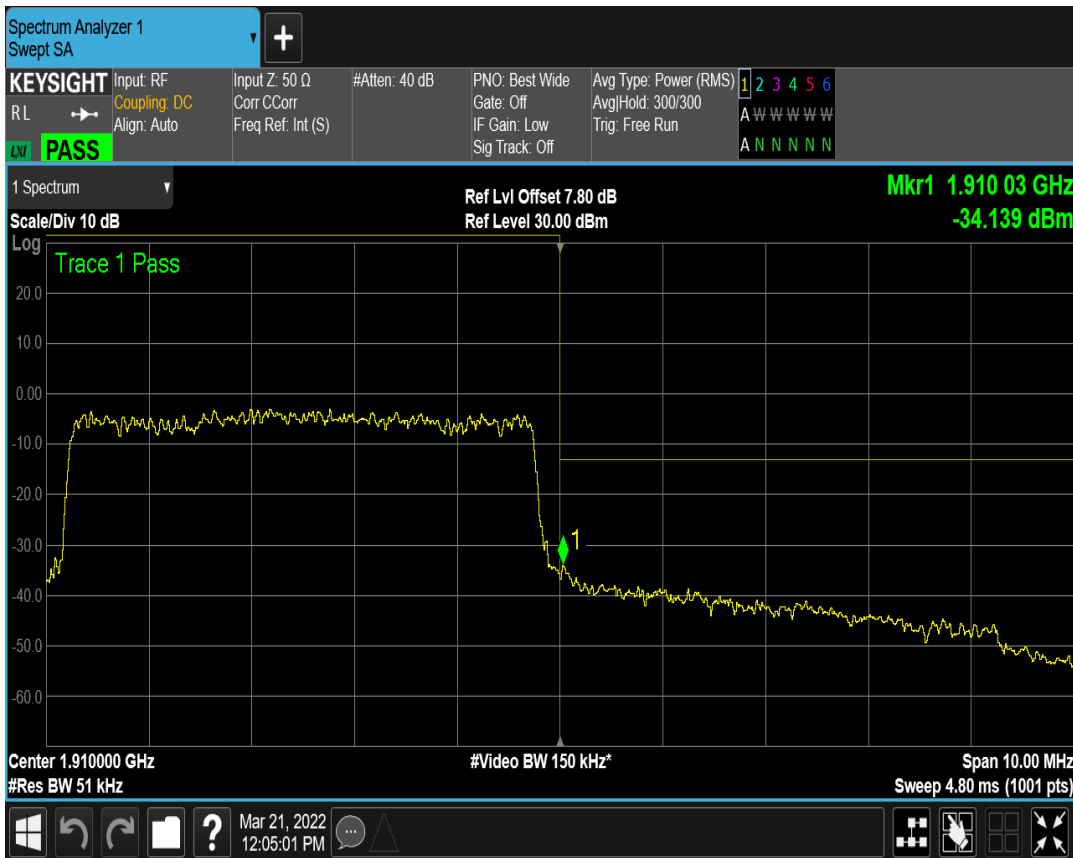
n2 SCS=15kHz DFT_QPSK BW=5MHz Channel=381500 RB=1@24
