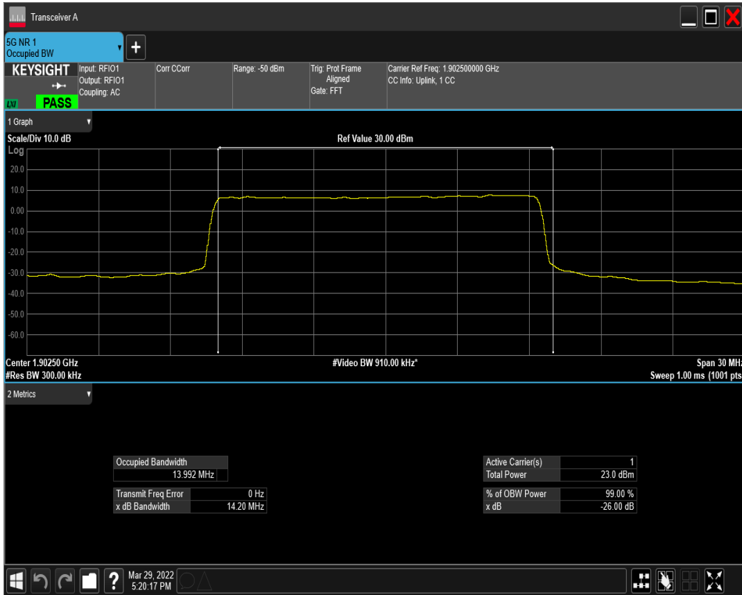
n2 SCS=15kHz DFT_QPSK BW=15MHz Channel=380500 RB=75@0
