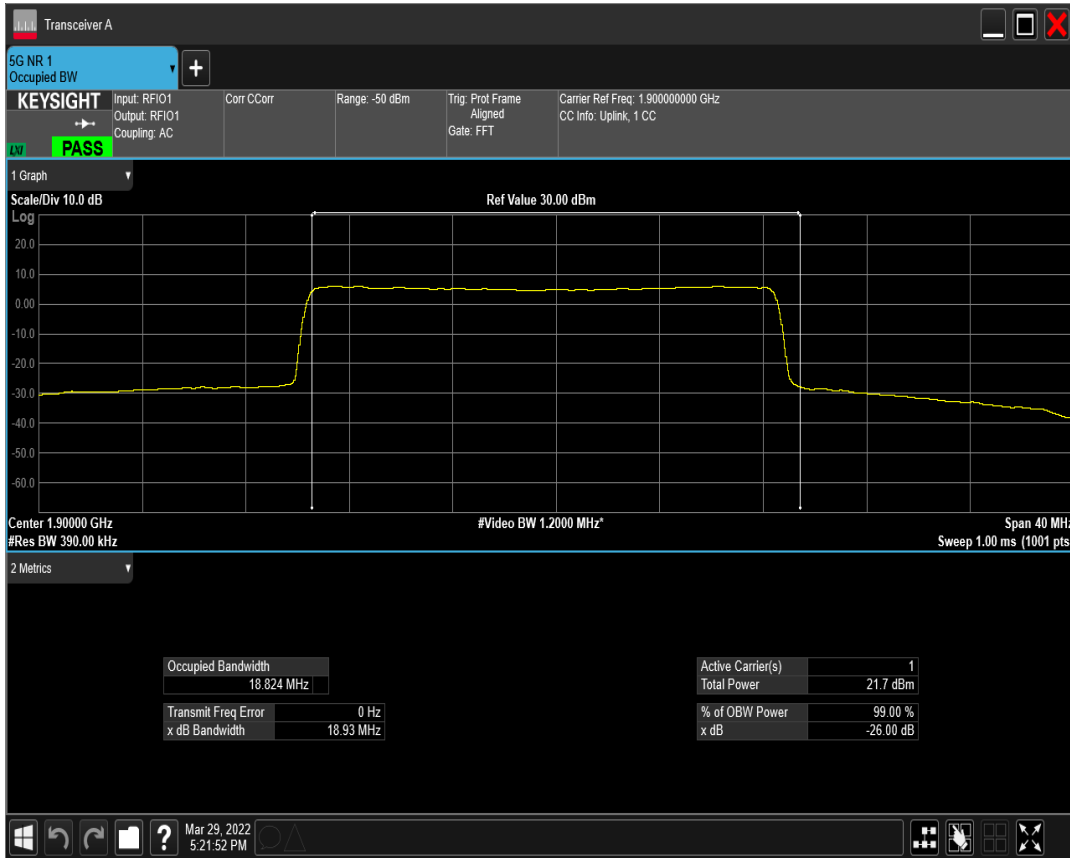
n2 SCS=15kHz DFT_QAM64 BW=20MHz Channel=380000 RB=100@0
