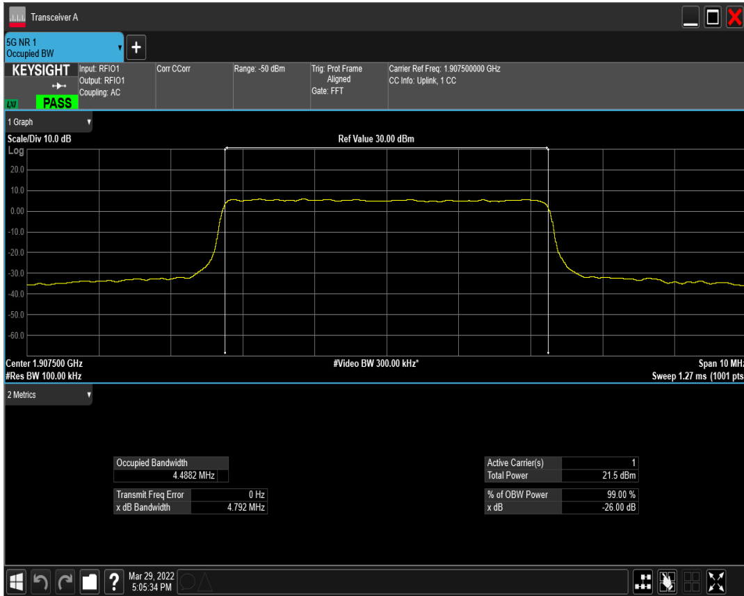
n2 SCS=15kHz DFT_QAM64 BW=5MHz Channel=381500 RB=25@0
