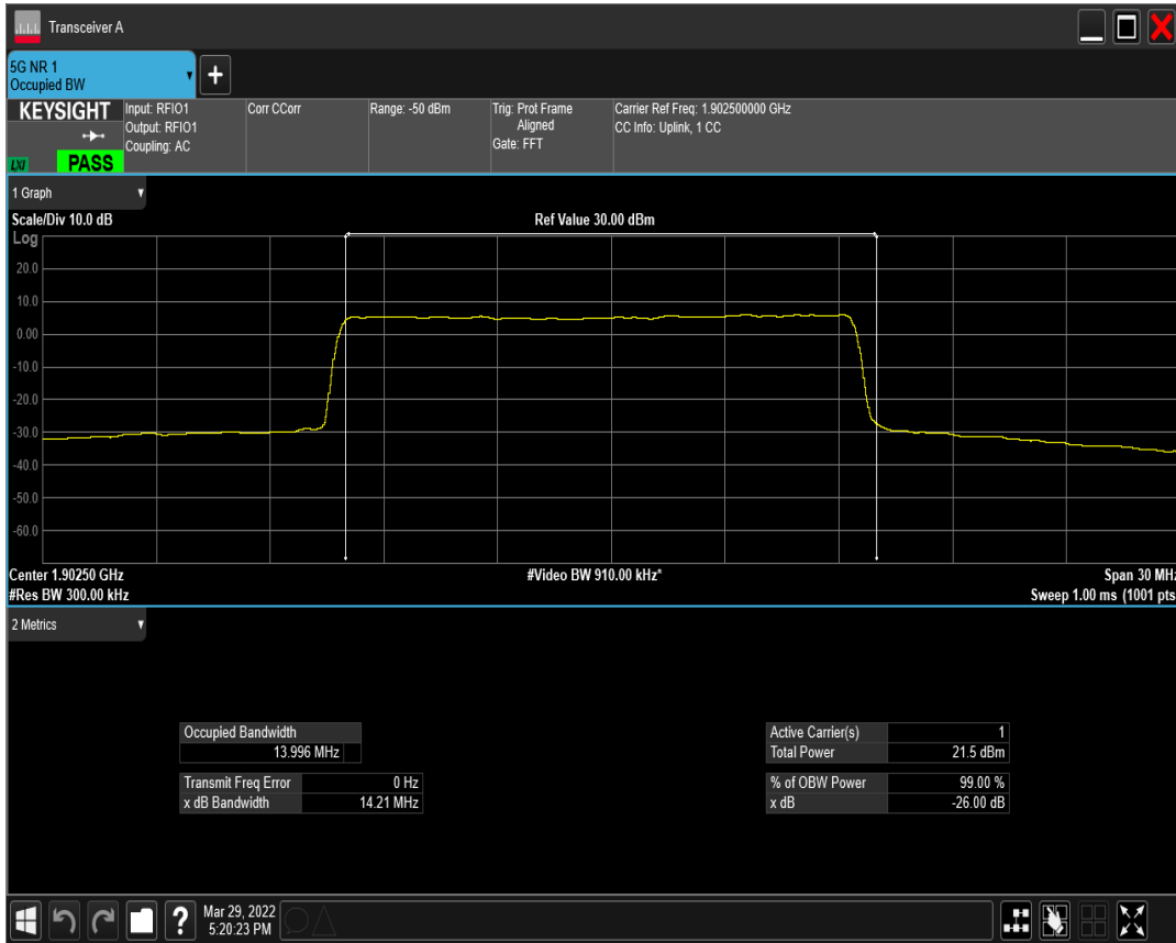
n2 SCS=15kHz DFT_QAM64 BW=15MHz Channel=380500 RB=75@0
