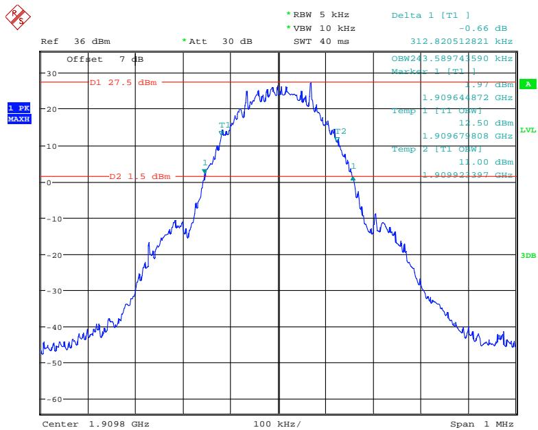
**26 dB Emissions & 99% Occupied Bandwidth for EGPRS (8PSK) Mode, Low channel**
