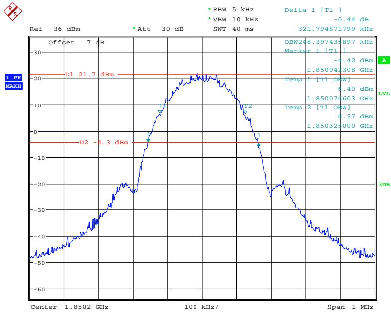
**26 dB Emissions &99% Occupied Bandwidth for EGPRS (8PSK) Mode, Middle channel**
