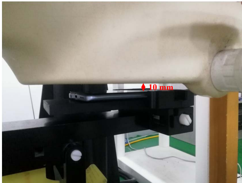
Body (Worn) Front Setup Photo (10mm)
