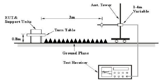
The radiated emission tests were performed in the 3 meters chamber test site, using the setup accordance with the ANSI C63.4-2014. The specification used was the FCC Part 15.109 limits.
