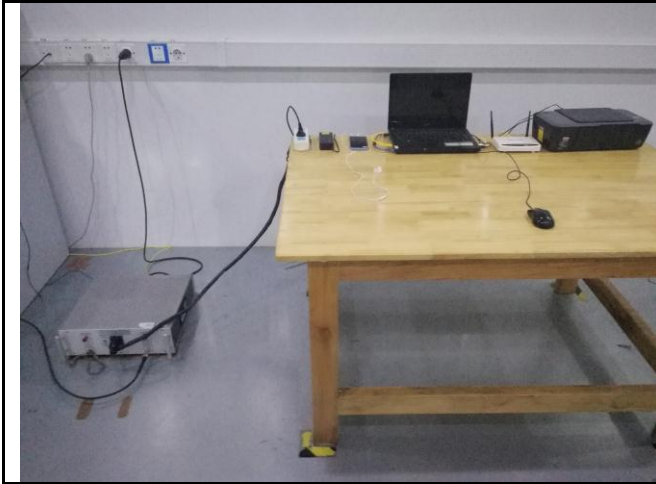
Conducted Emissions Test Setup – Front View
