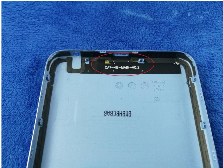
GSM/PCS/UMTS-FDD/LTE Antenna View
