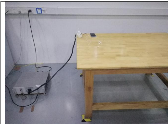
Conducted Emissions Test Setup Front View
