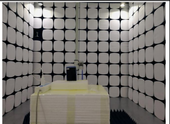
Radiated Spurious Emissions Test Setup Above 1GHz
