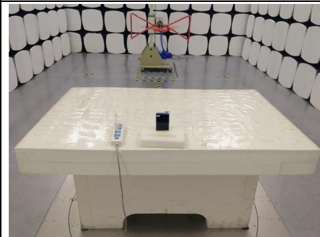
Conducted Emissions Test Setup Front View
