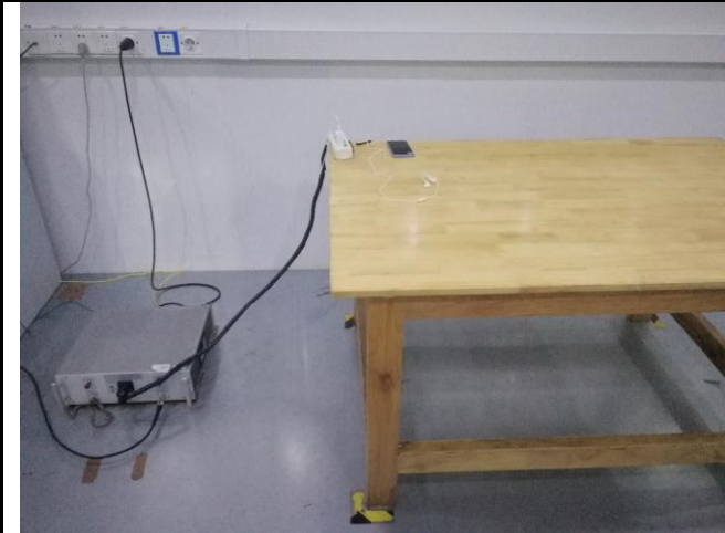
Conducted Emissions Test Setup Front View
