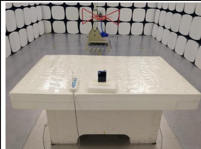
Conducted Emissions Test Setup Front View
