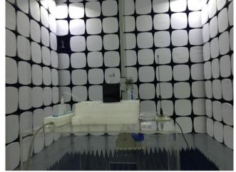
Radiated Spurious Emissions Test Setup Above 1GHz
