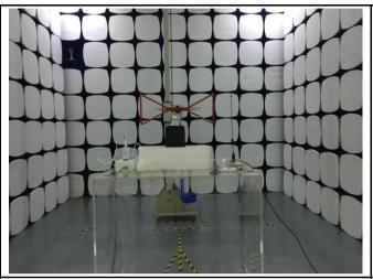
Radiated Spurious Emissions Test Setup Below 1GHz
