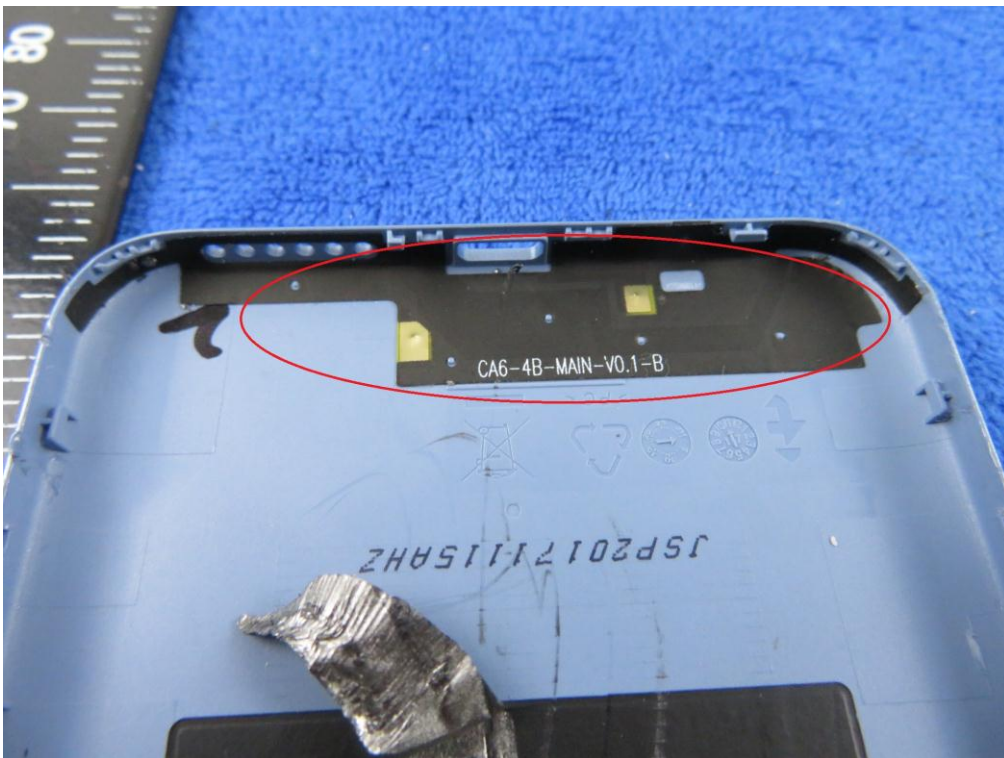
GSM/PCS/UMTS-FDD/LTE Antenna View
