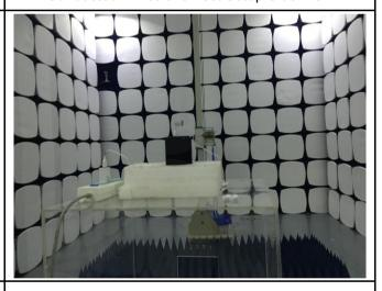
Radiated Spurious Emissions Test Setup Above 1GHz
