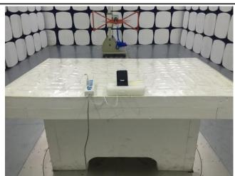
Radiated Spurious Emissions Test Setup Below 1GHz
