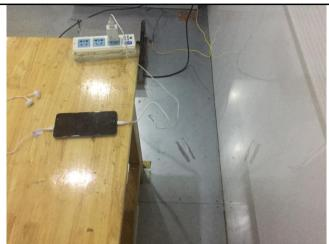
Conducted Emissions Test Setup Side View
