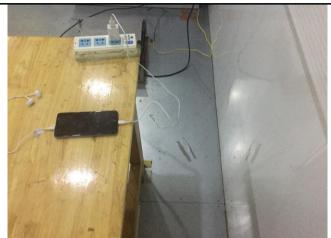
Conducted Emissions Test Setup Side View
