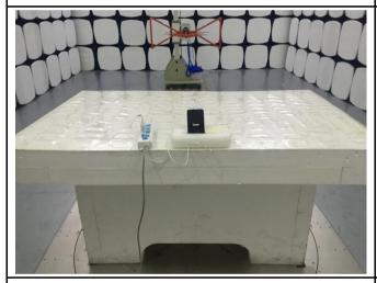
Radiated Spurious Emissions Test Setup Below 1GHz
