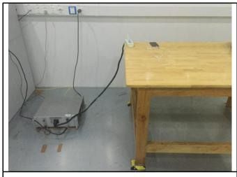
Conducted Emissions Test Setup Front View
