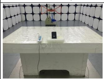
Radiated Spurious Emissions Test Setup Below 1GHz
