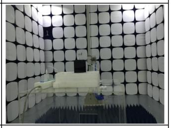
Radiated Spurious Emissions Test Setup Above 1GHz
