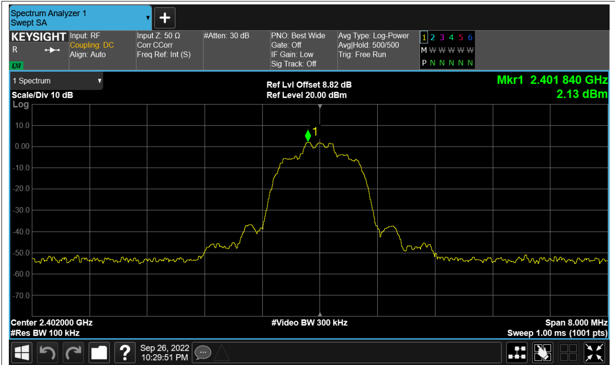
Band Edge NVNT 3-DH1 2402MHz Ant1 No-Hopping Emission
