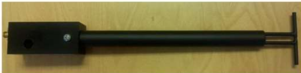
Figure 1 – MVG COMOSAR Validation Dipole
