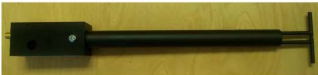
Figure 1 – MVG COMOSAR Validation Dipole
