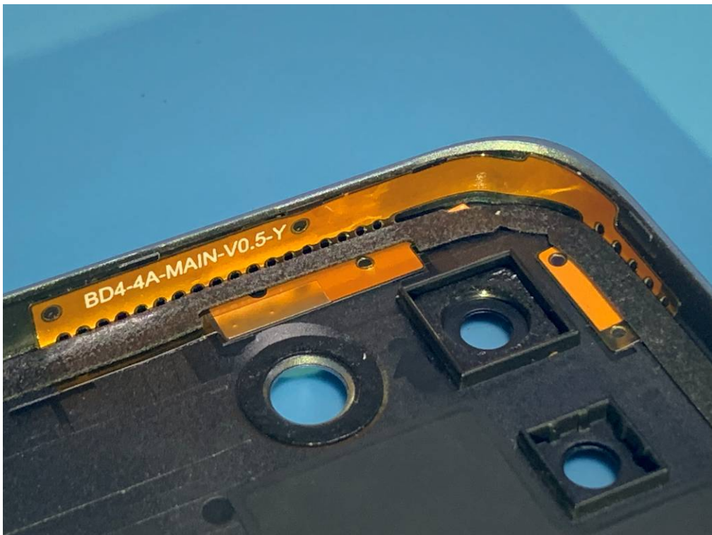
GSM & WCDMA & LTE Main Antenna
