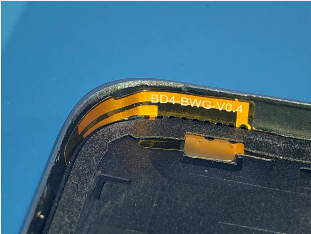
GSM & WCDMA & LTE Main Antenna
