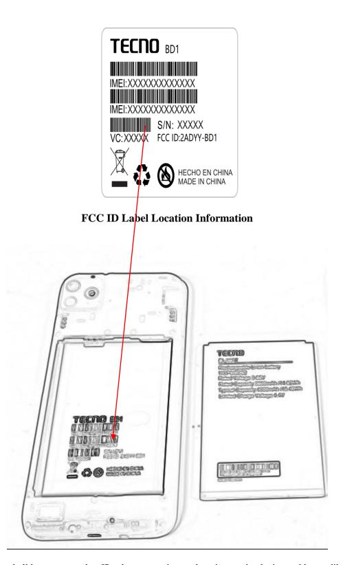
The label shown shall be permanently affixed at a conspicuous location on the device and be readily visible to the user at the time purchase (Labeling requirements per 2.925)
