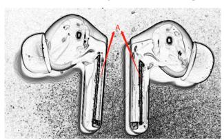
B. Top cover (B): The top cover does not provide enough physical space to fit the printing of the FCC certification No. according to below reference picture.
