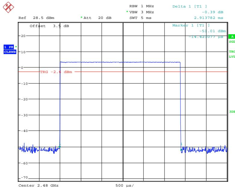
**EDR ( $\pi/4$ -DQPSK):****Pulse time, Low Channel, 2DH1**
