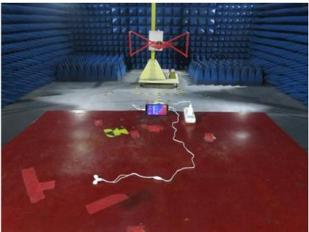
RADIATED EMISSION TEST (Frequency above 1GHz)
