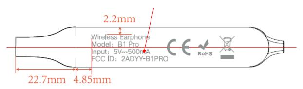
The label shown shall be permanently affixed at a conspicuous location on the device and be readily visible to the user at the time purchase (Labeling requirements per 2.925)
